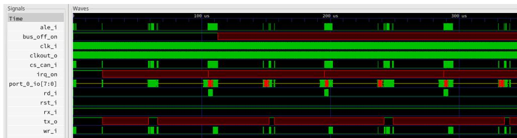
Figure 2.6. Post-Synthesis Standalone Controller Waveforms
