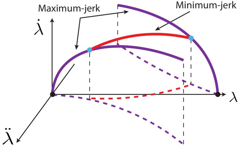
Figure 2.9 – Three-dimensional phase space with jerk limits [44]
