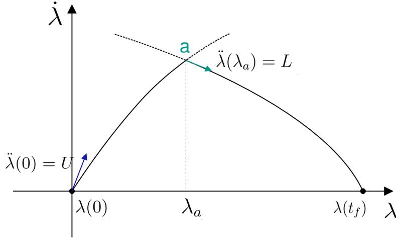
**Figure 2.13** – Optimal trajectory with single switching point
