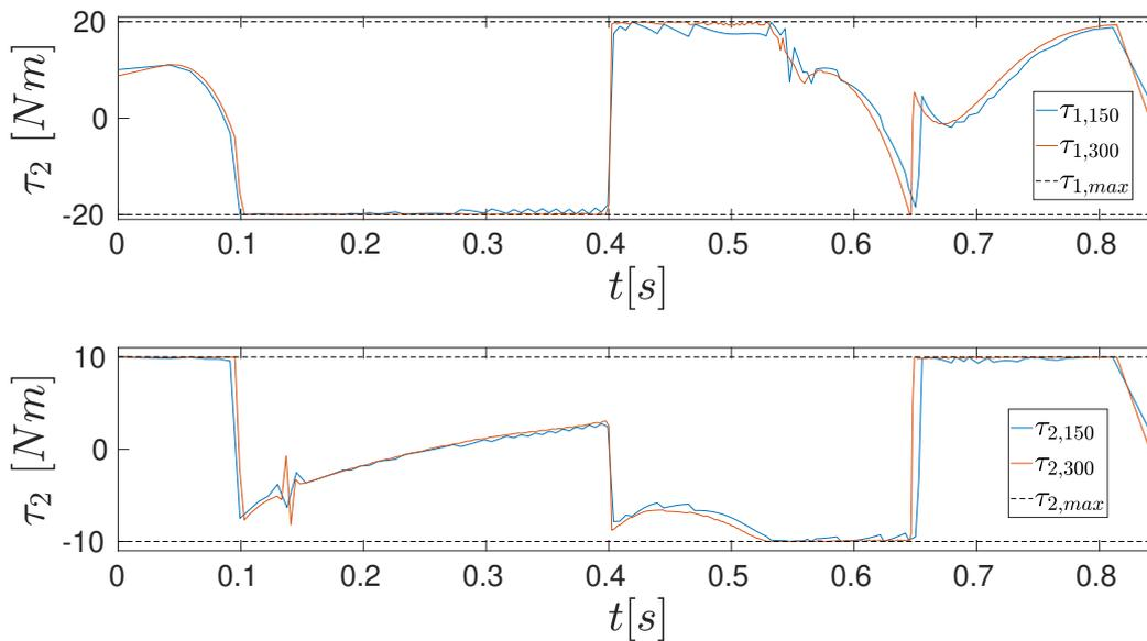
**Figure 5.9** – Third simulation. The comparison between planned torques in 1<sup>st</sup> simulation with low grid resolution (blue) and 2<sup>nd</sup> simulation with high grid resolution (red).
