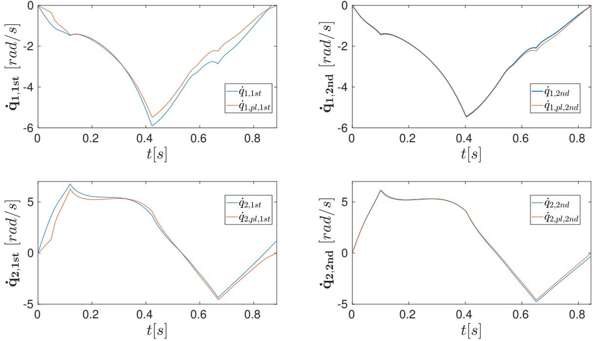
**Figure 5.7** – Second simulation: The comparison between simulated joints' velocities (blue), and ideal ones (red) obtained from planning. On the left, the results from 1<sup>st</sup> formulation, on the right from 2<sup>nd</sup> formulation.
