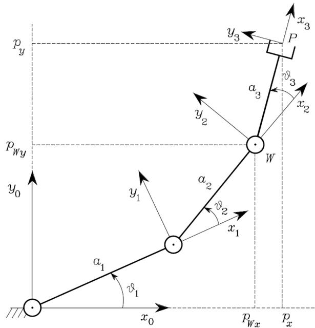
**Figure 2.2** – Joint and task space in a three-links manipulator [49]
