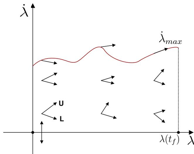
**Figure 2.8** – Representation of *pseudo-acceleration* limits as arrows in phase plane plot
