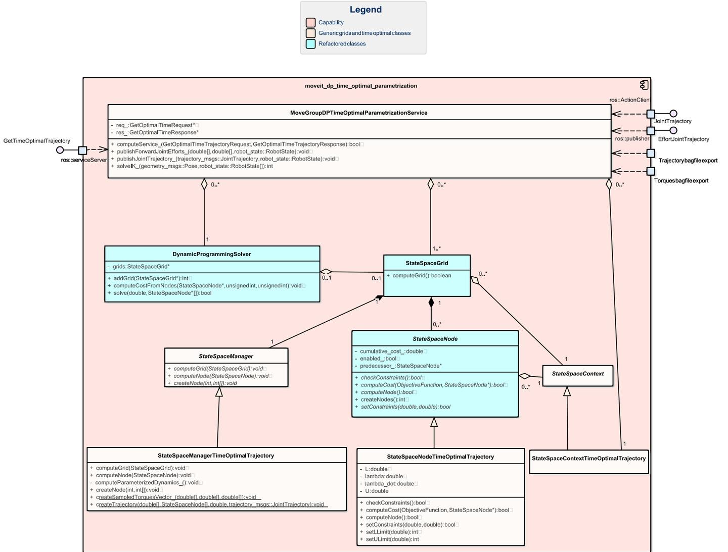
**Figure 4.5** – UML decomposition/class diagram representing the classes which compose the time optimal trajectory generation module.
