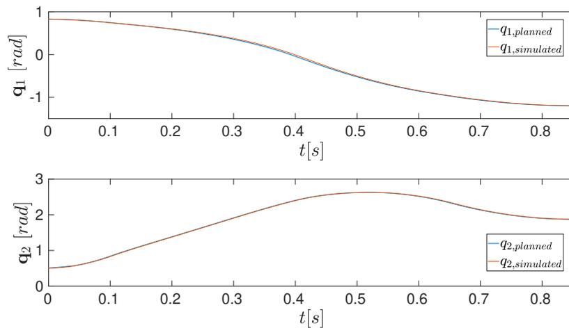
**Figure 5.13** – Fourth simulation. The comparison between simulated (red) joints' positions and planned ones (blue).
