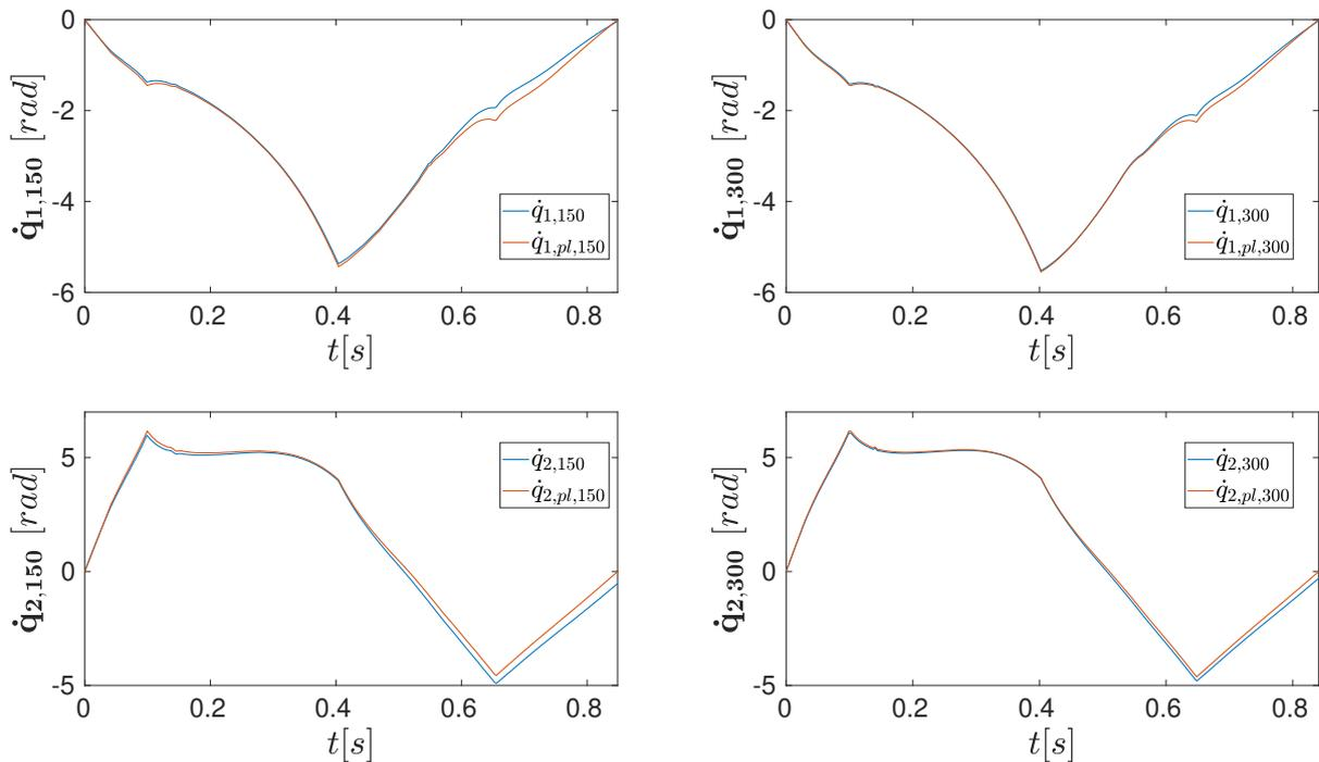
**Figure 5.11** – Third simulation. The comparison between simulated joints’ velocities (blue) and ideal ones (red) obtained from planning. On the left, the results from 1<sup>st</sup> simulation with low grid resolution, on the right from 2<sup>nd</sup> simulation with high grid resolution.
