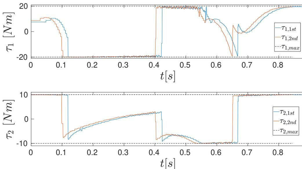
**Figure 5.5** – Second simulation: The comparison between planned torques in 1<sup>st</sup> formulation (blue) and 2<sup>nd</sup> formulation (red).
