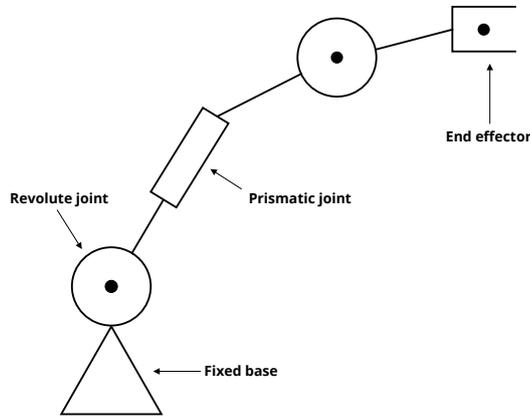
**Figure 2.1** – Kinematic chain
