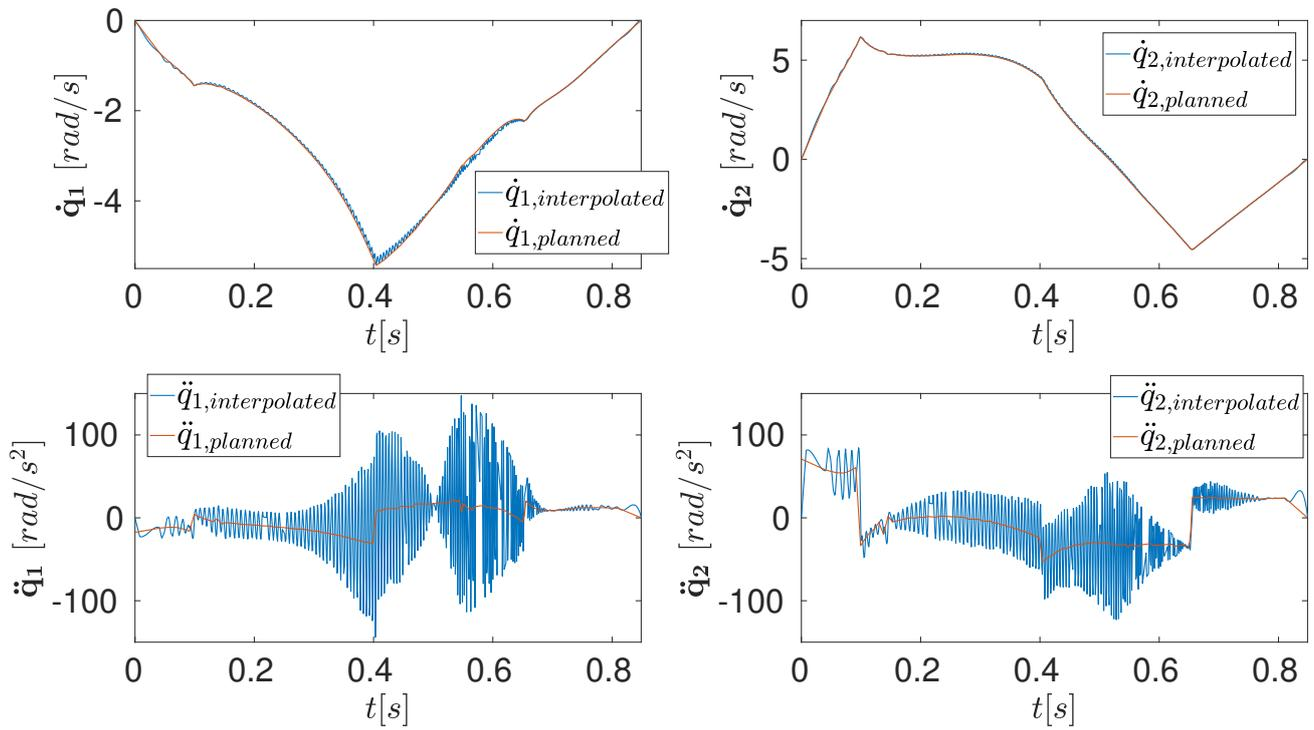
**Figure 5.12** – Fourth simulation. The comparison between planned (red) and interpolated (blue) joints' velocities and accelerations.
