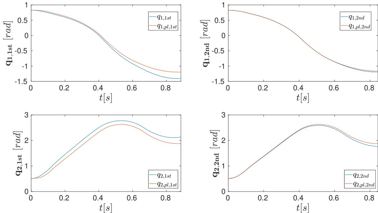
**Figure 5.6** – Second simulation. The comparison between simulated joints’ position (blue) and ideal ones (red), obtained from planning. On the left, the results from 1<sup>st</sup> formulation, on the right from 2<sup>nd</sup> formulation.
