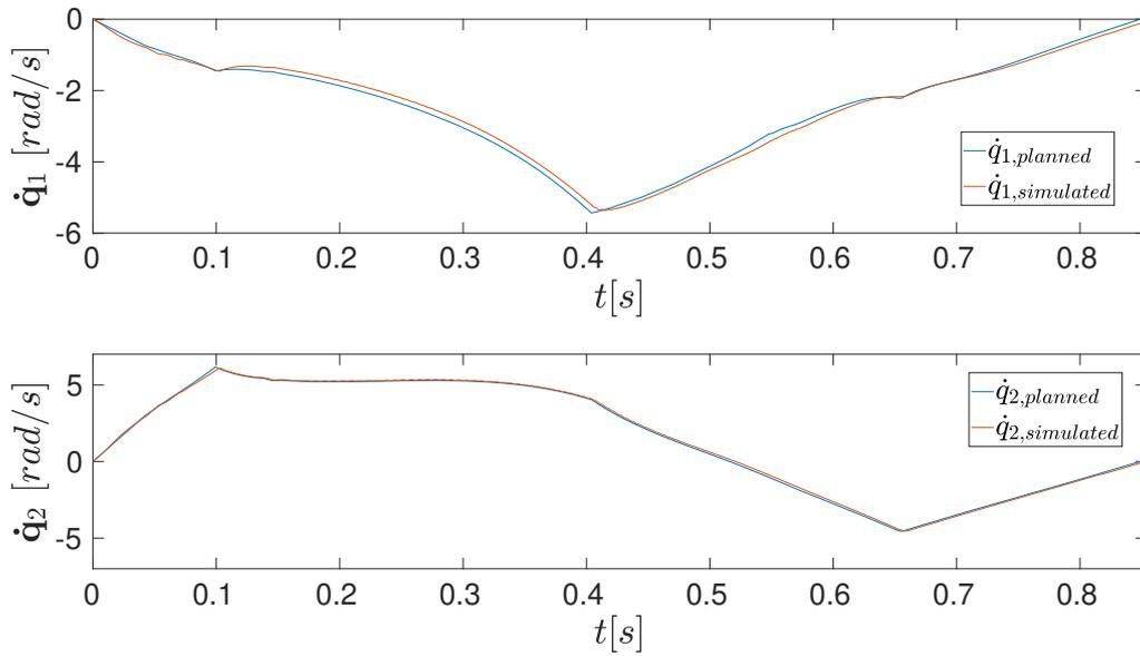
**Figure 5.14** – Fourth simulation. The comparison between simulated (red) joints' velocities and planned ones (blue).
