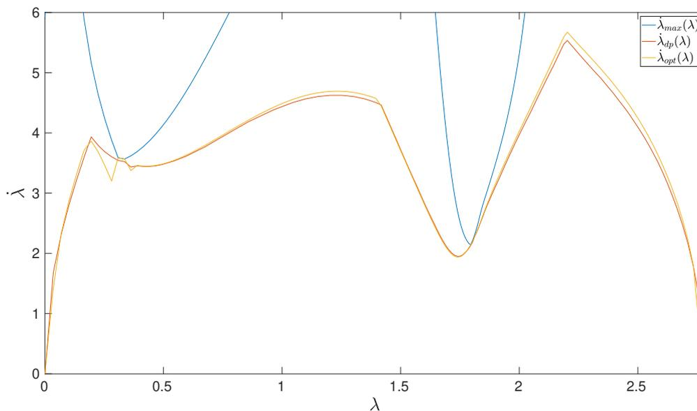
**Figure 5.2** – First simulation. The optimal trajectories in phase plane: in red the trajectory obtained through dynamic programming, in yellow the trajectory obtained through switching points method and in blue the MVC.
