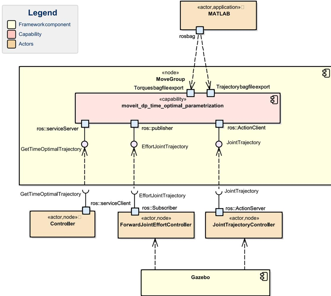
**Figure 4.4** – UML component diagram representing the connections between the capability and the other components. The link with Gazebo is better explained in Fig. 4.3.
