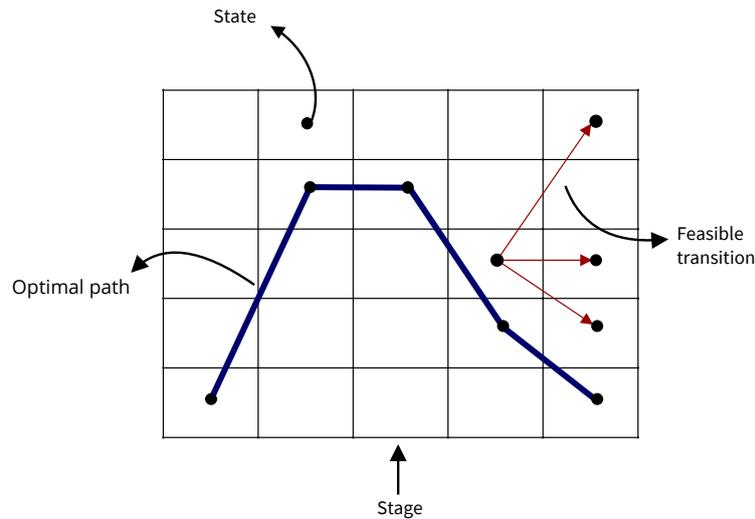
**Figure 3.3** – Example of a grid explored by dynamic programming
