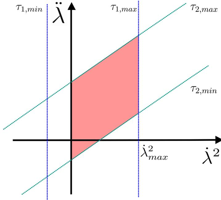
**Figure 2.11** – Polygon of feasible *pseudo-acceleration* in the  $\dot{\lambda}^2 - \ddot{\lambda}$  plane with a critical point
