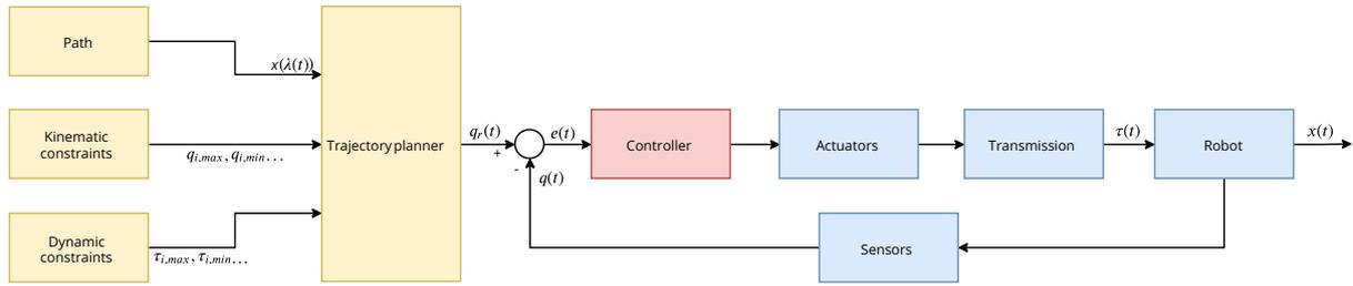
Figure 2.3 – General control scheme for trajectory planning
