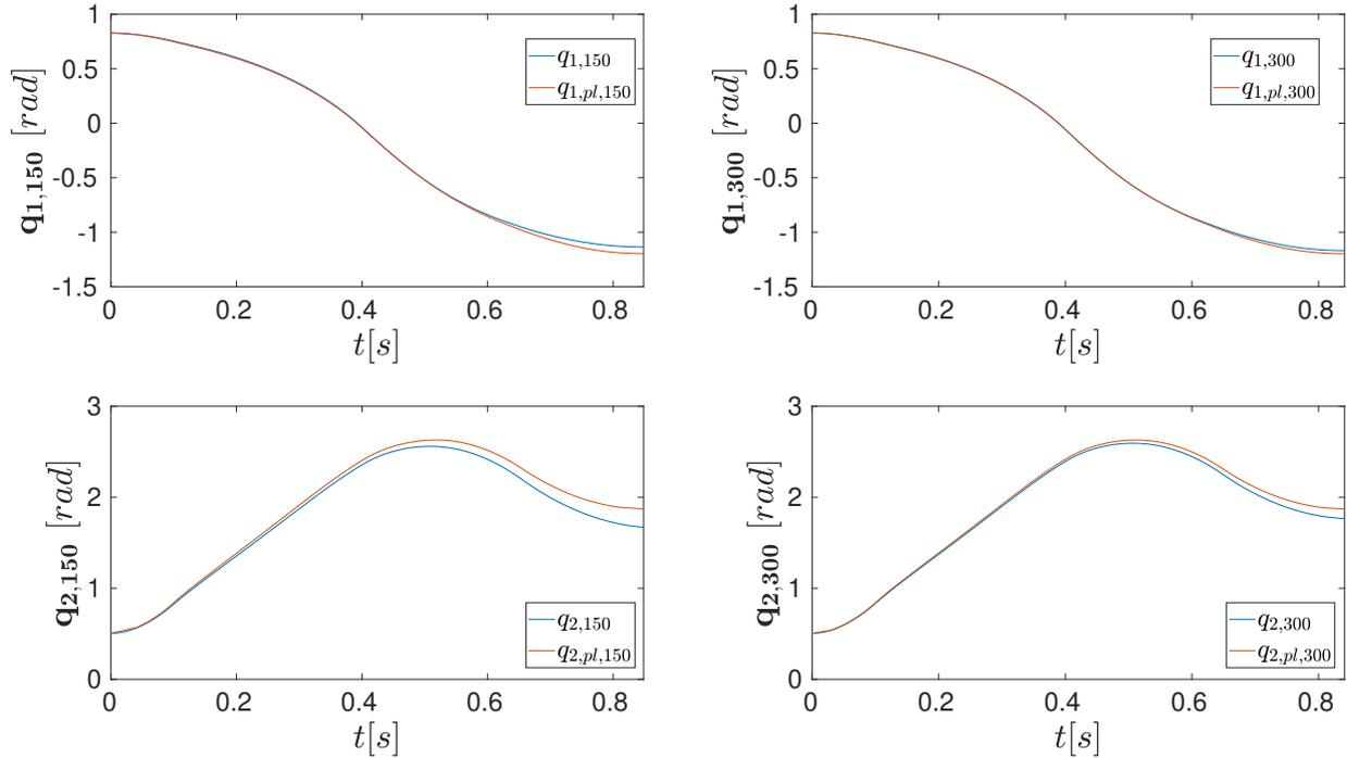
**Figure 5.10** – Third simulation. The comparison between simulated joints' positions (blue) and ideal ones (red) obtained from planning. On the left, the results from 1<sup>st</sup> simulation with low grid resolution, on the right from 2<sup>nd</sup> simulation with high grid resolution.
