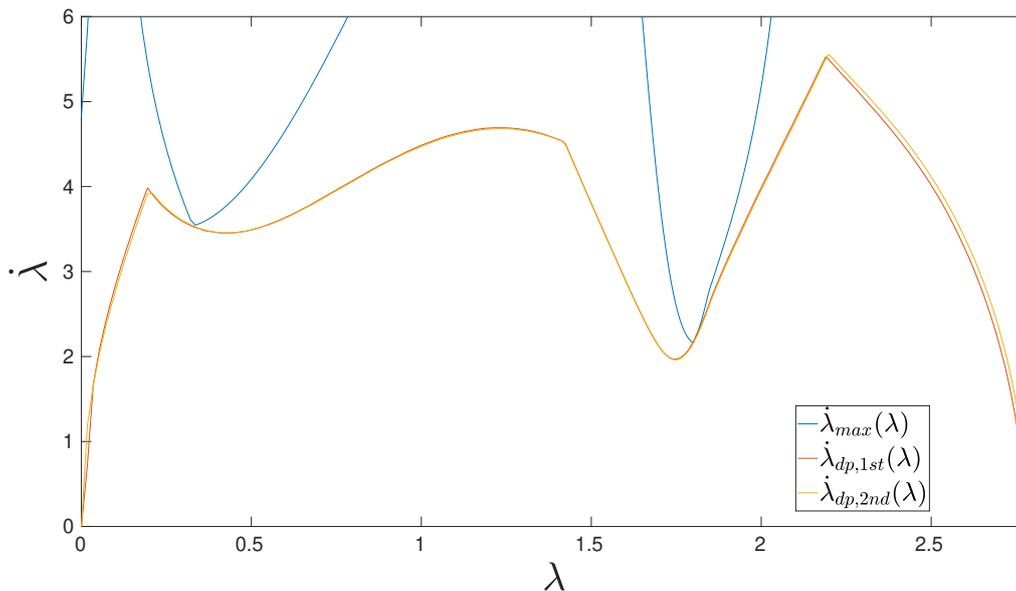
**Figure 5.4** – Second simulation. The optimal trajectories in phase plane: in red the trajectory obtained through dynamic programming with 1st formulation, in yellow the trajectory with 2nd formulation and in blue the MVC, corresponding to  $N_i = 300$ .
