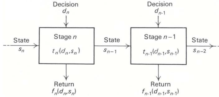
**Figure 3.2** – Stage transition process [21]
