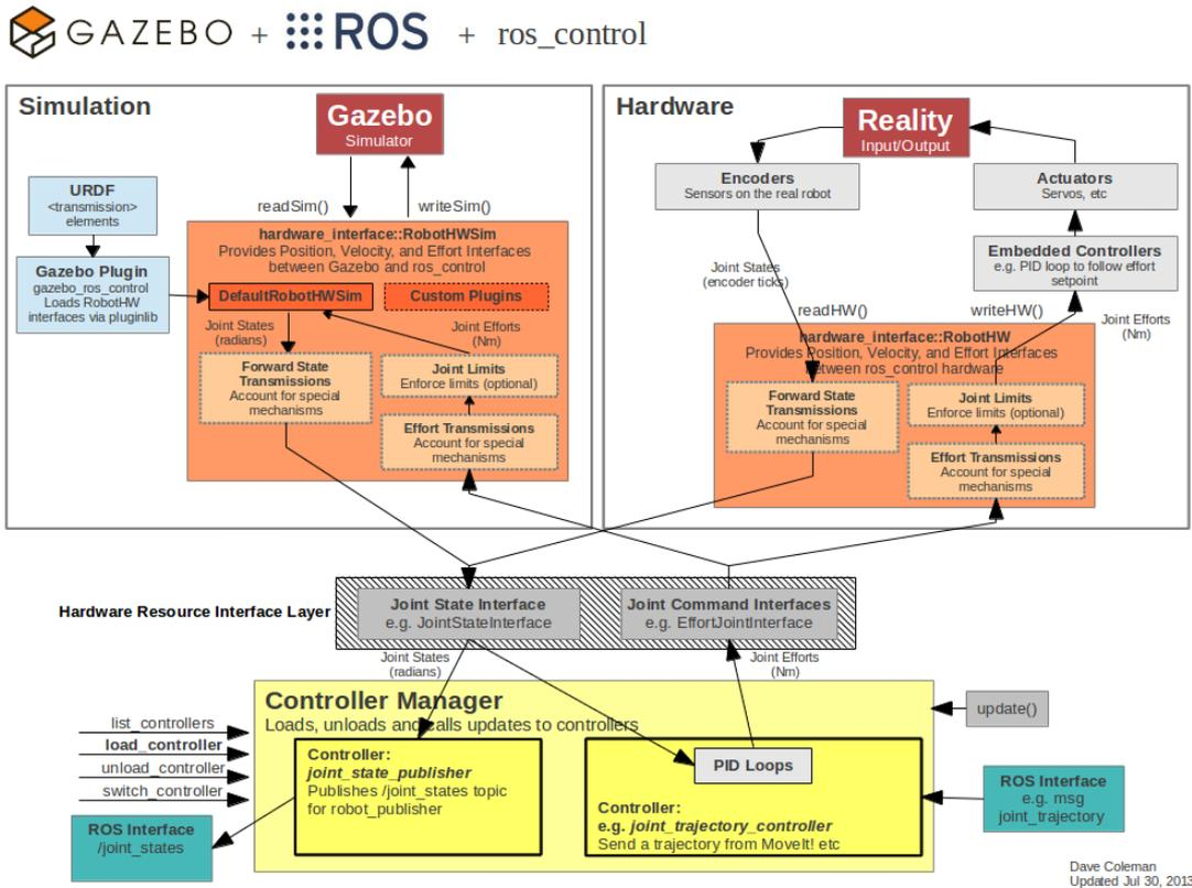
Figure 4.3 – Scheme representing the architecture overview on the simulated robot in Gazebo, the real robot and the controllers in ROS [2]
