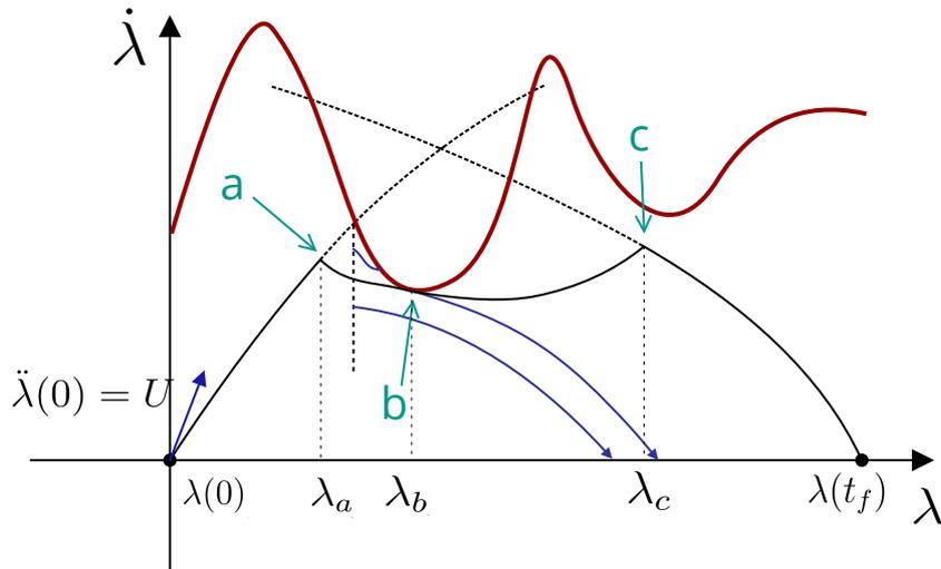
**Figure 2.14** – Resolution with multiple switching points: a, b and c are the three switching points, the red curve is the MVC and the blue curves are those obtained through integration during the *trial and error* phase.
