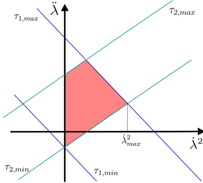
**Figure 2.10** – Polygon of feasible *pseudo-acceleration* in the  $\dot{\lambda}^2 - \ddot{\lambda}$  plane
