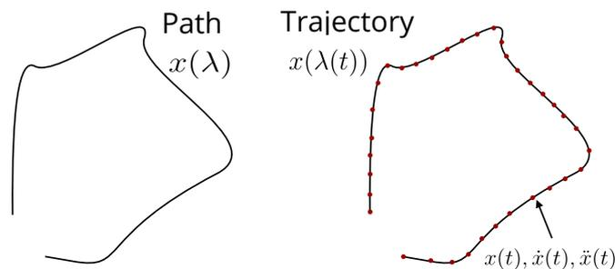
Figure 2.4 – Path and trajectory representation
