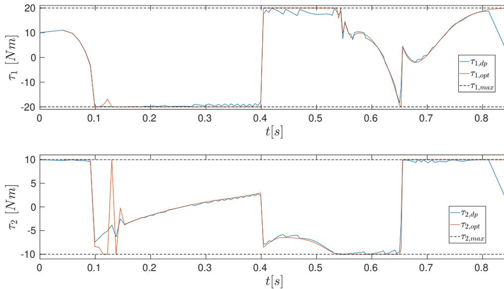
**Figure 5.3** – First simulation. Comparison between planned torques obtained through dynamic programming (blue) and switching points method (red).
