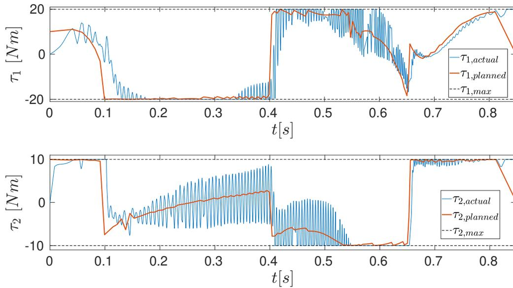
**Figure 5.15** – Fourth simulation. The comparison between planned torques (red) and the applied one (blue).
