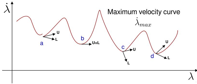
**Figure 2.12** – Representation of discontinuous (*a*), tangent(*b*) and singular point (*c,d*) on the MVC
