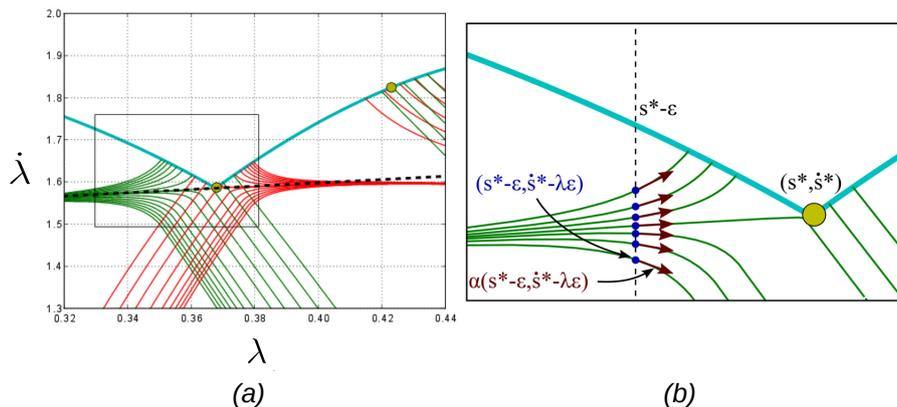
**Figure 2.15** – (a) fields of the *pseudo-acceleration* L (green curves) and U (red curves) in the neighbourhood of the switching points; (b) zoom of the black box of (a) [45]
