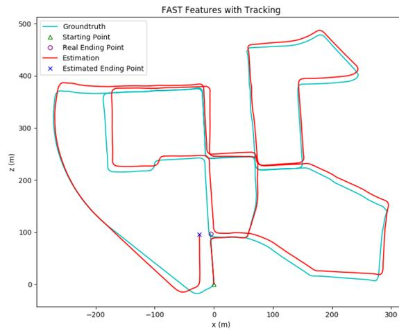
Figure 4.5: FAST features with Tracking
