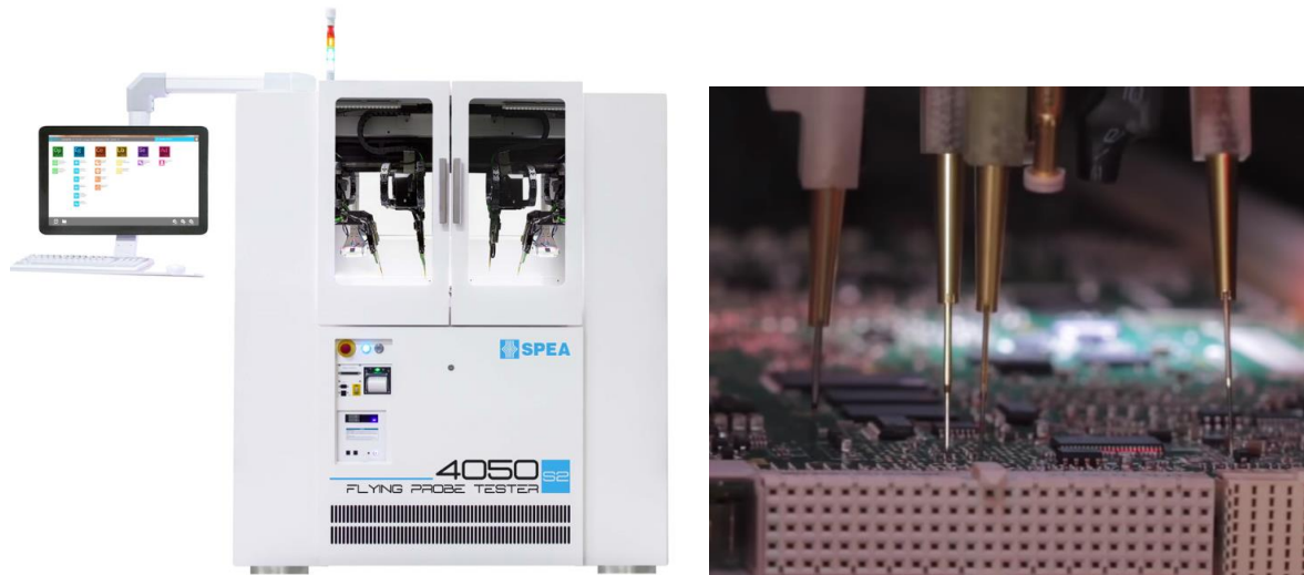
Figure 2.2 Example of Flying Probe Tester & internal testing environment
