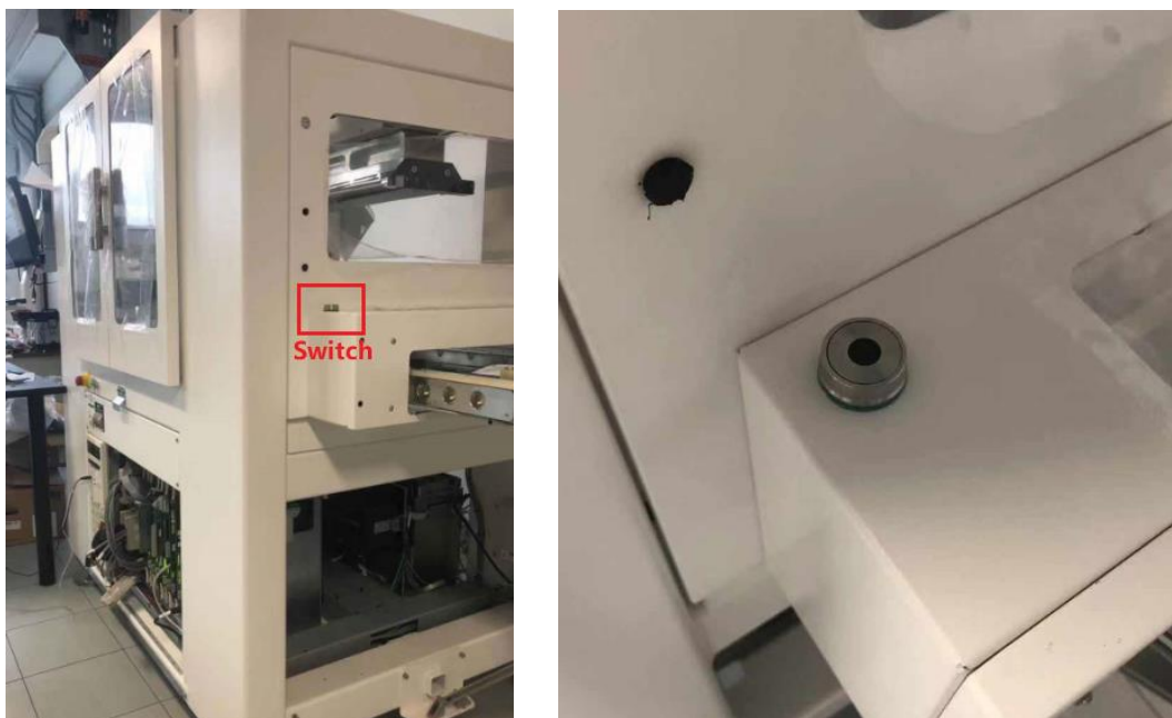
Figure 4.8 Position of the “Execute” switch
