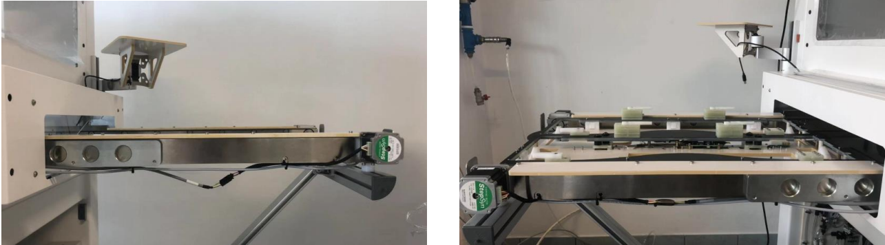
Figure 4.4 one side of conveyer (right side) & Conveyer loaded with washing machine panel (left side)
