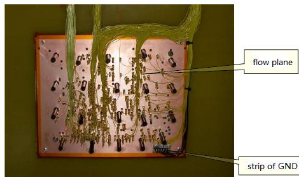
Figure 4.2 Example of the wire structure under the fixture
