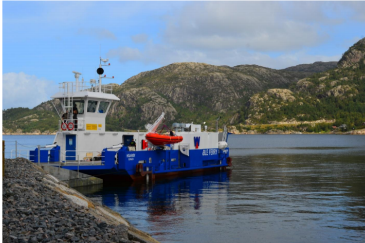
FIGURE 2.8: Electrovaya Electric Cable Ferry [7]
