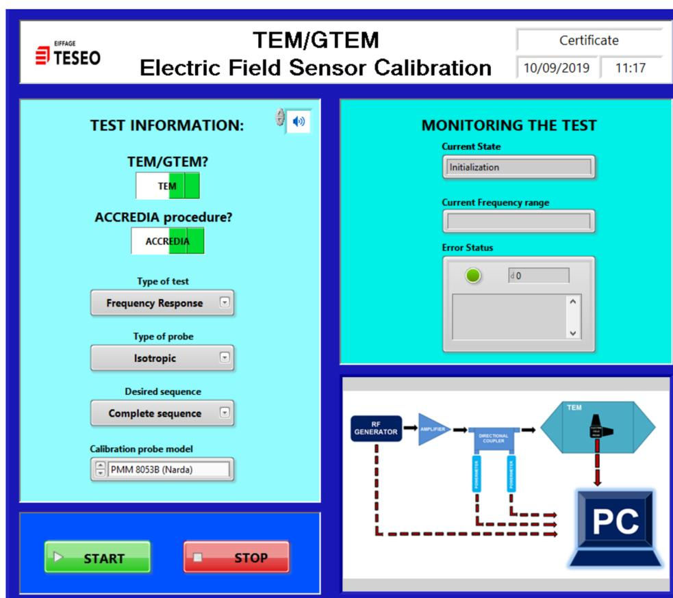
Figure 7.1: Calibration Software, Main VI - Front Panel
