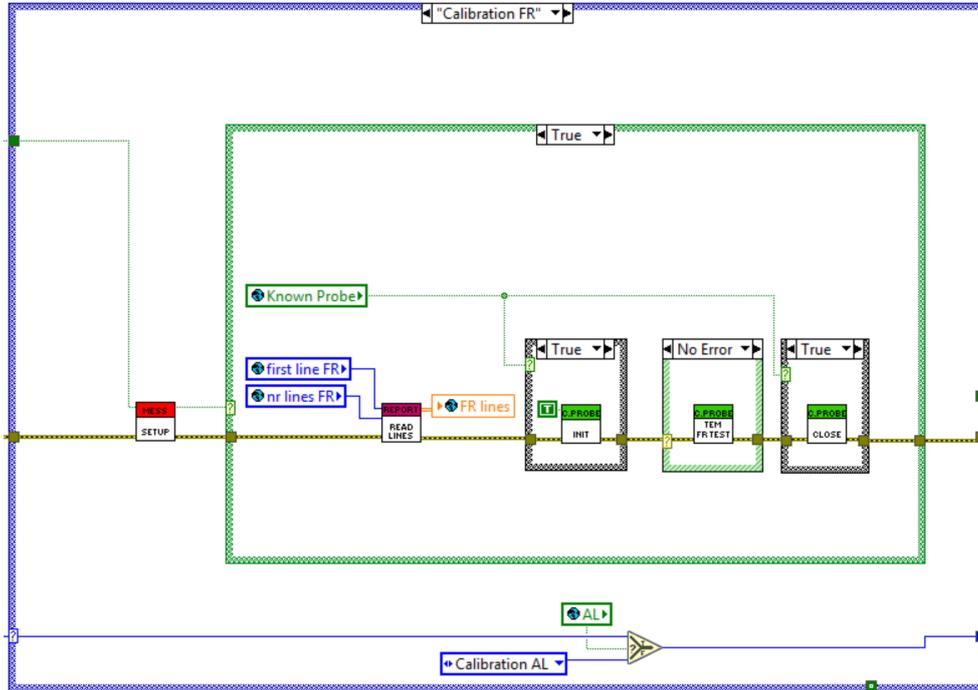
**Figure 7.10:** Calibration Software, Main VI - TEM Frequency Response Test
