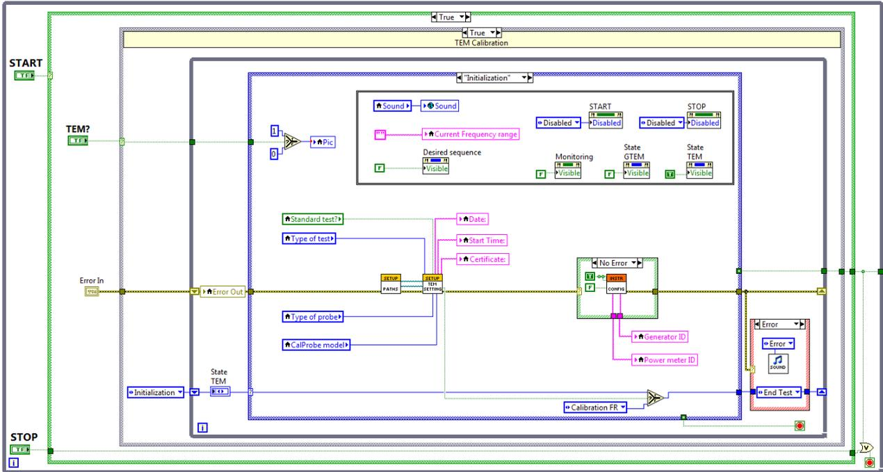
Figure 7.2: Calibration Software, Main VI - Block Diagram
