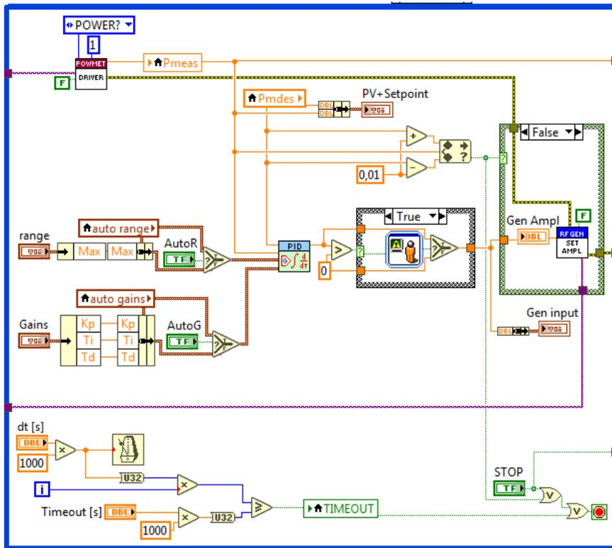
**Figure 7.12:** Calibration Software, Calibration Probe VI - PID controller
