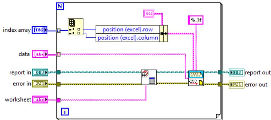
Figure 7.8: Calibration Software, Set Cell Value VI
