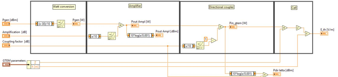
**Figure 8.1:** Plant model in LabVIEW
