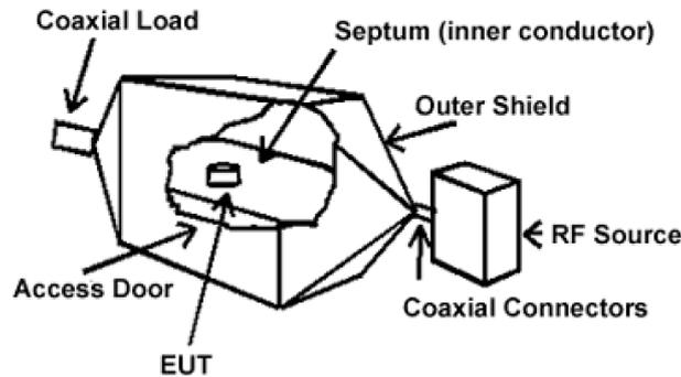
Figure 3.2: TEM cell structure [14]
