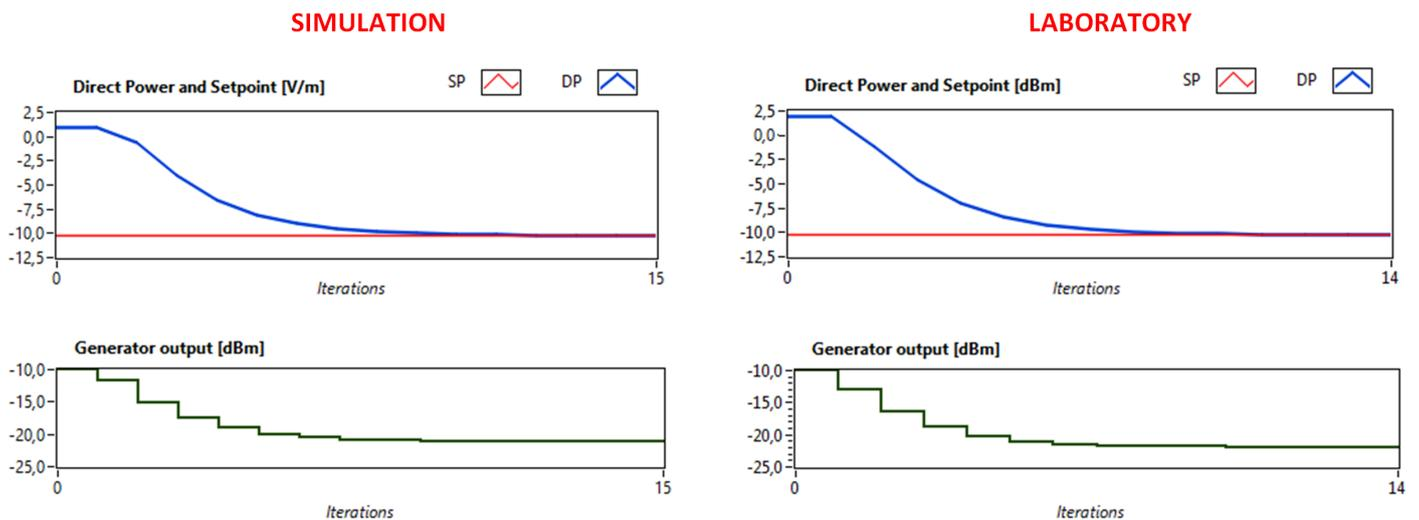
Figure 8.3: PID tuning Calibration Probe - Simulation vs laboratory results
