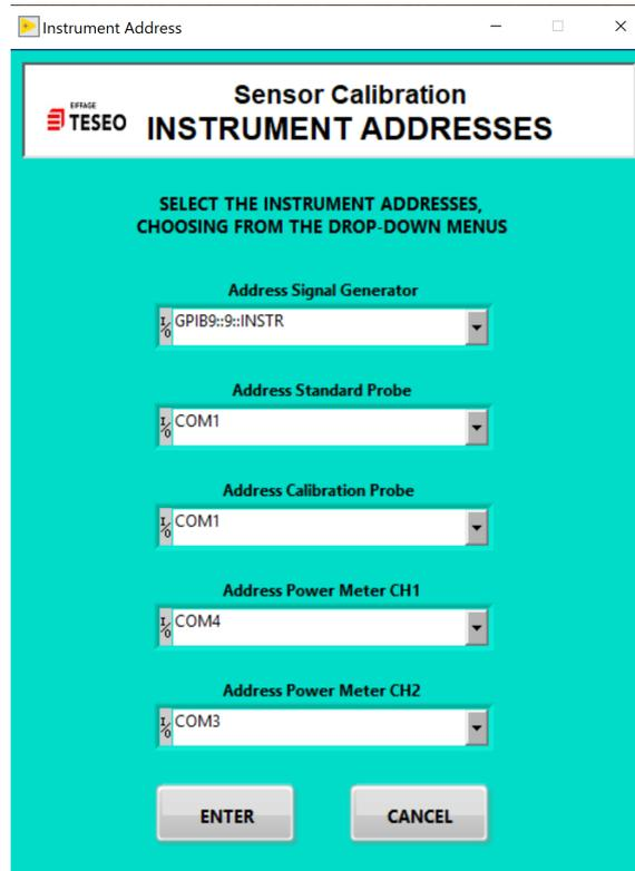
**Figure 7.9:** Calibration Software, Instrument Address VI
