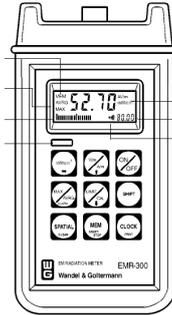
**Figure 5.6:** Wandel & Goltermann EMR-300 Electric Field Sensor [30]
