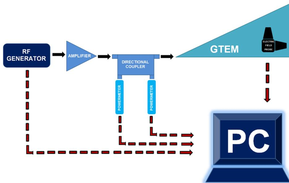
Figure 4.3: GTEM cell measurement scheme
