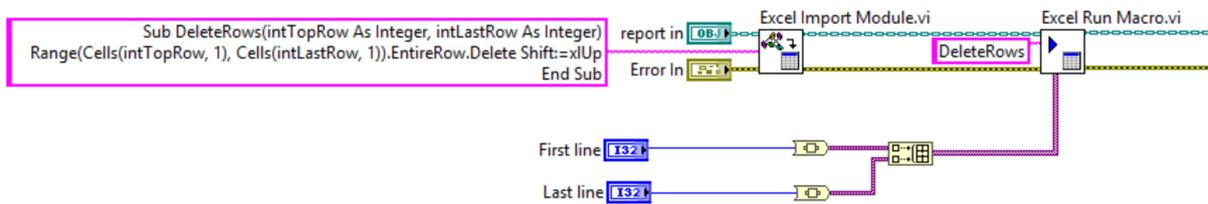
**Figure 7.7:** Calibration Software, Delete rows VI extract - VBA code
