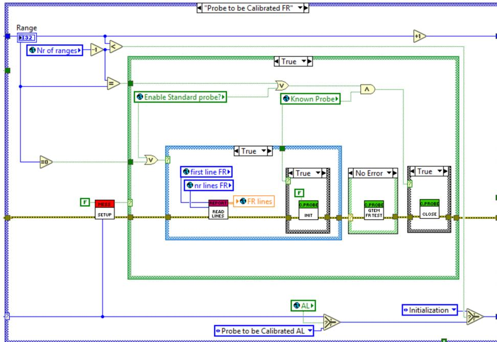
Figure 7.19: Calibration Software, Main VI - Calibration Probe FR Test
