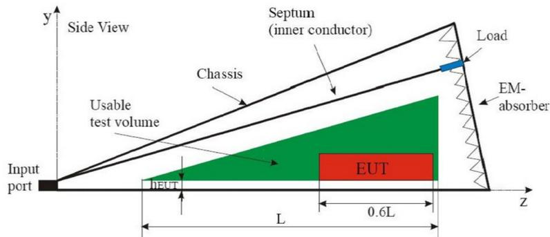
**Figure 3.4:** GTEM cell structure [16]
