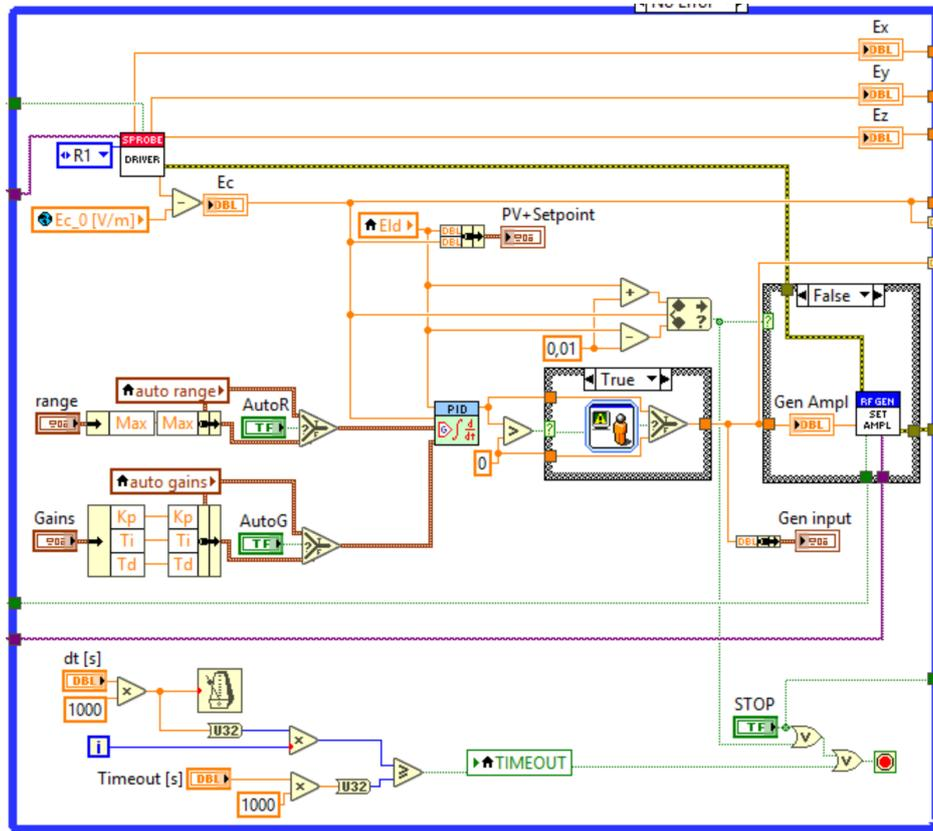
**Figure 7.18:** Calibration Software, Standard Probe VI - PID controller
