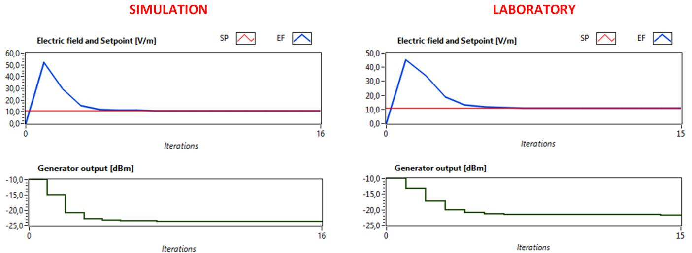
Figure 8.2: PID tuning Standard Probe - Simulation vs laboratory results
