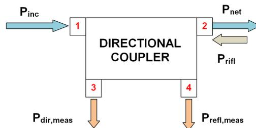
**Figure 5.8:** Directional Coupler scheme
