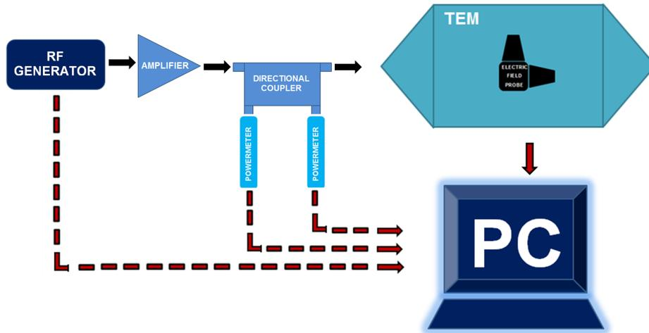
Figure 4.1: TEM cell measurement scheme
