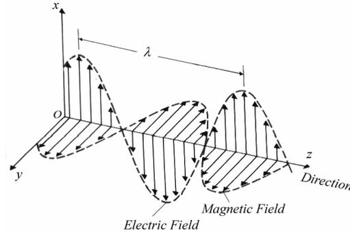
**Figure 3.1:** Electromagnetic wave in far-field [11]
