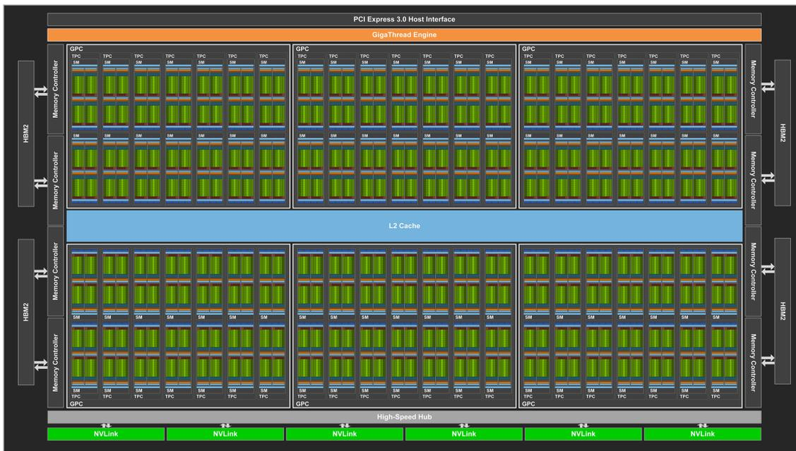
Figure 1.6: The main architecture of NVIDIA
