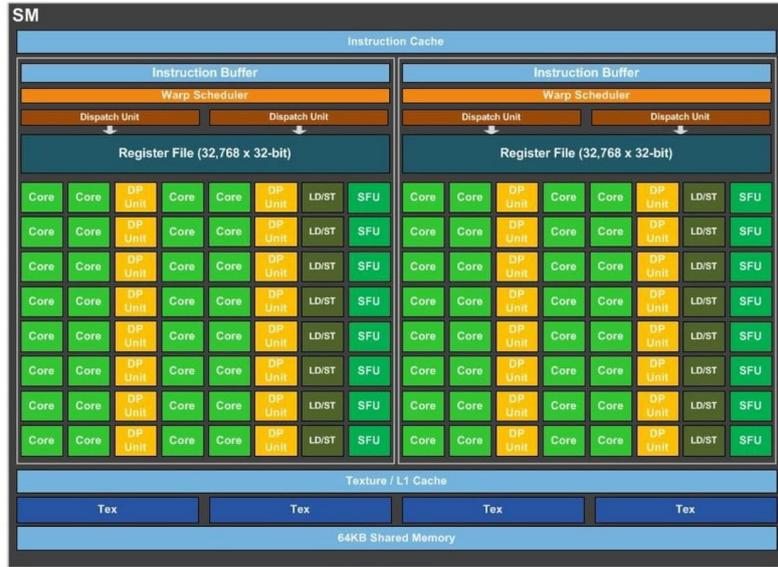
Figure 1.7: Inside Streaming Multi Processor SM
