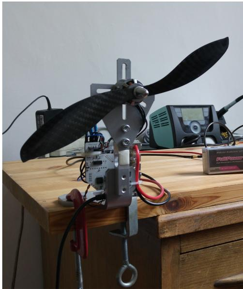
Figure 4.8: Thrust test bench
