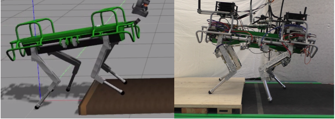
Figure 6.3 – HyQ robot stepping up a pallet of 10cm in both simulation (Gazebo) and hardware experiment.
