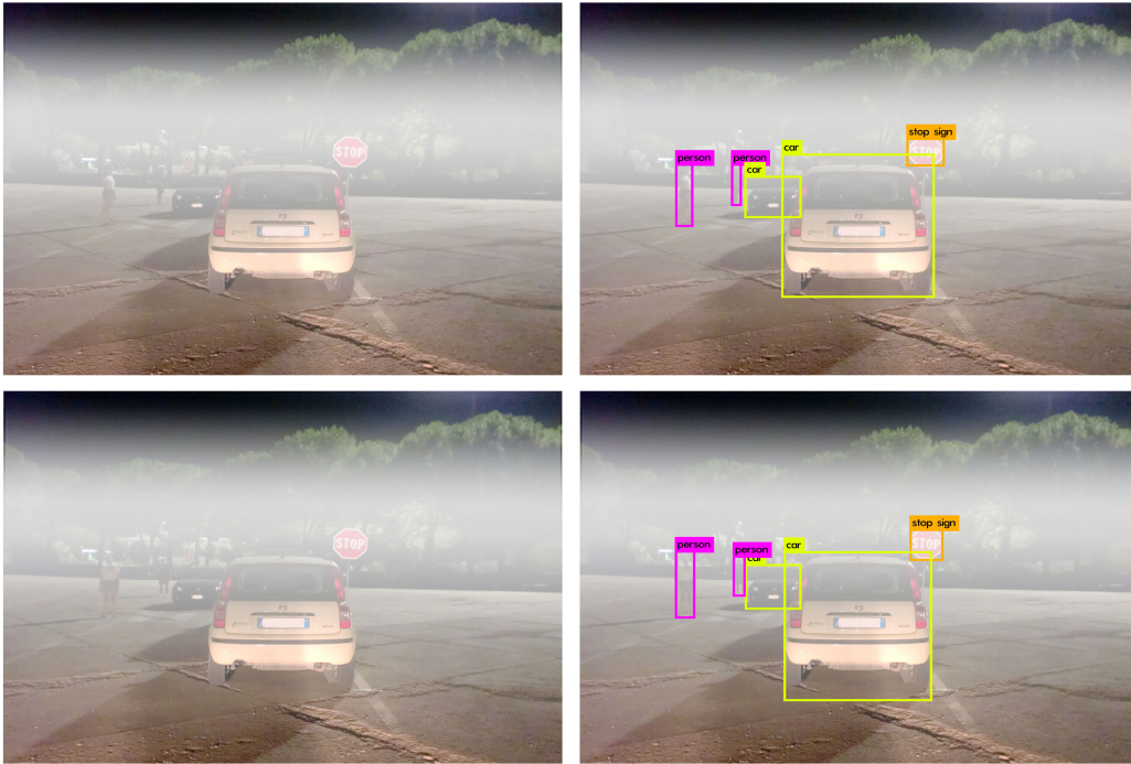
Figure 6.28. Results of the tests performed during the night with light fog at full resolution (car lights ON)
