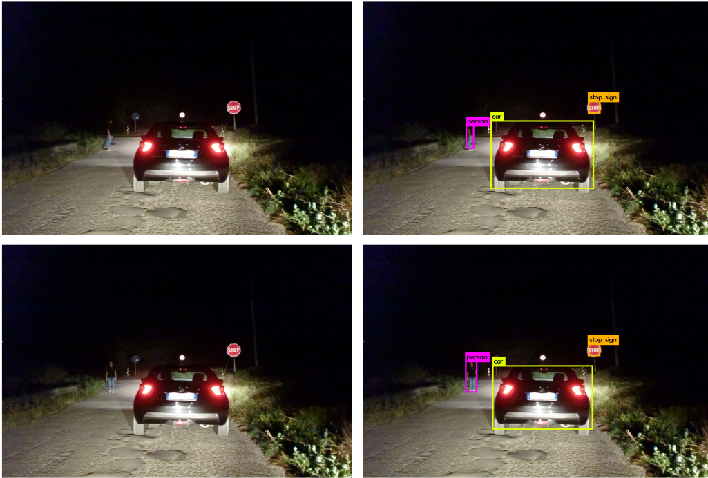
Figure 6.40. Results of the tests performed during the night with a car in front of the vehicle in low light conditions at full resolution (car lights ON)
