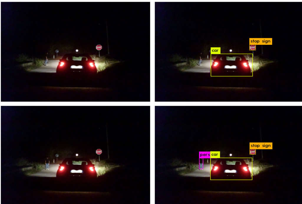
Figure 6.39. Results of the tests performed during the night with a car in front of the vehicle in low light conditions at VGA resolution (car lights OFF)
