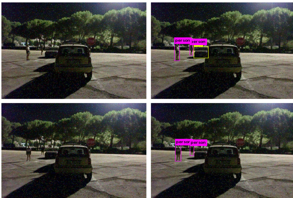
Figure 6.13. Results of the tests performed during the night with micro defects at VGA resolution (car lights OFF)
