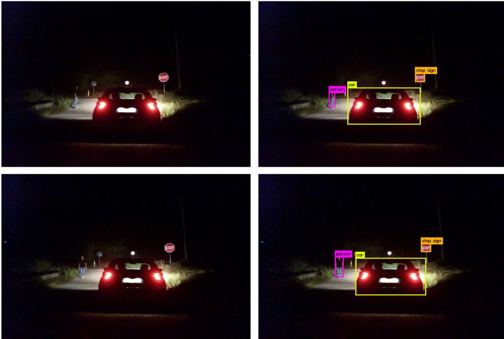
Figure 6.38. Results of the tests performed during the night with a car in front of the vehicle in low light conditions at full resolution (car lights OFF)
