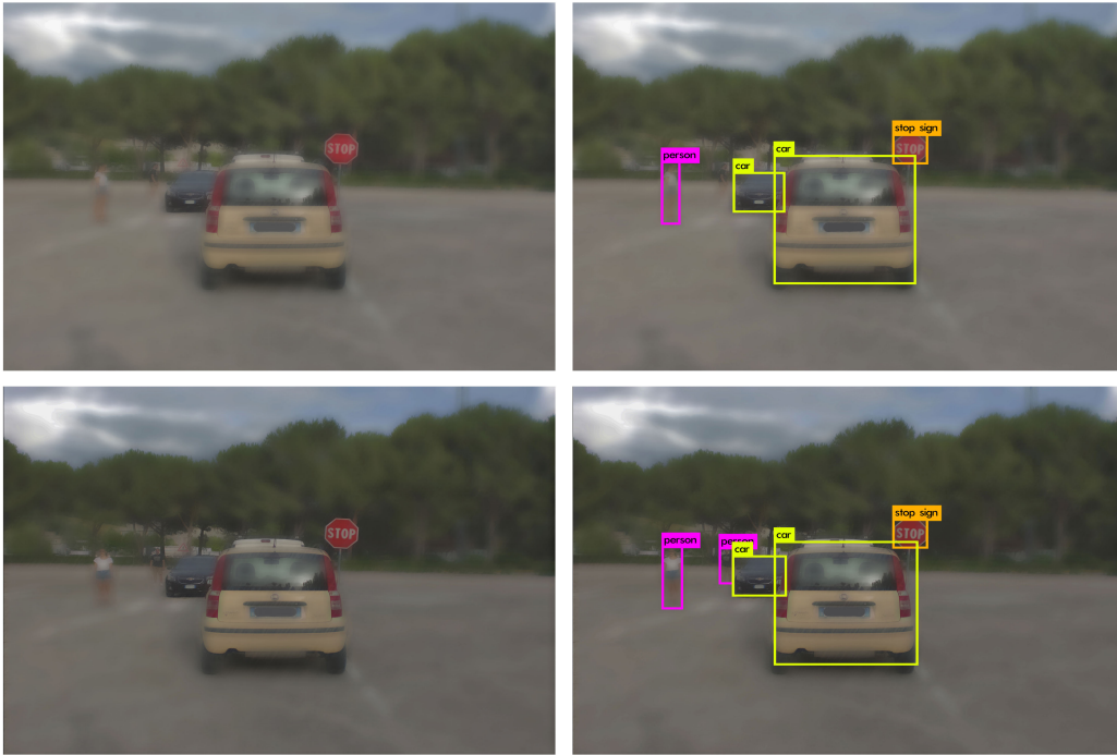
Figure 6.34. Results of the tests performed during the morning with heavy rain simulating the presence of water on the camera glass at full resolution
