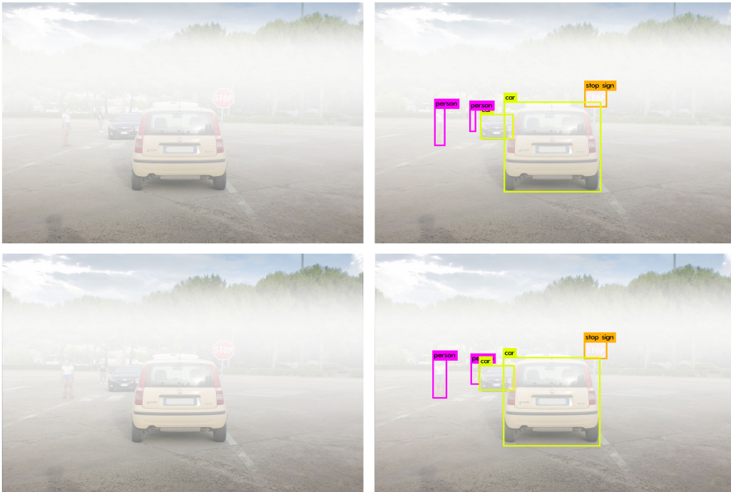
Figure 6.25. Results of the tests performed during the morning with thick fog at full resolution
