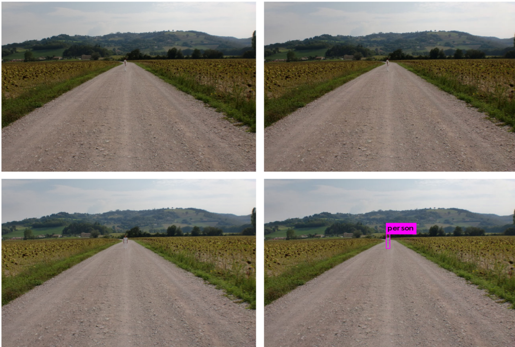
Figure 6.47. Results of the tests performed during the daytime on a white street with a pedestrian dressed in white at VGA resolution
