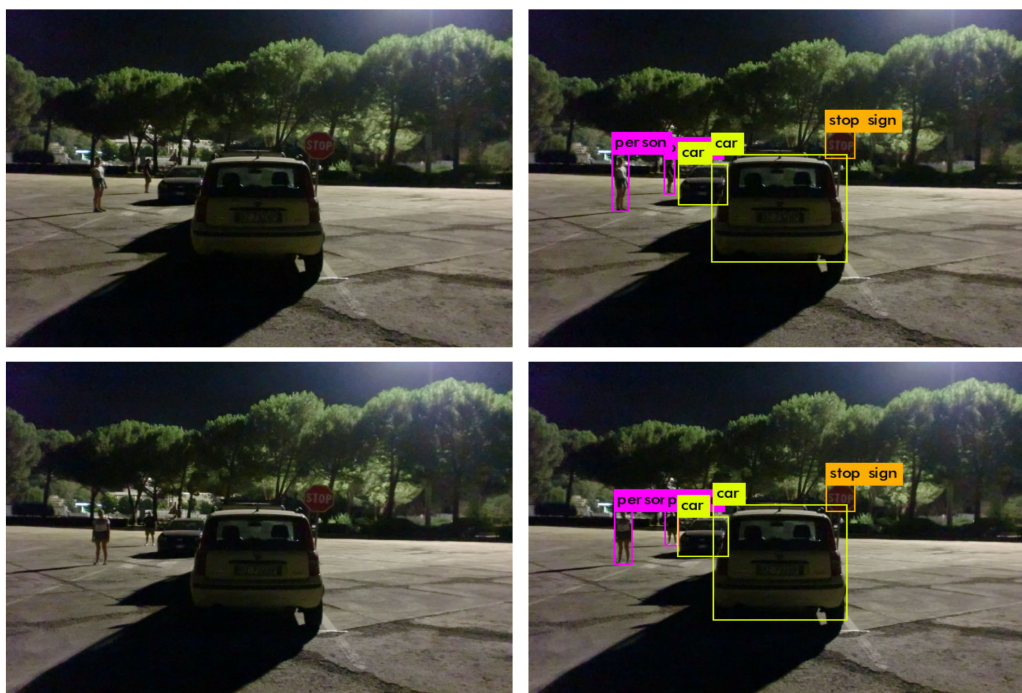
Figure 6.6. Results of the tests performed during the night with VGA resolution (car lights OFF)
