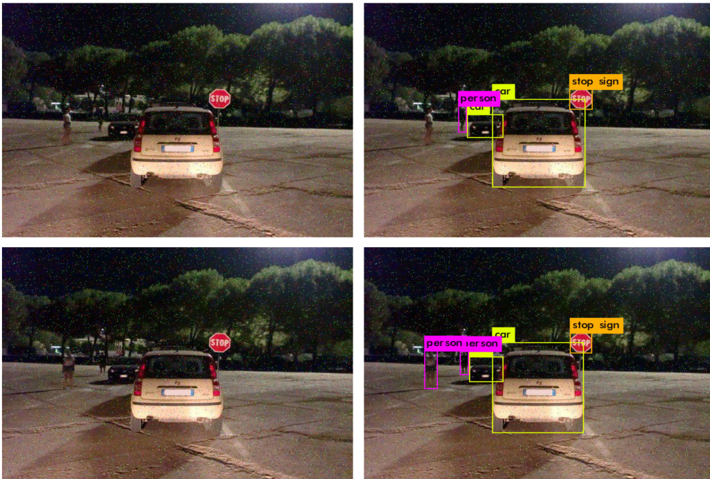
Figure 6.15. Results of the tests performed during the night with micro defects at VGA resolution (car lights ON)
