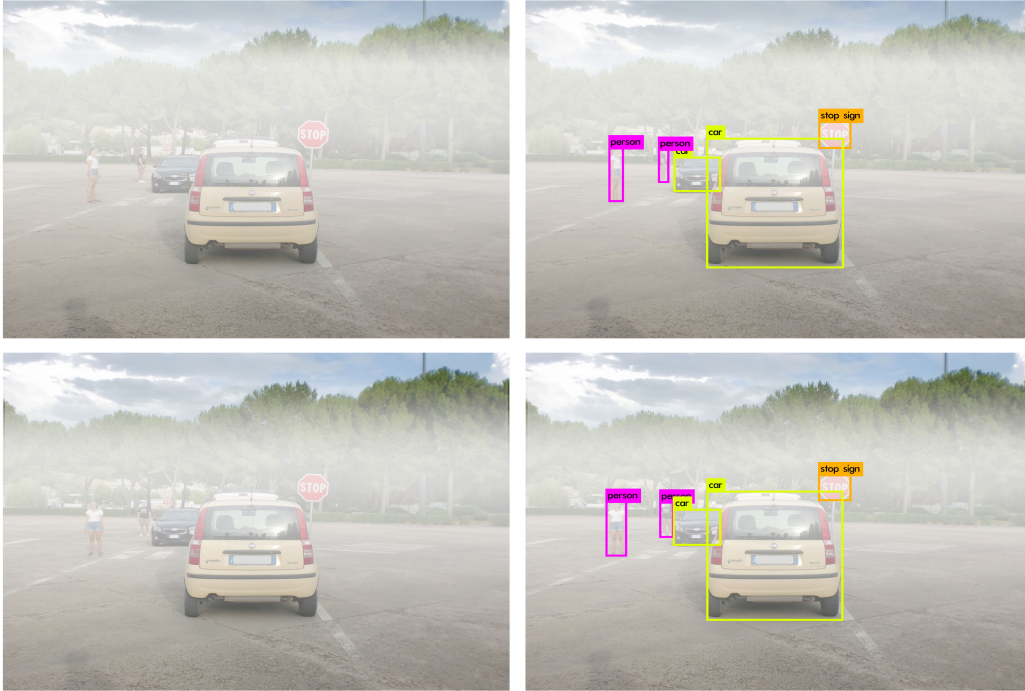
Figure 6.24. Results of the tests performed during the morning with light fog at full resolution
