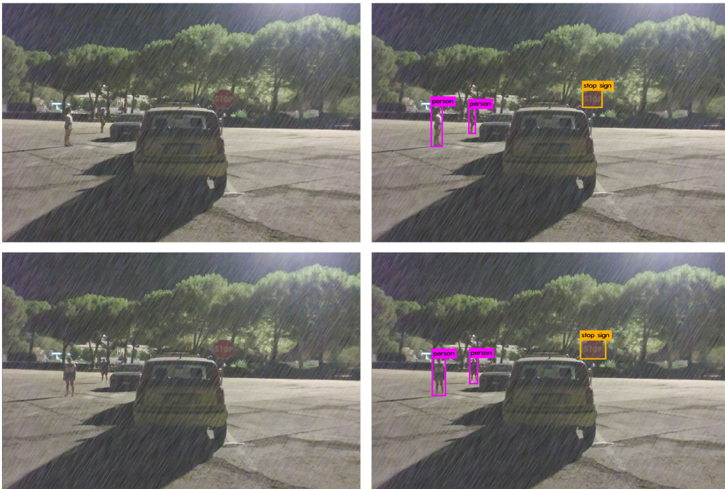
Figure 6.32. Results of the tests performed during the night with heavy rain at full resolution (car lights OFF)
