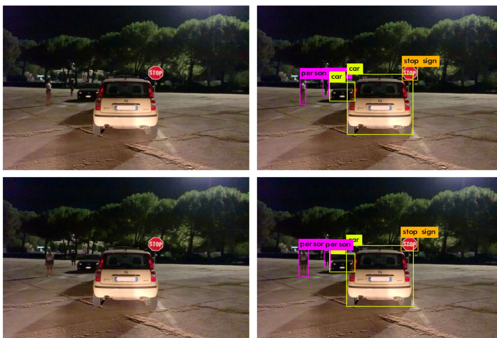
Figure 6.7. Results of the tests performed during the night with VGA resolution (car lights ON)
