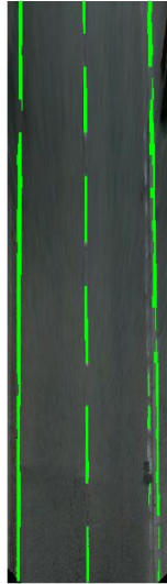
Figure 4.5. Final result during the nightfall with threshold = 8, (lower sensitivity)
