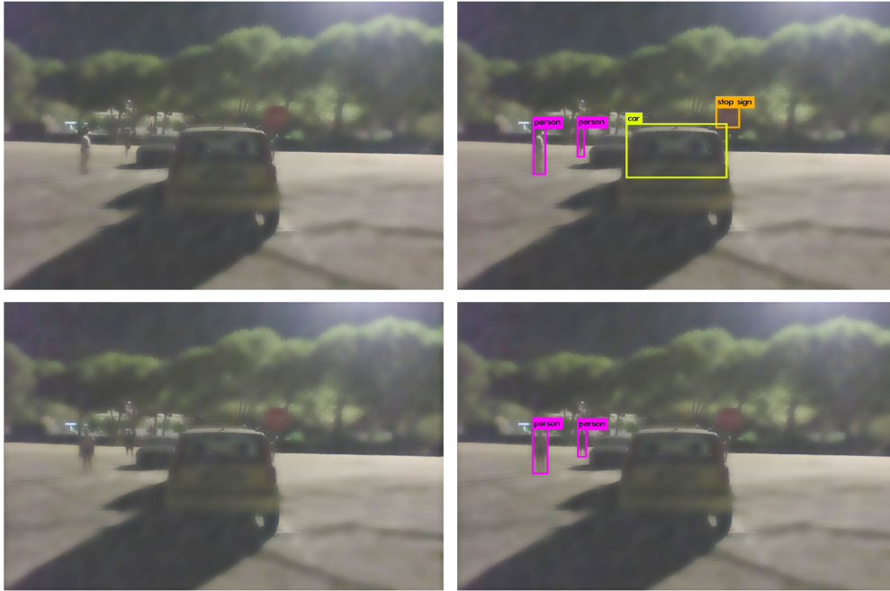
Figure 6.36. Results of the tests performed during the night with heavy rain simulating the presence of water on the camera glass at full resolution (car lights OFF)
