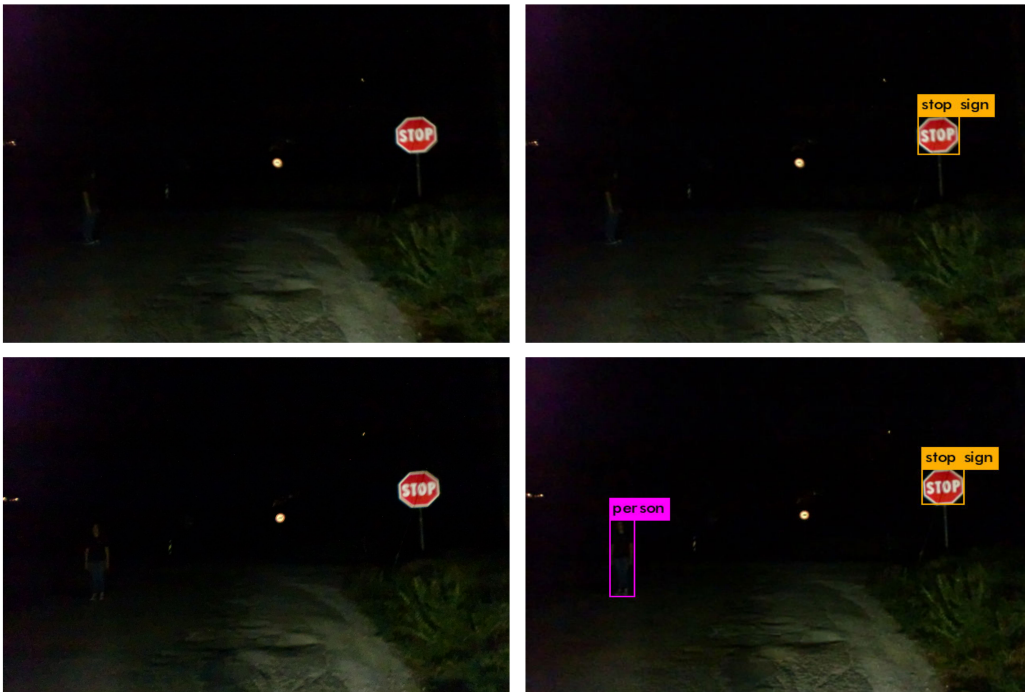
Figure 6.43. Results of the tests performed during the night in low light conditions at VGA resolution (car lights OFF)
