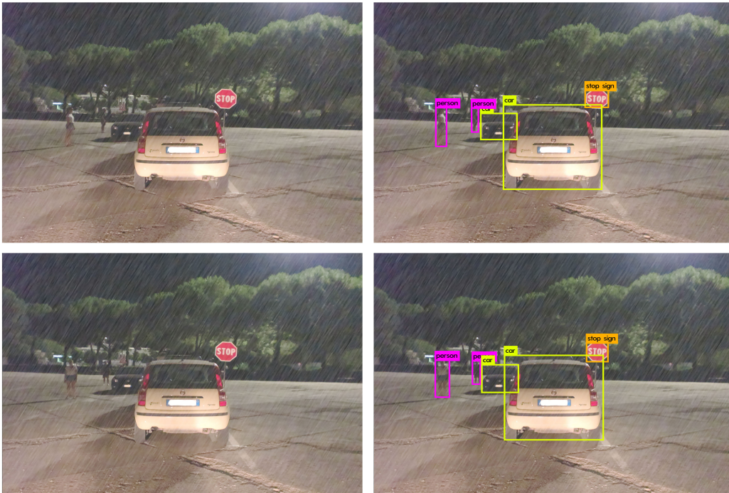
Figure 6.33. Results of the tests performed during the night with heavy rain at full resolution (car lights ON)
