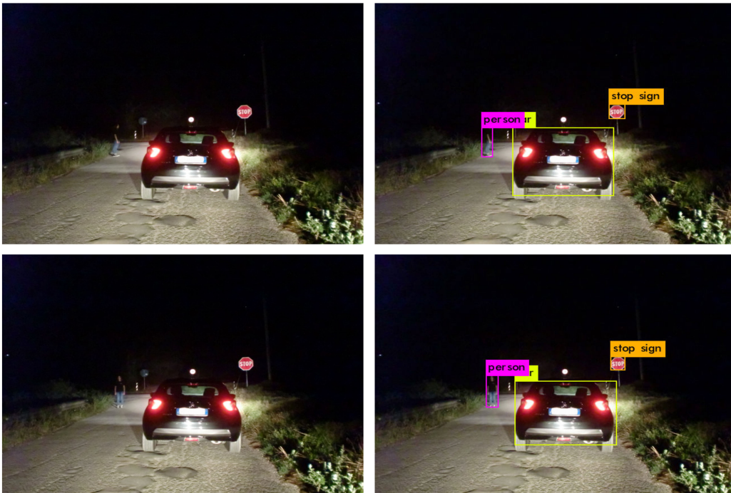
Figure 6.41. Results of the tests performed during the night with a car in front of the vehicle in low light conditions at VGA resolution (car lights ON)
