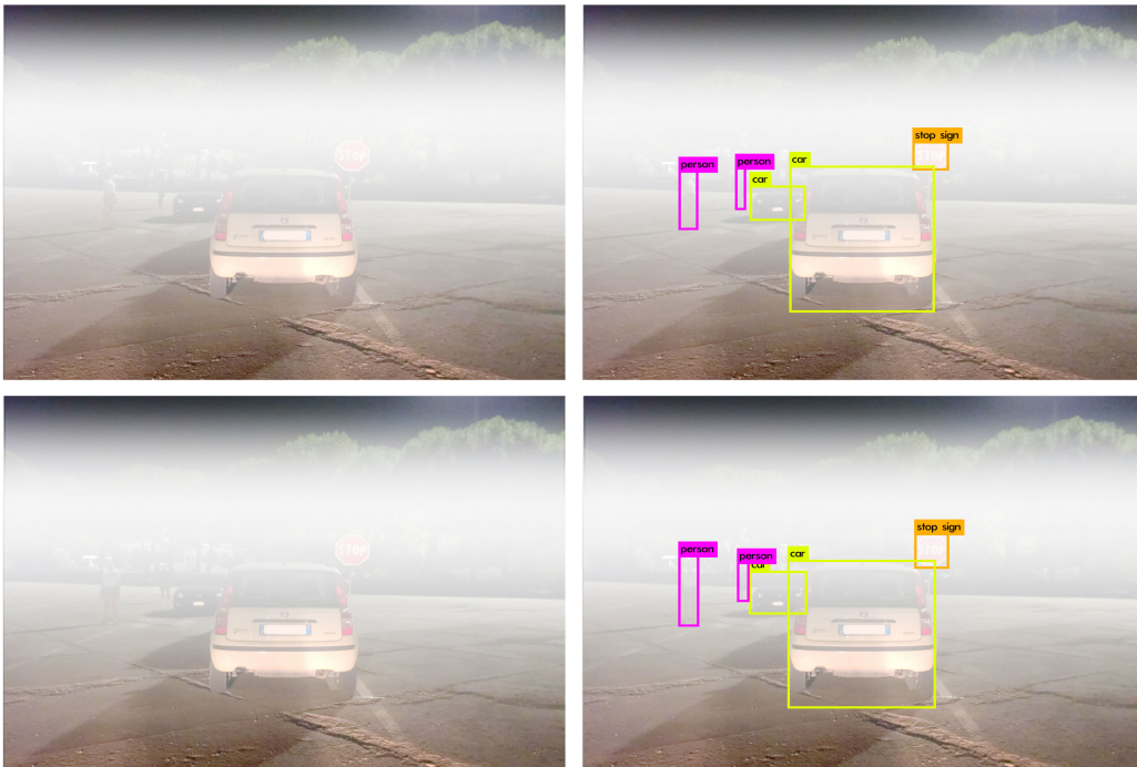
Figure 6.29. Results of the tests performed during the night with thick fog at full resolution (car light ON)
