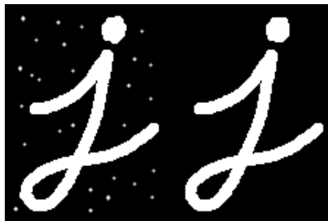
Figure 19: An example of how to use morphological transformations to eliminate noise [11]
