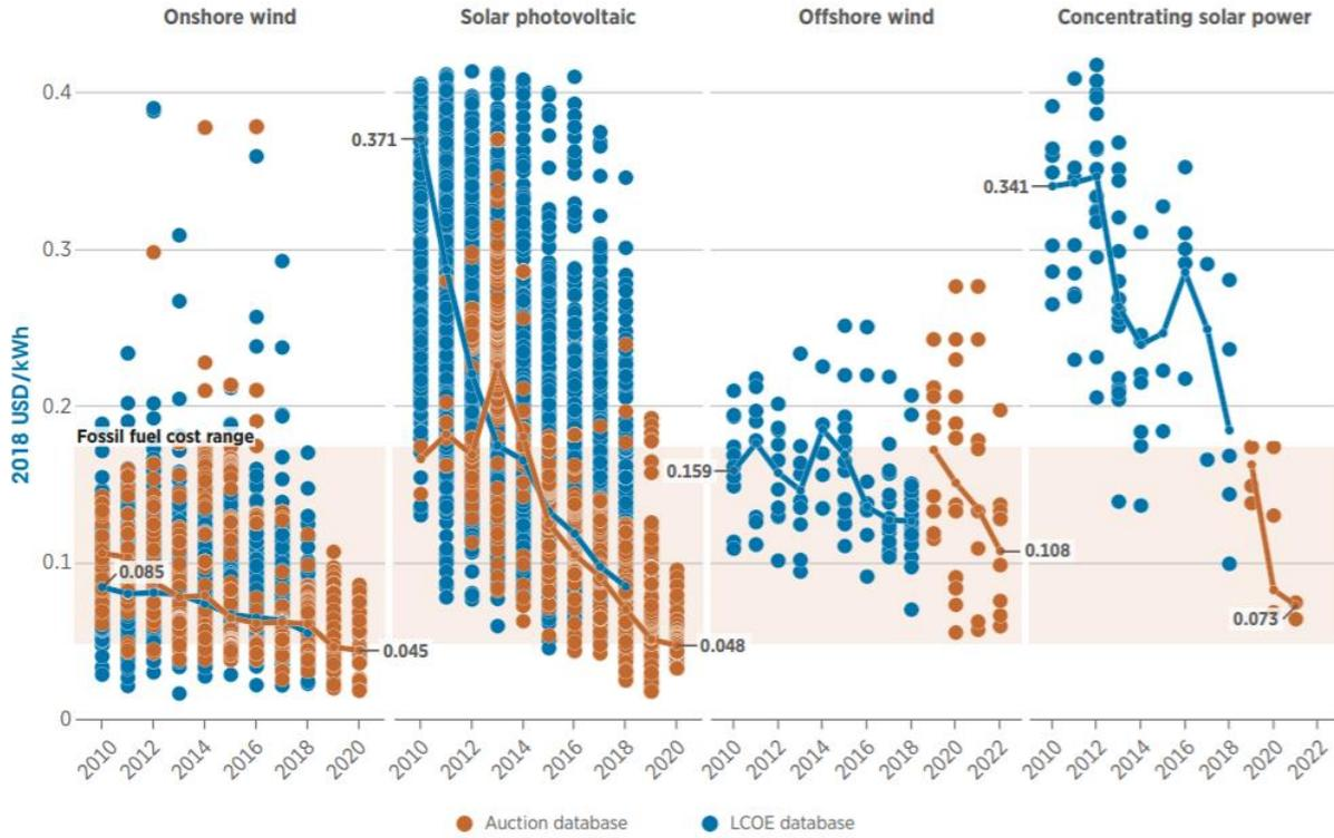
Figure 40: The LCOE for projects and global weighted average value [35]
