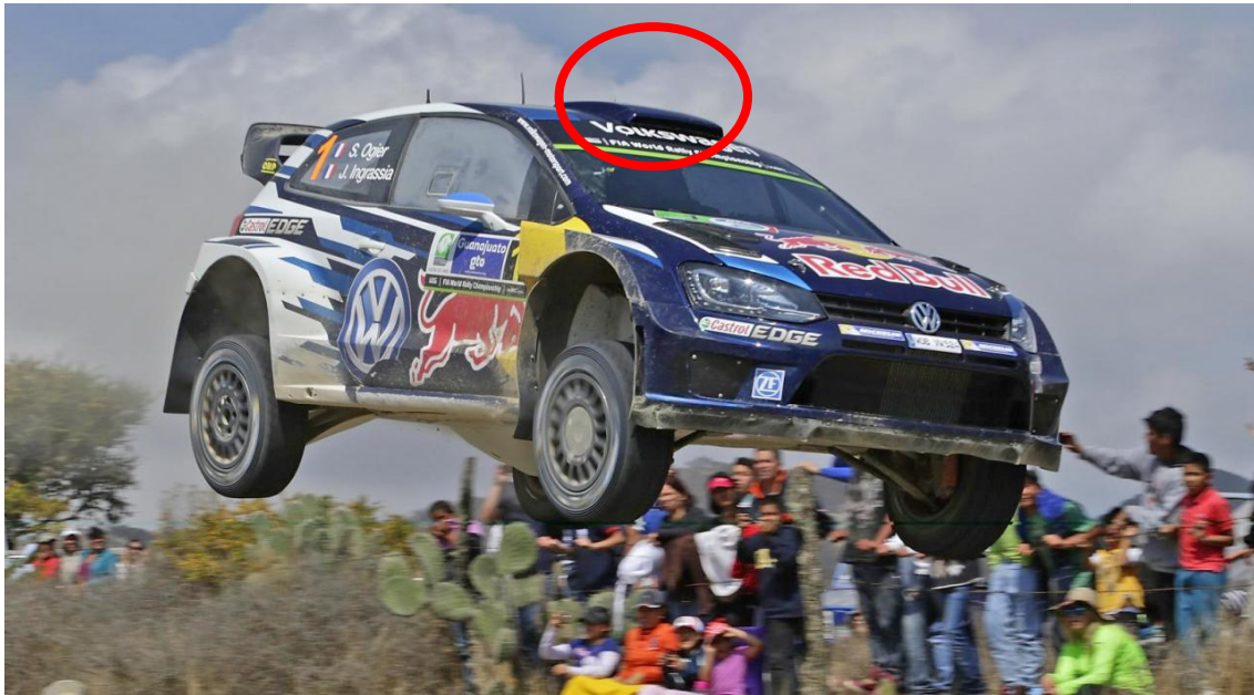
Figure 25 Roof scoop used in rally cars [27]
