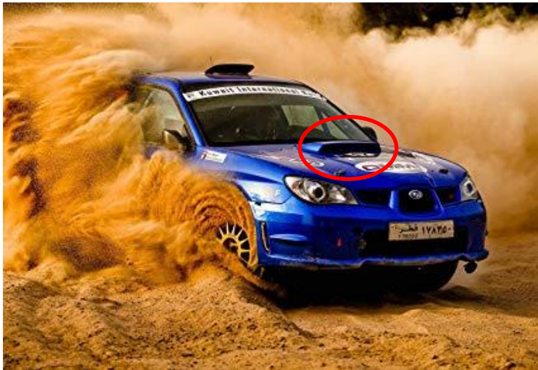
Figure 26 Hood scoop used in rally cars [28]
