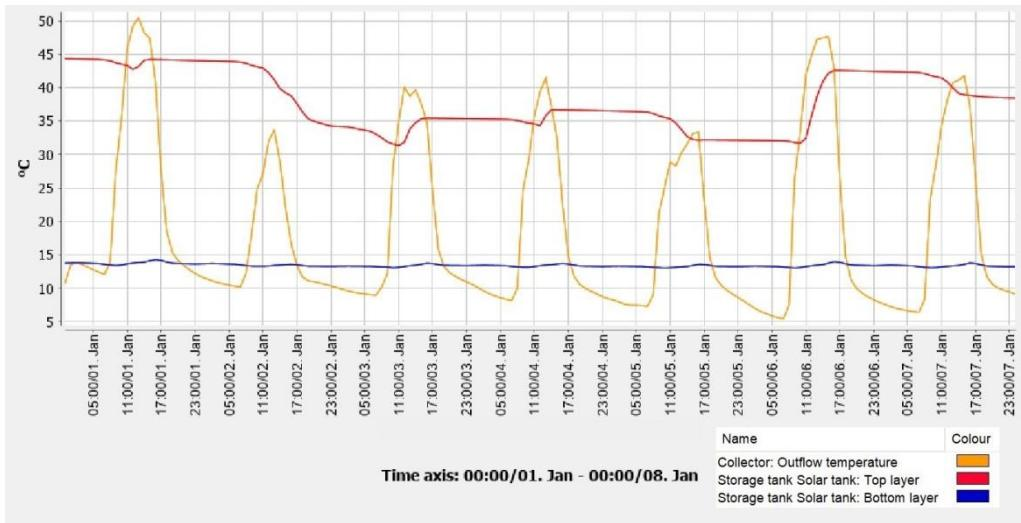
Figure 4.27 Flat plate, temperature evolution first week
