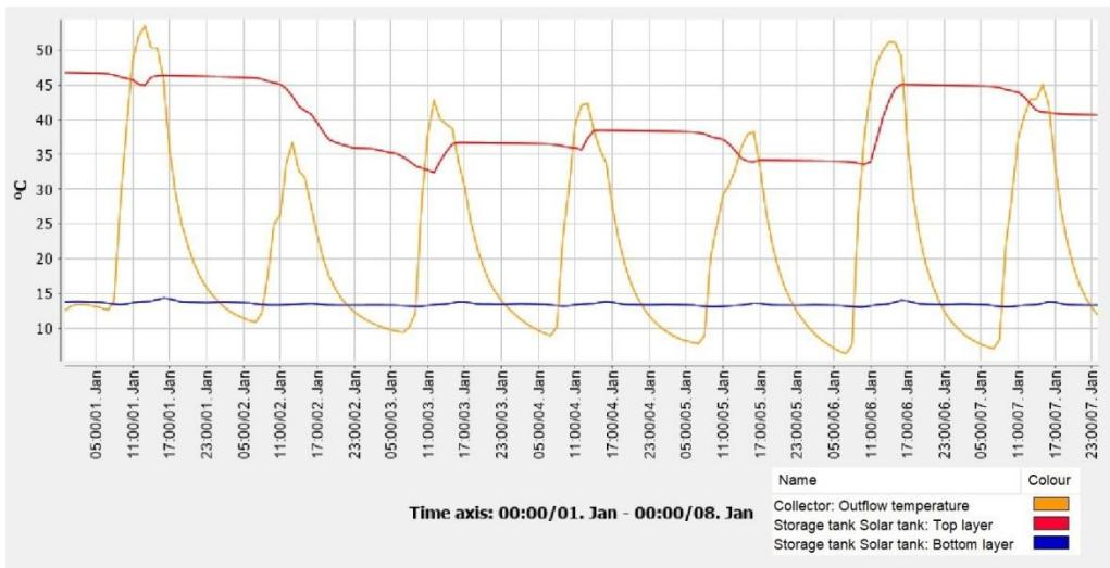
Figure 4.25 Vacuum tube, temperature evolution first week
