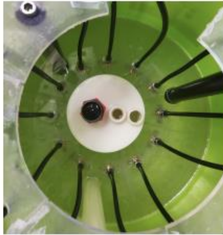
Figure 51: Tank filled with the coupling liquid with phantom and RX/TX antennas inside [7].
