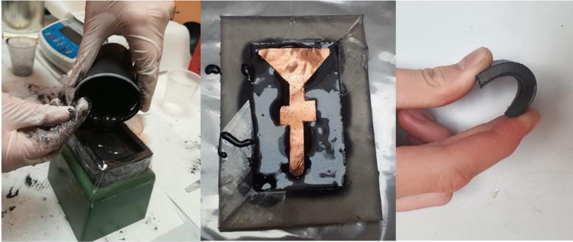
Figure 7.3 (left) Pouring of the liquid G25 mixture in the mold for the 2 cm thick sample. (middle) Finished antenna sample left to dry. (right) Already dried substrate sample without copper that is bent.
