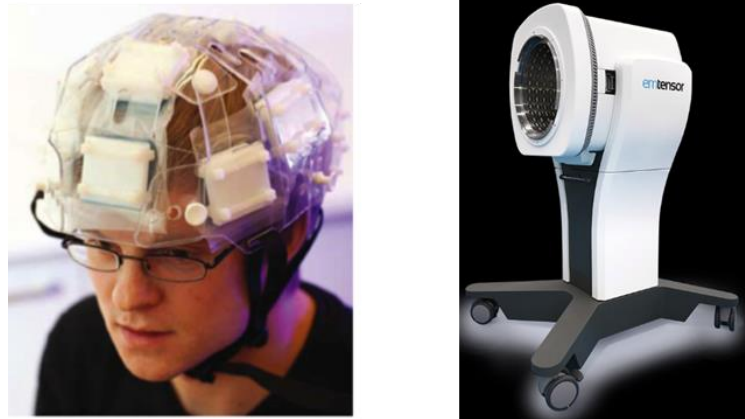
Figure 1.7: Comparison of two different MWI devices developed for brain imaging: the one on left is a prototype of a Sweden group of researchers, the one on right is an EMTensor GmbH product [12] [13].
