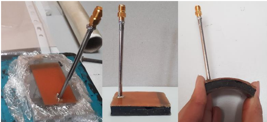
Figure 7.5 (left) Covering of the antenna with urethane rubber layer on both sides. (middle) Lateral view of the finished Antenna Prototype 1. (right) Finished antenna bending.
