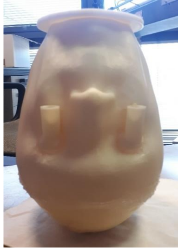
Figure 7.6: 3D printed head phantom used for the measurements made of ABS.
