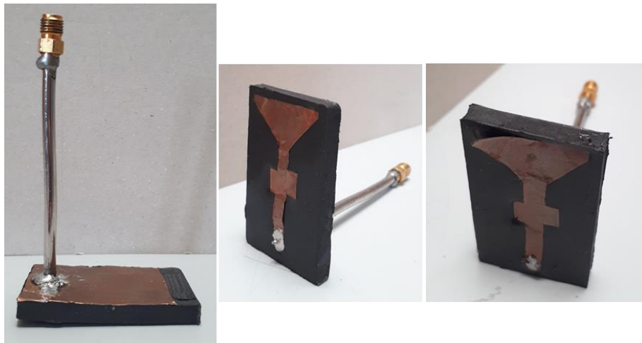
Figure 7.4 (left) Lateral view of welded antenna prototype 1. (middle) Bottom view of the welded antenna prototype 1. (right) Detachment issue of the copper from the substrate.
