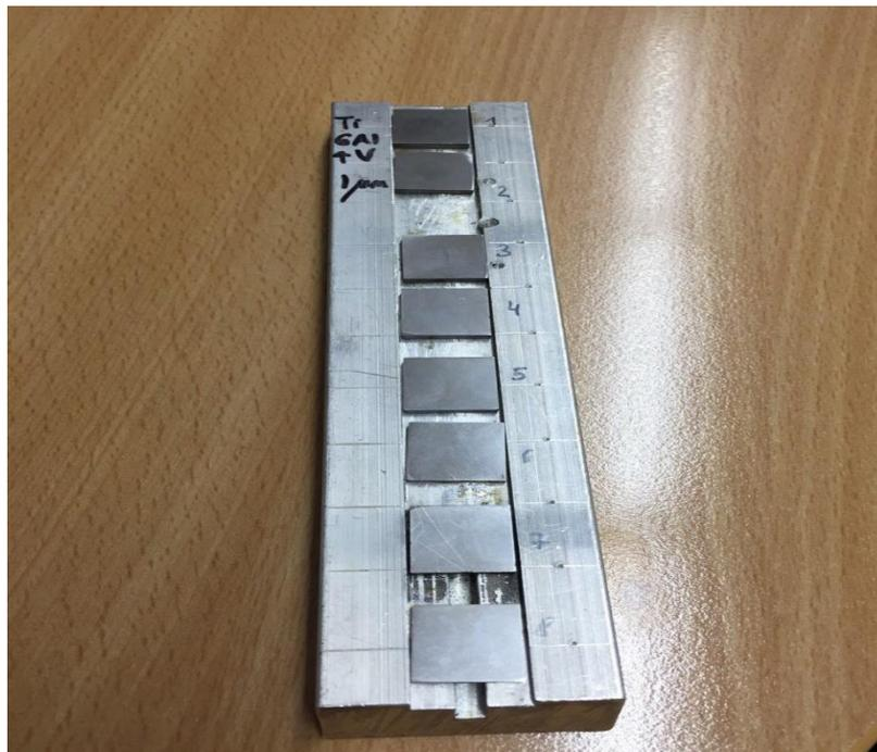
**Figure 4.6** Sample holder with Ti-6Al-4V samples.
