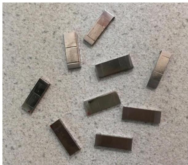
**Figure 4.13** Ti-15Mo cut samples.
