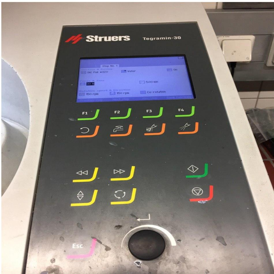
**Figure 4.3** Setting parameters of polishing machine.
