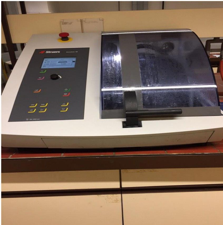
**Figure 4.12** Struers Accutom-10 machine in work phase with the glass closed.
