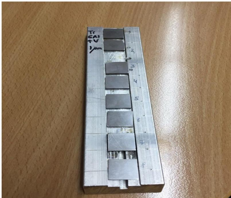
**Figure 4.6** Sample holder with Ti-6Al-4V samples.
