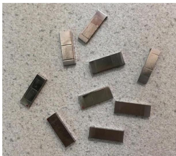
**Figure 4.13** Ti-15Mo cut samples.
