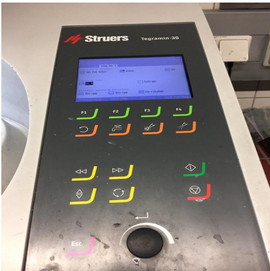
**Figure 4.3** Setting parameters of polishing machine.
