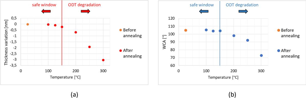
*Figure 5.12: experimental results of thermal study, carried on at 6 different temperatures, for a Co coupon pre-treated with DMAB solution and EtOH, treated with wet-annealing (at 40°C, for 6 minutes) and rinsed with EtOH before spinning. (a) Thickness loss from SE curves; (b) WCA decrease.*
