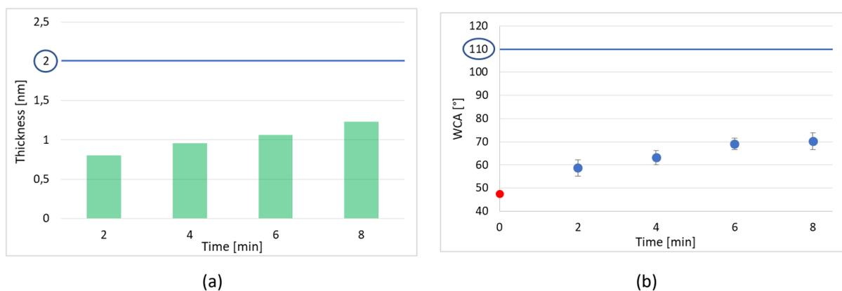
Figure 5.4: experimental results, at different ODT solution contact times, for coupons rinsed with EtOH after spinning. (a) thicknesses from SE curves; (b) WCA values.
