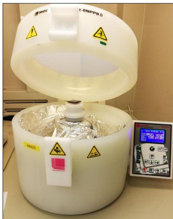
*Figure 4.1: Picture of the spin coater.*
