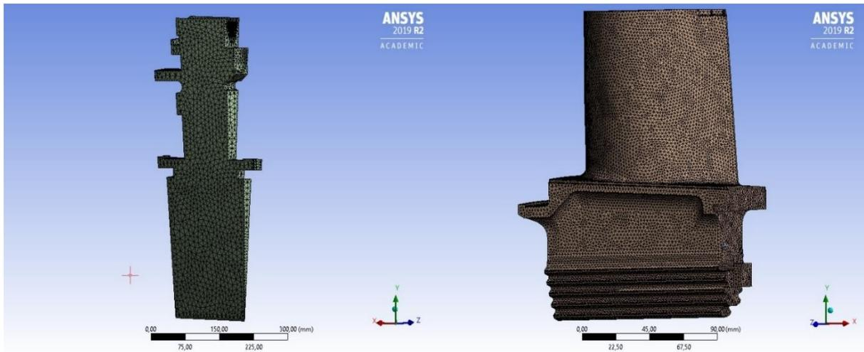
*Figure 3.5: meshes of a single slide of the disk and the blade of a first stage, standard version.*
