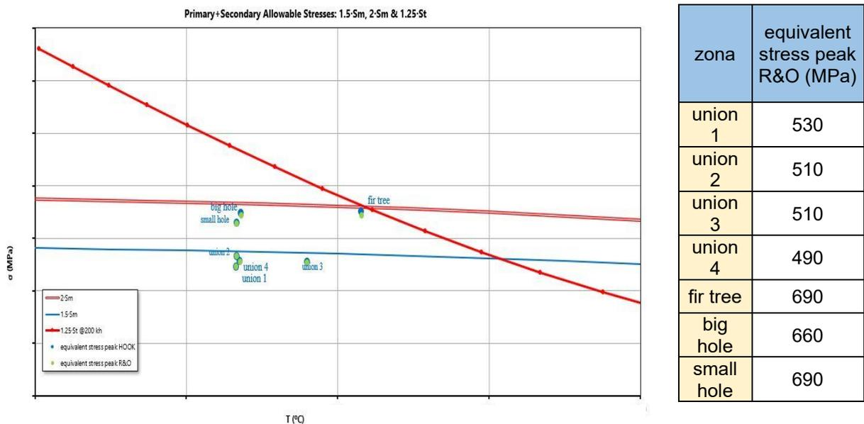
Figure 4.31: peaks of equivalent stress plotted and peak values reported in R&O curve.
