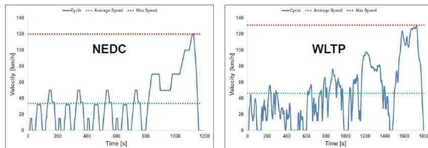
Figure 3.1: NEDC and WLTP cycles
