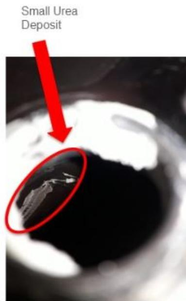
Figure 6.19: SCR inspection after 90 hours with  $\alpha=10$
