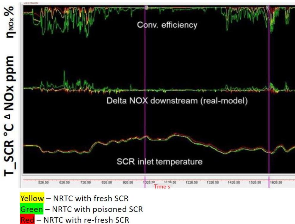
Figure 4.23: 380 °C NRTC cycles comparison
