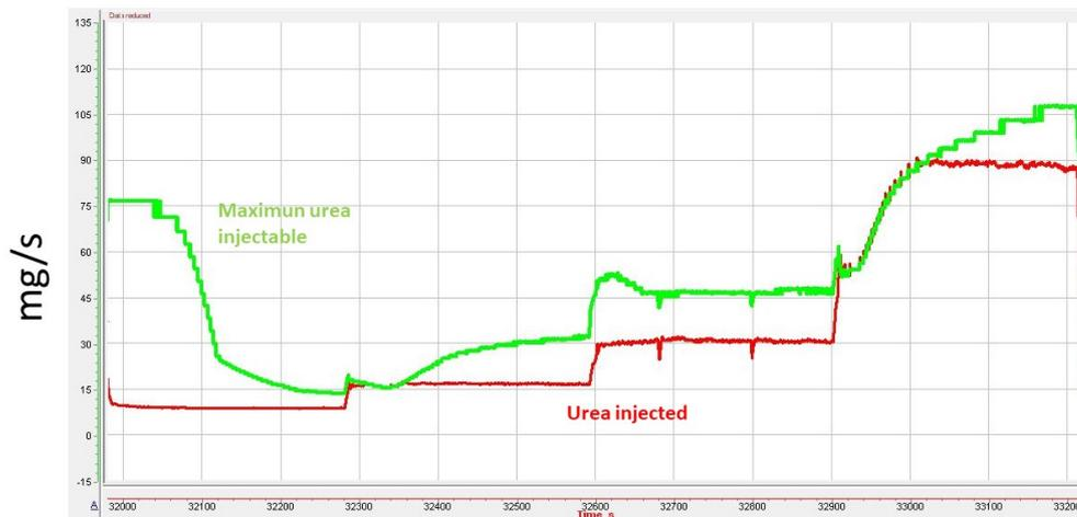
Figure 6.13: Urea injected vs. urea injectable with  $\alpha=2$
