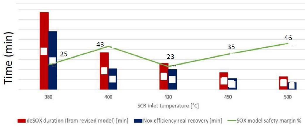
Figure 4.22: DeSOx times comparison
