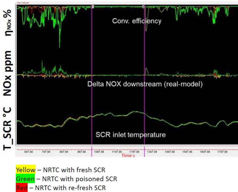
Figure 4.26: 500 °C NRTC cycles comparison
