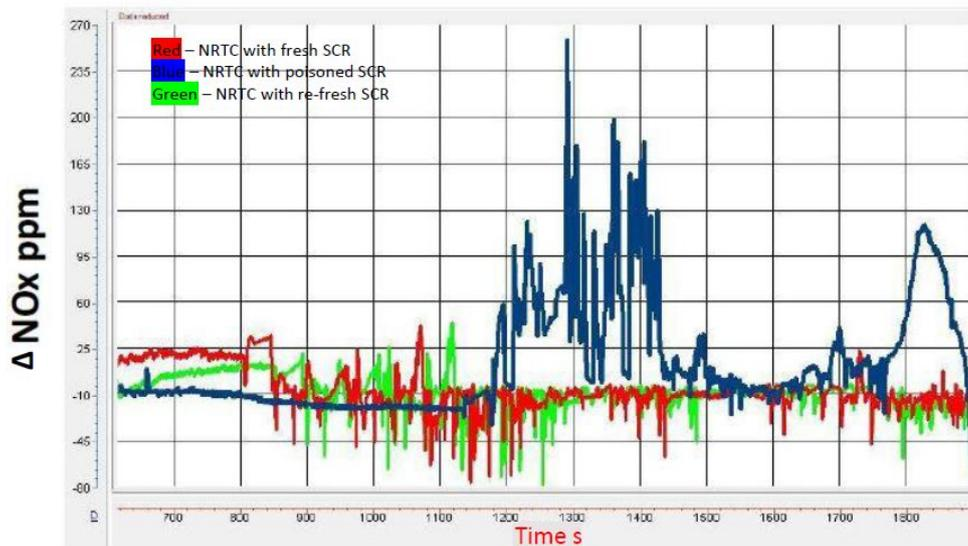
Figure 4.10:  $\Delta_{NO_x}$  NRTC-transient cycles comparison
