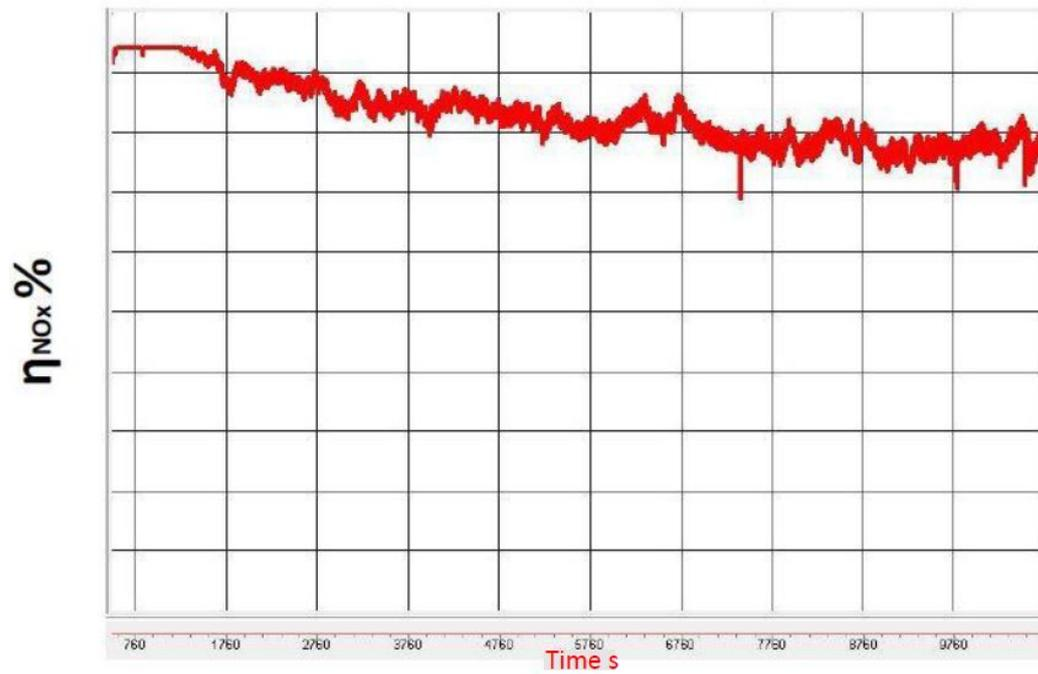
Figure 4.15:  $\eta_{NO_x}$  during poisoning phase
