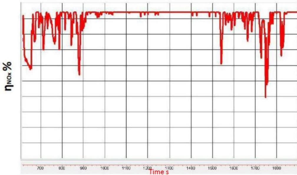
Figure 4.7:  $\eta_{NOx}$  NRTC-transient cycle fresh SCR
