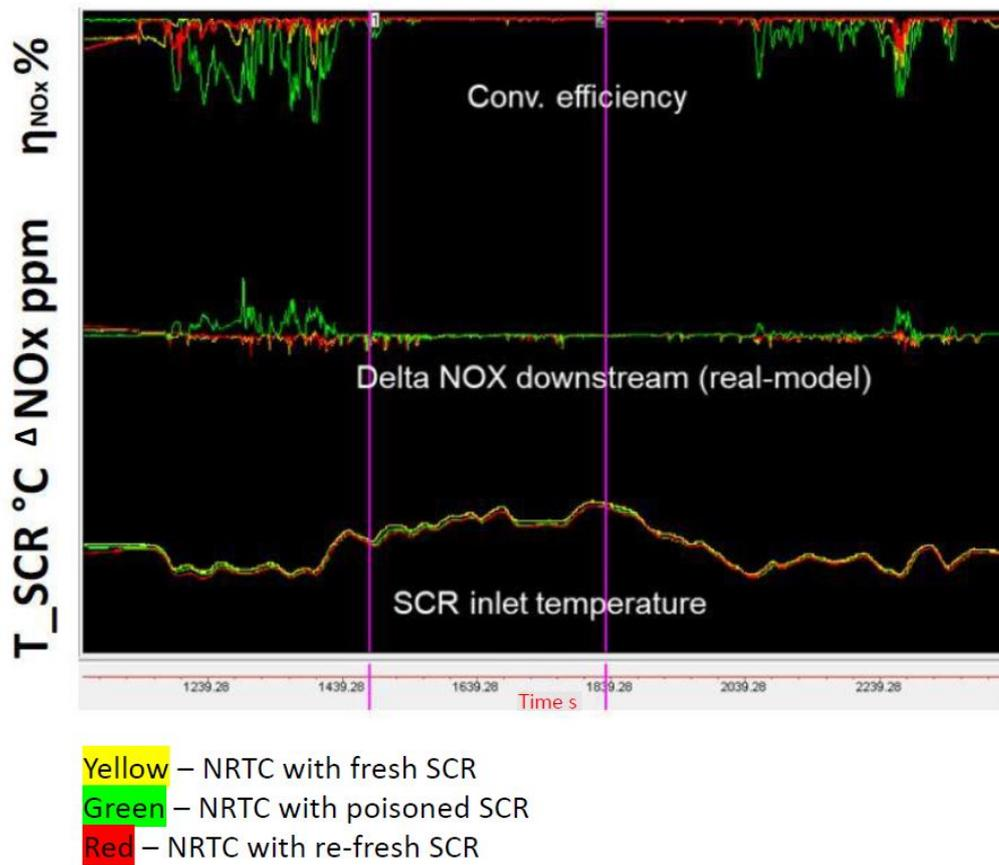
Figure 4.25: 420 °C NRTC cycles comparison
