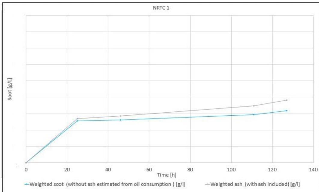
Figure 5.5: Soot accumulated on NRTC 1
