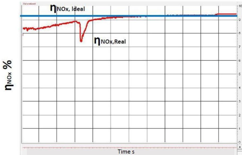
Figure 4.21:  $\eta_{NO_x, Real}$  and  $\eta_{NO_x, Ideal}$  during the DeSOx phase
