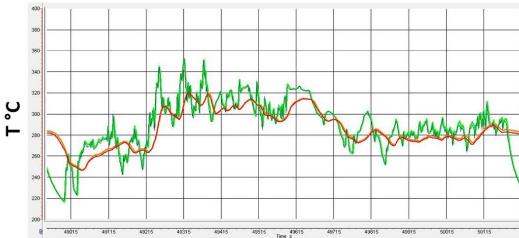
Figure 5.4: Exhaust gases temperatures on DOC and DPF with NRTC transient cycle
