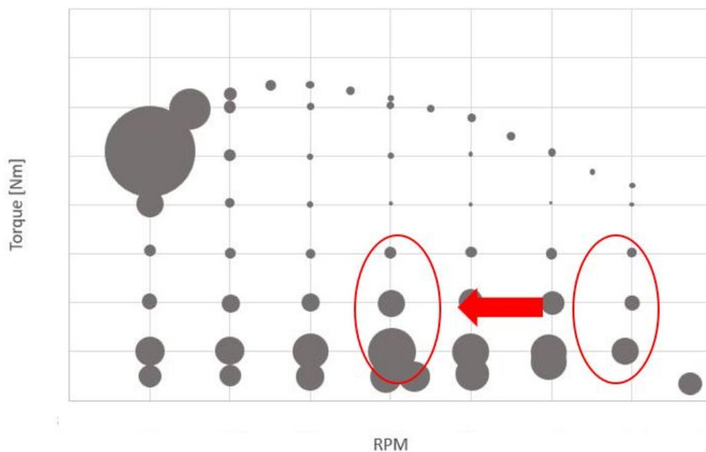
Figure 5.12: Engine operating points downwards shift
