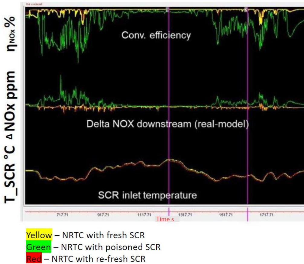
Figure 4.24: 400 °C NRTC cycles comparison
