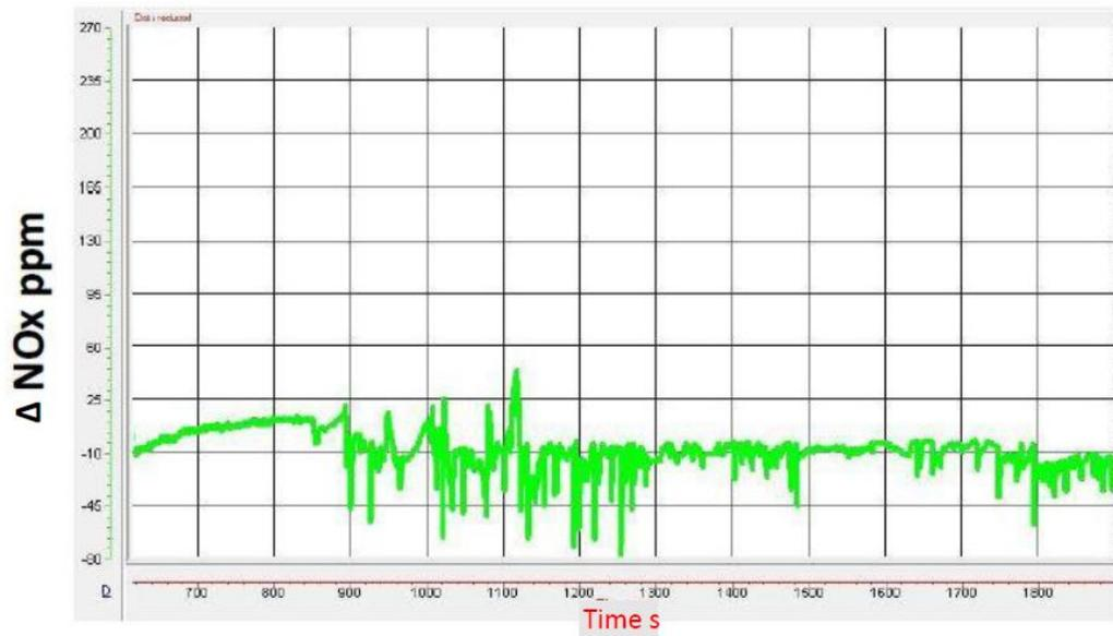
Figure 4.13:  $\Delta_{NO_x}$  NRTC-transient cycle re-fresh SCR
