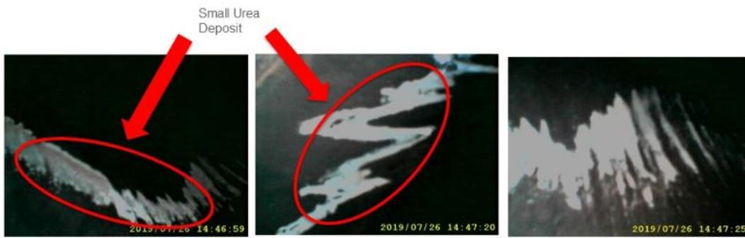
Figure 6.18: SCR inspection after 40 hours with  $\alpha=10$
