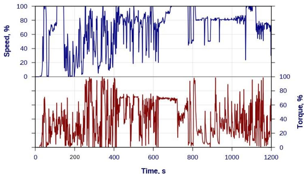
Figure 3.9: Normalized Speed and Torque NRTC profile
