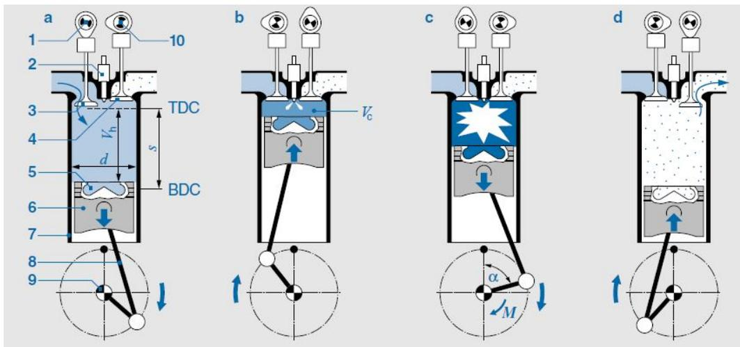
Figure 1.2: Four stroke Diesel engine operating cycle
