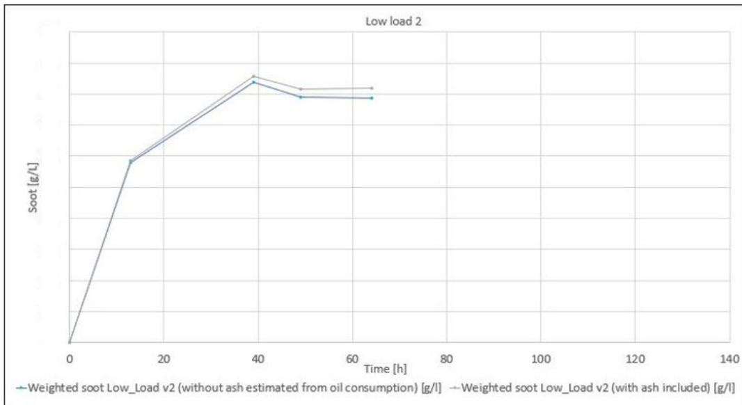
Figure 5.13: Soot accumulated on Low load v2
