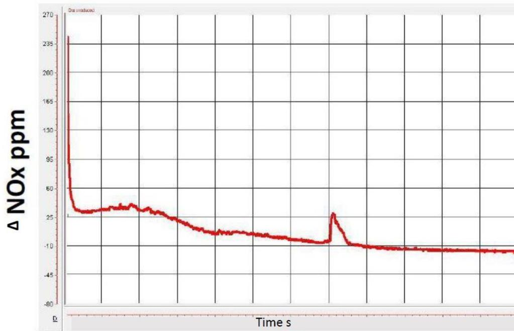
Figure 4.20:  $\Delta NO_x$  parameter during DeSOx phase
