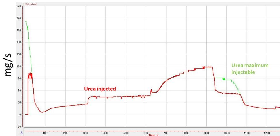
Figure 6.14: Urea injected vs. urea injectable with  $\alpha=10$
