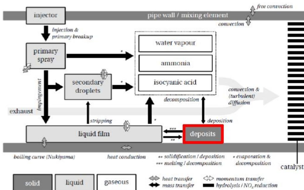
Figure 6.1: Model of SCR Urea deposits
