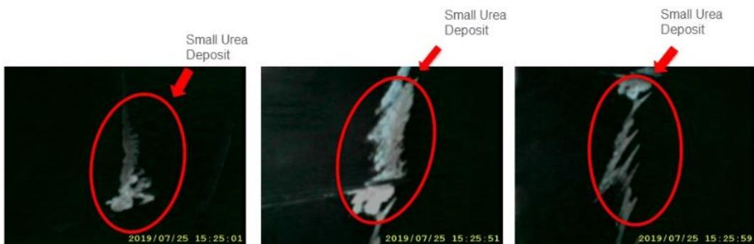
Figure 6.17: SCR inspection after 20 hours with  $\alpha=10$
