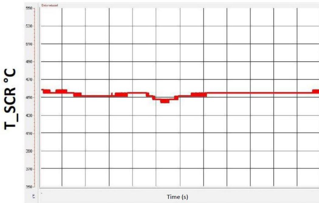
Figure 4.18:  $T_{SCR}$  °C during DeSOx phase
