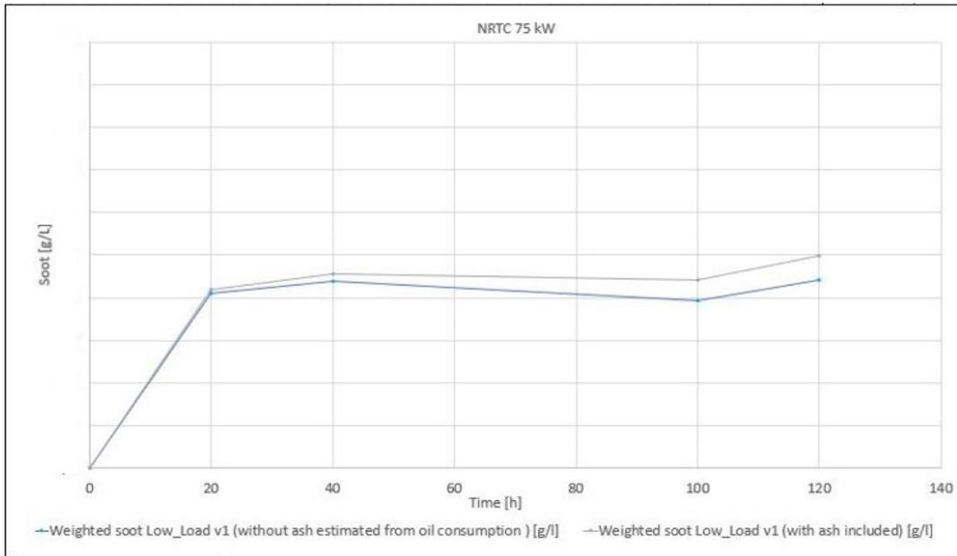
Figure 5.7: Soot accumulated on NRTC with a power reduced calibration
