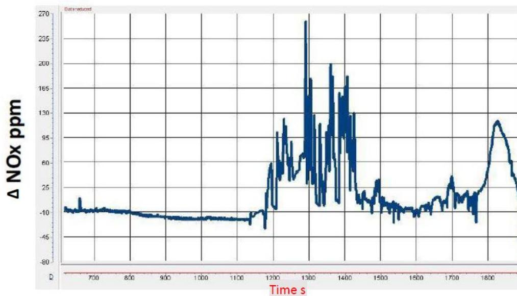
Figure 4.12:  $\Delta NO_x$  ppm NRTC-transient cycle poisoned SCR
