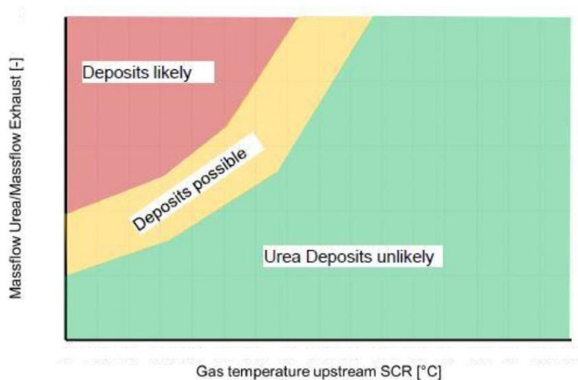
Figure 6.3: MassflowUrea/MassflowExhaust vs Temperature upstream SCR defines critical urea deposit zone
