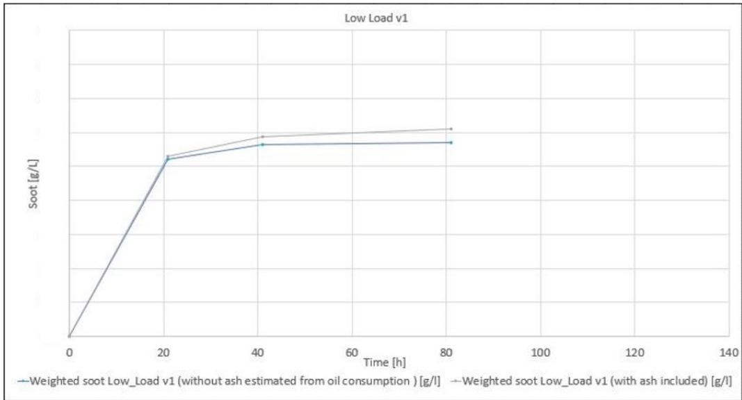
Figure 5.10: Soot accumulated on Low load v1
