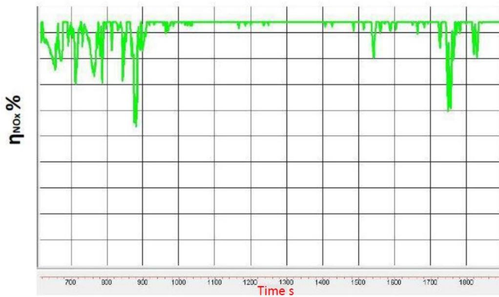
Figure 4.9:  $\eta_{NO_x}$  NRTC-transient cycle re-fresh SCR
