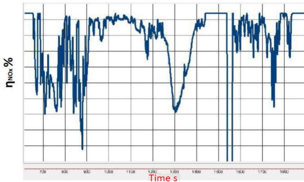
Figure 4.8:  $\eta_{NO_x}$  NRTC-transient cycle poisoned SCR
