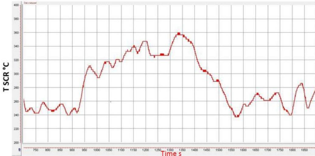
Figure 4.4: SCR inlet temperature
