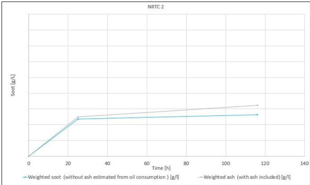
Figure 5.6: Soot accumulated on NRTC 2
