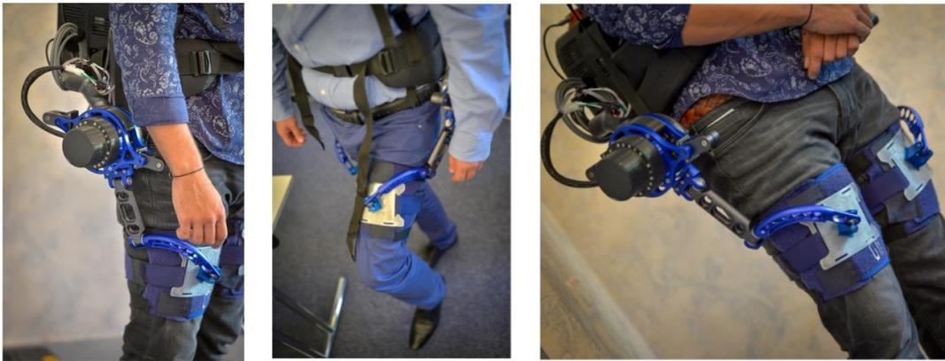
*Figura 11 Esoscheletro Active Trunk Robot-Mate [8]*
