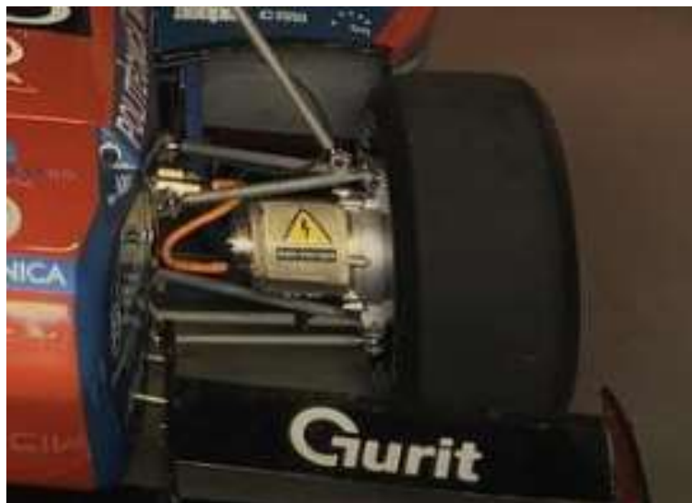
Figure 1: Hub Motor of a Formula SAE racing car
