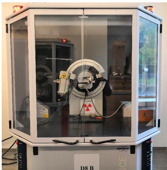
**Figure 3.6** D8 Advance X-Ray Diffractometer
