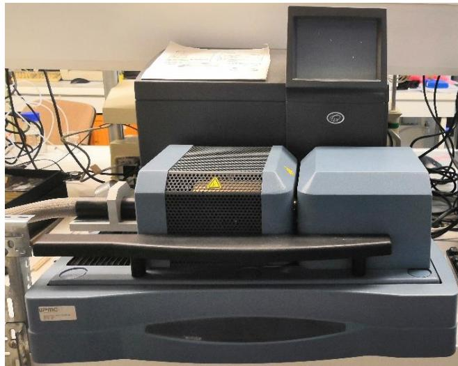
**Figure 3.7** SDT Q600 Thermogravimetric Analyzer
