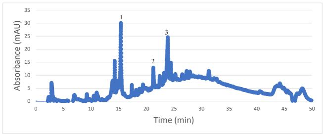
Figure 44 shows the corresponding chromatogram for wine less extraction at 100°C, using 60 % ethanol for 5 minutes and 2 operation cycles:
