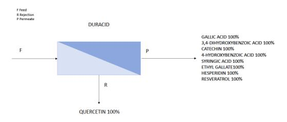
Figure 53 - Scheme of the membrane system performance for DURACID membrane and corresponding result
