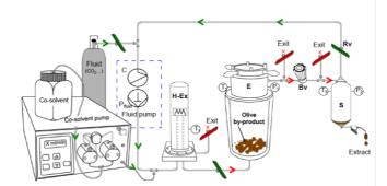
Figure 20 - Schematic lab-scale set-up of supercritical fluid extraction (Roselló-Soto et al. 2015)
