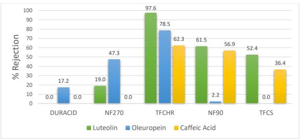
Figure 55 - Nanofiltration results for luteolin, oleuropein and caffeic acid (% rejection)
