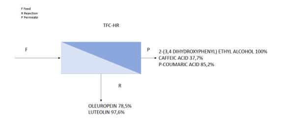
Figure 56 - Scheme of the TFC-HR membrane system performance and corresponding result
