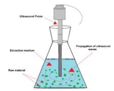
Figure 17 - Ultraosund system coupled to a probe (Medina-Torres et al. 2017)
