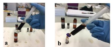
**Figure 32** - a) Filtration with a 0.45  $\mu$ m filter b) Filtration with a 0.22  $\mu$ m to proceed with HPLC analysis
