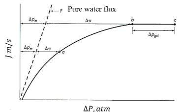
*Figure 23* – *Flux vs applied pressure*
