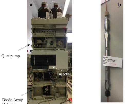
Detector Figure 37 - a) Chromatograph Agilent Series 1100, b) Chromatographic column
