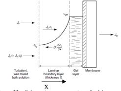
Figure 22 – Schematic representation of gel-layer model
