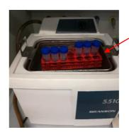
Distilled water ultrasonic bath with samples properly immersed
