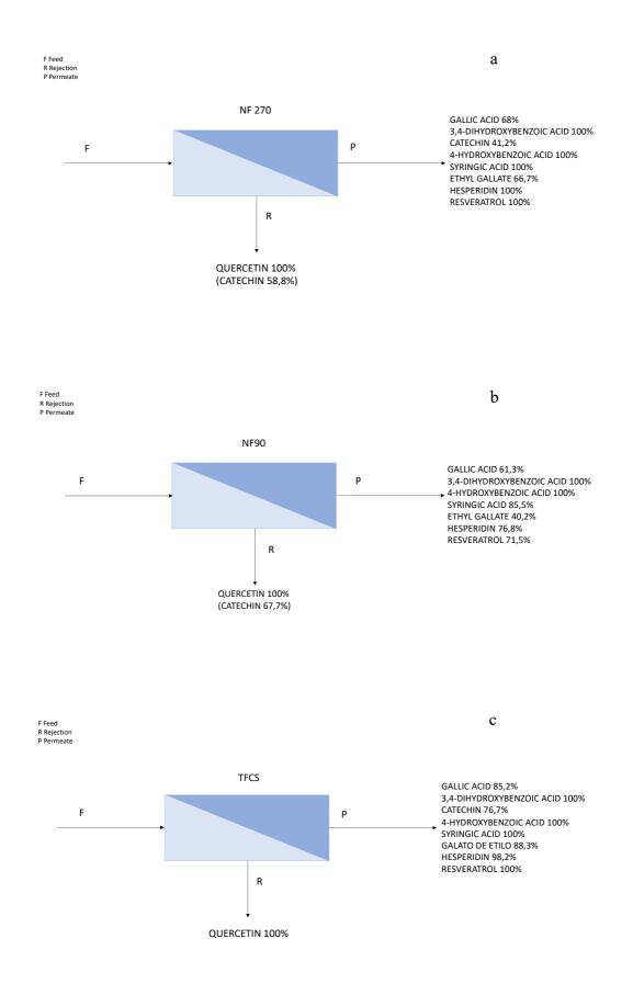
Figure 54 - Nanofiltration membranes schemes a) NF270, b) NF90, c) TFCS
