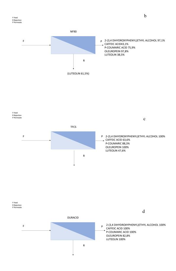
Figure 57 - Nanofiltration membranes schemes a) NF270, b) NF90, c) TFCS, d) DURACID
