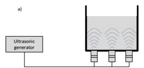
Figure 16 - Scheme of ultrasonic bath (Tiwari 2015)
