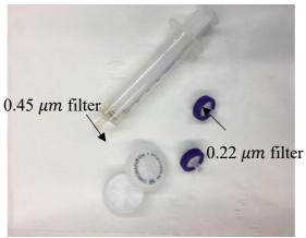
Figure 31 - Syringe and the two types of filters
