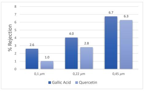
Figure 50 - Microfiltration results for gallic acid and quercetin
