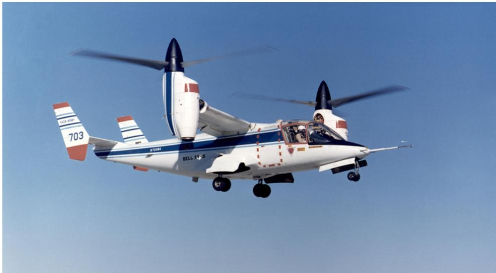
Figure 1.5: Bell/Boeing XV-15 prototype in helicopter mode
