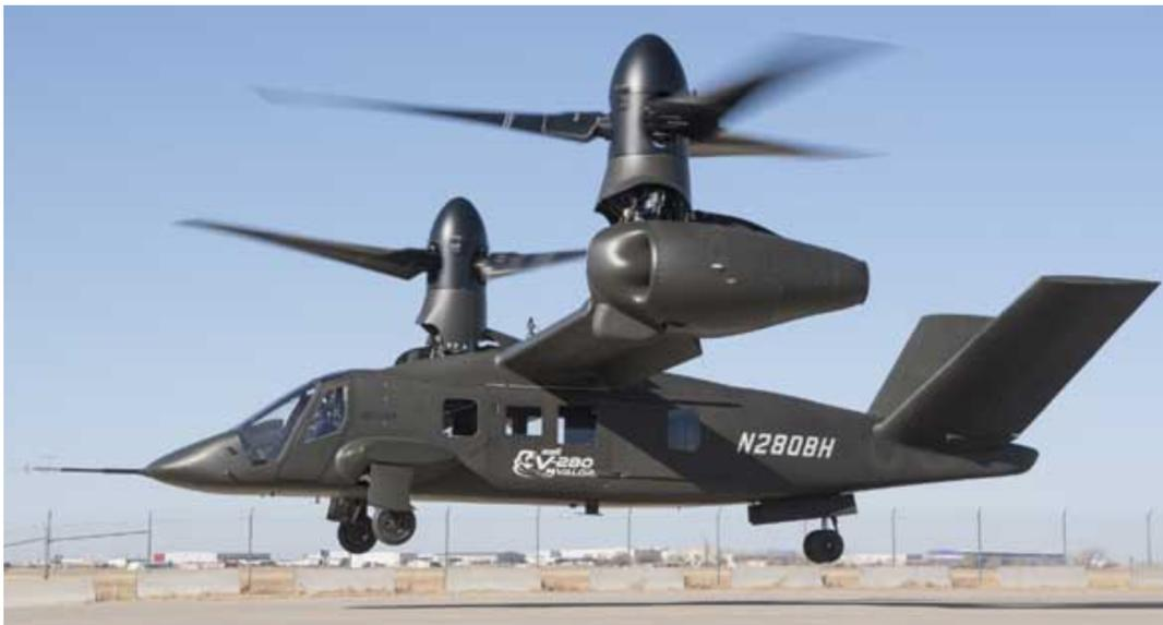
Figure 1.9: V-280 tilt-rotor
