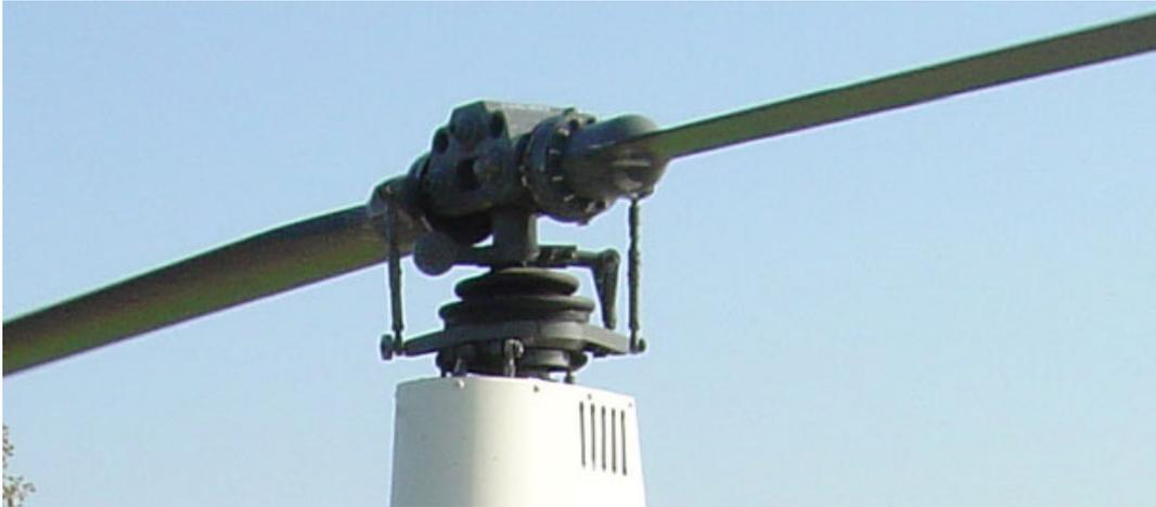
Figure 1.3: Robinson R-22 semi-rigid rotor
