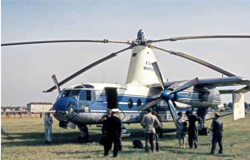
Figure 2: Fairey Rotodyne - Example of a VTOL rotorcraft<sup>10</sup>
