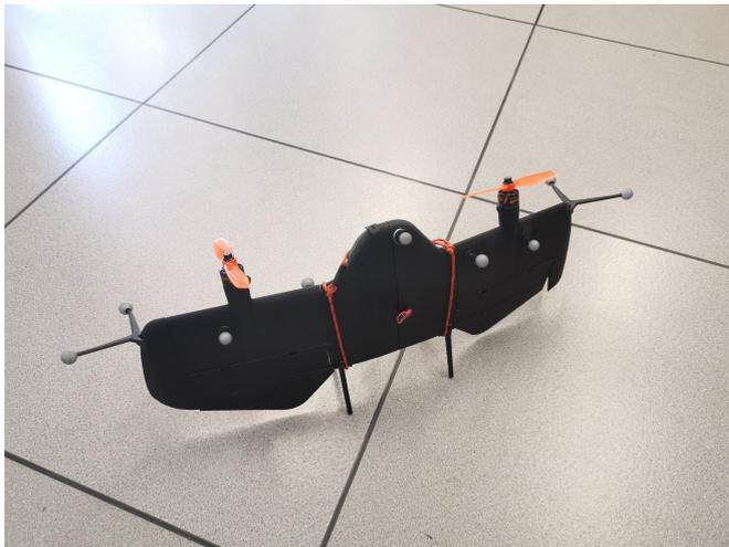
Figure 9: DarkO with the OptiTrack markers
