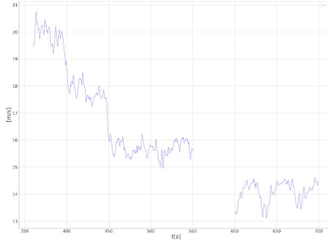
Figure 59: Airspeed for clockwise inner and outer circles
