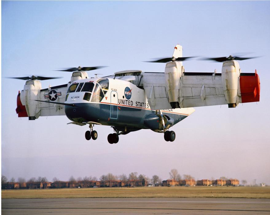
Figure 3: Ling-Temco-Vought XC-142A - Example of a VTOL powered-lift aircraft<sup>11</sup>
