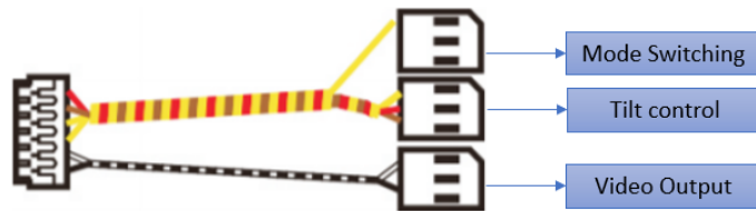
Figure 5.6: Tarot T4-3D wires connections
