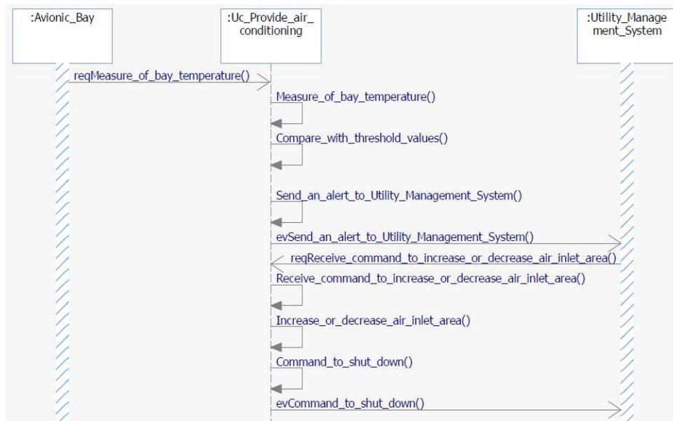
Figure 2.4: Provide Air Conditioning - Sequence Diagram 1
