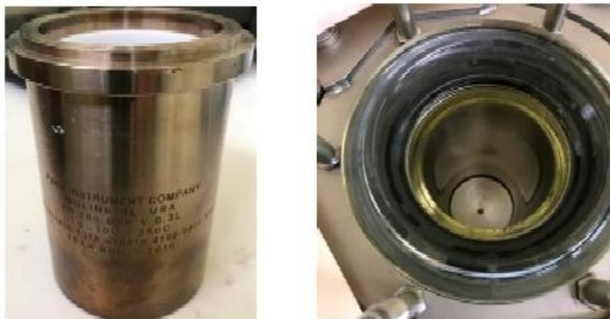
Figura 18- Autoclave massima pressione 200 bar e massima T 250°C (Fonte: Synthesis of Magnesium Carbonate via Carbonation under High Pressure in an Autoclave Srecko Stopic 1, Christian Dertmann et. al. 2018)
