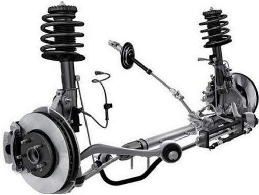
Figure 12. McPherson suspension.
