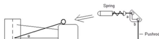
The first type of motion ratio has been explained in Chapter 6, but what we generally deal with is the second type. The motion ratio can be approximated as  $MR = a/b \cdot \sin(\theta)$ , where  $a$  and  $b$  are the rocker sides and  $\theta$  the push-rod inclination.
