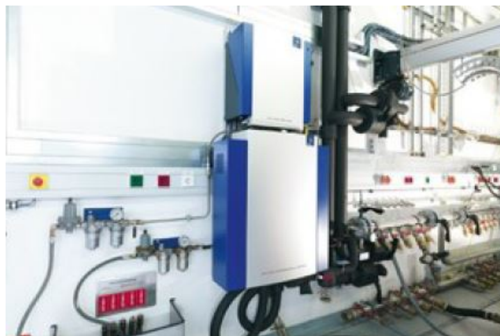
Figure 5.7: AVL KMA 4000 fuel consumption measuring system;
