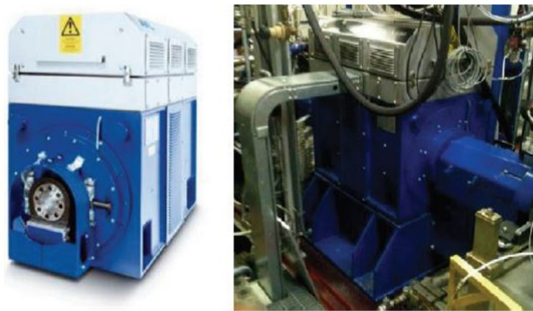
Figure 5.5: AVL transient dynamometer installed in ICEAL;
