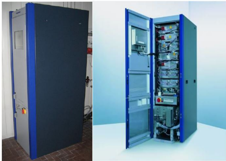
Figure 5.8: AVL AMA i60 emissions analyzer;
