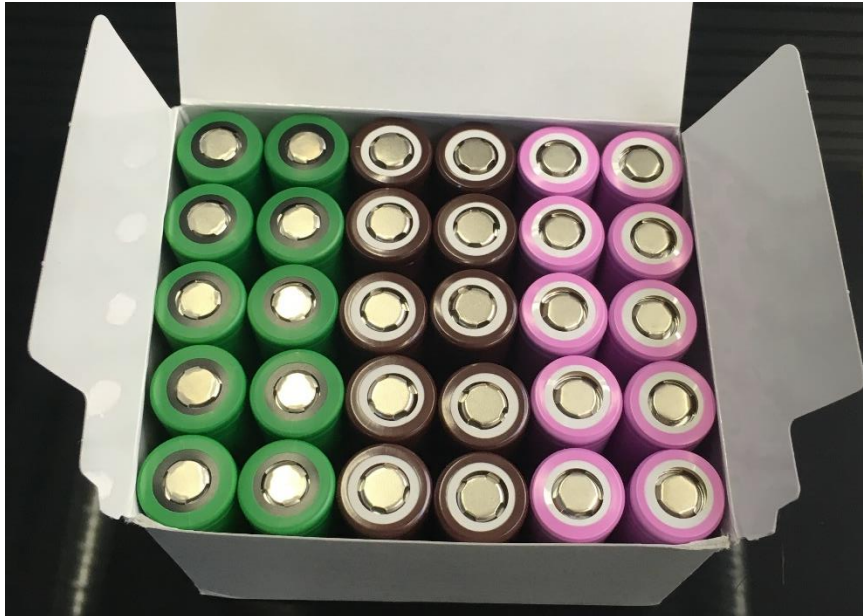
Figure 19: SONY VTC6, LG HG2 and SAMSUNG 30Q cells.
