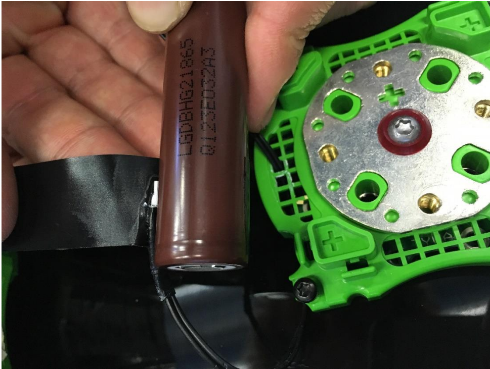
Figure 22: Positioning of the PT100 sensor to measure cell temperature during discharge.
