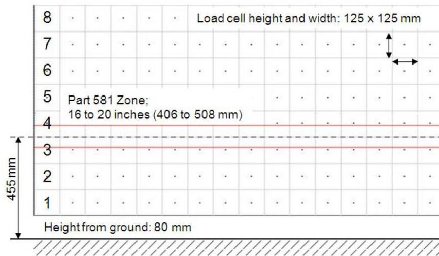
FIGURE 33 - Scheme of a LCW
