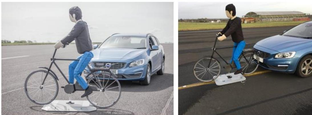
*FIGURE 13 - AEB test for cyclist*
