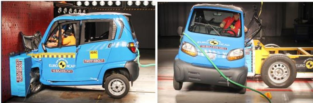
*FIGURE 12 - Quadricycle's test, frontal impact on left and side impact on right*
