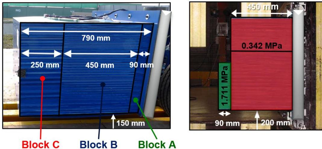
FIGURE 18 - Comparison between MPDB and ODB
