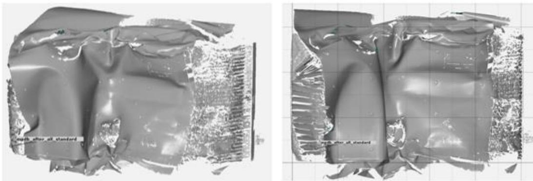
*FIGURE 63 - Barrier with almost complete cladding. Axonometric view on left ad frontal view on right*
