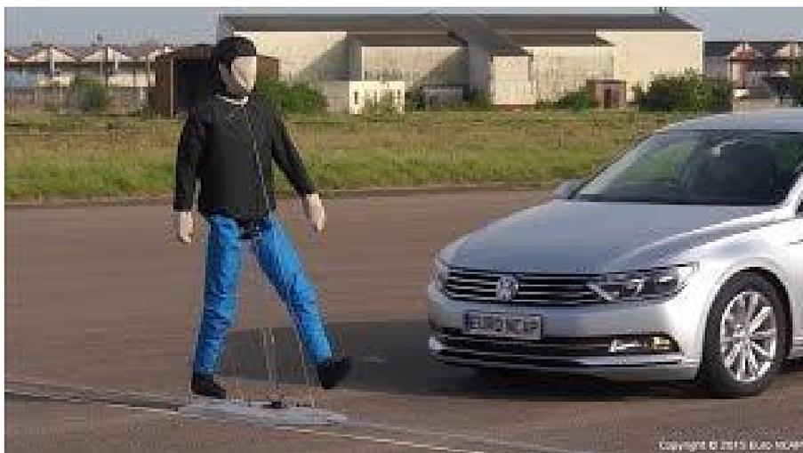
*FIGURE 11 - AEB test with a pedestrian*
