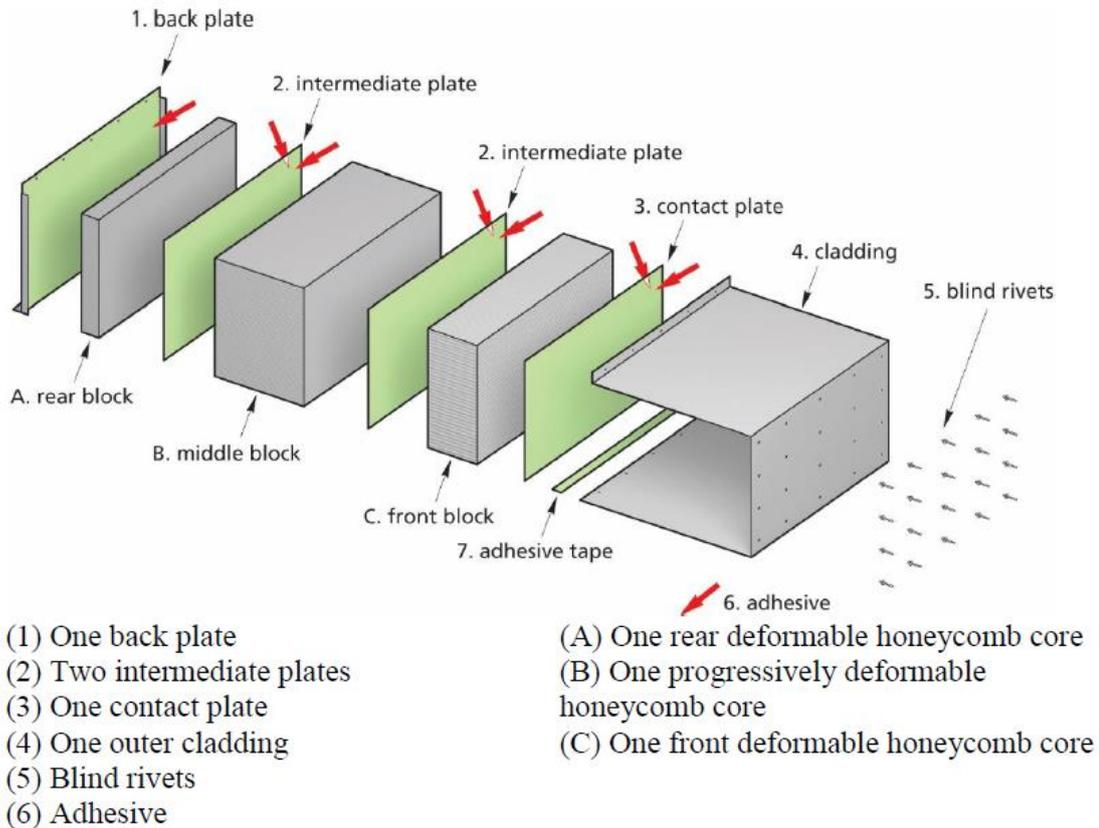
FIGURE 46 - Exploded view of the impactor
