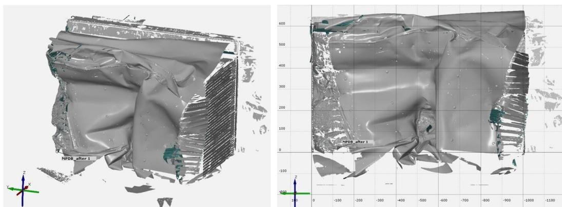
*FIGURE 108 - Different view of scansion of crashed barrier*
