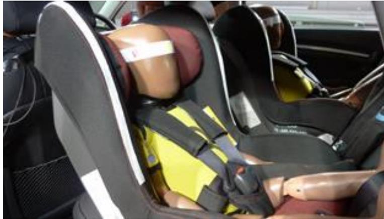
*FIGURE 4 - Child dummy in Child Restraint System*
