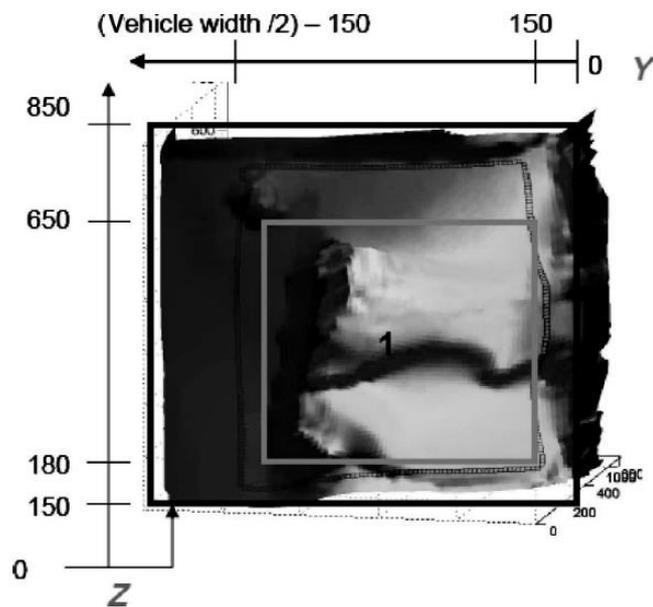
FIGURE 29 - Front view of the barrier with dimensions
