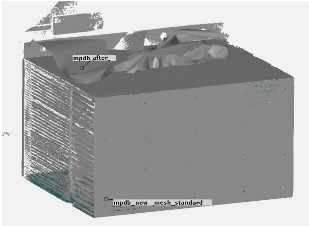
FIGURE 66 - New and after crash scansion aligned
