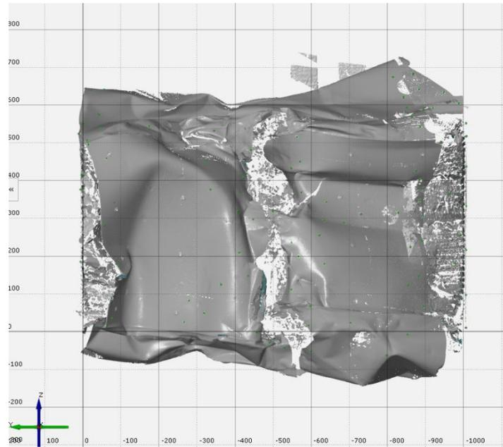
FIGURE 102 - Scansion of the barrier after the test
