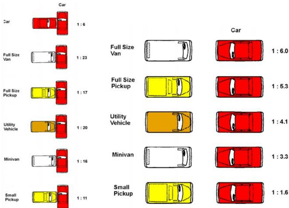
FIGURE 20 - Side impact and frontal impact with the relative AM
