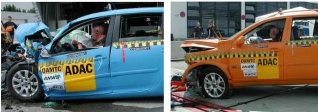
FIGURE 22 - Comparison of small vehicle (on left) and heavier vehicle (on right) after a frontal crash
