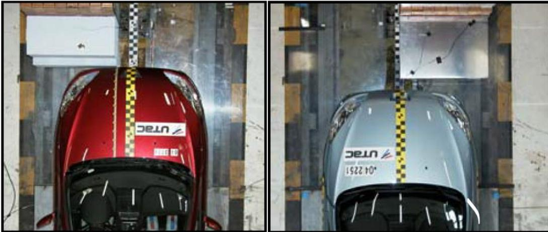
*FIGURE 15 - ODB on left and MPDB on right*
