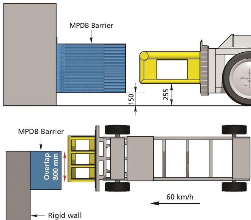
FIGURE 45 - Impactor and alignment
