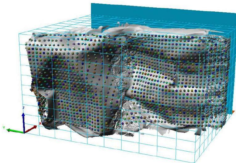
FIGURE 52 - Projection of grid in the deformed barrier mesh
