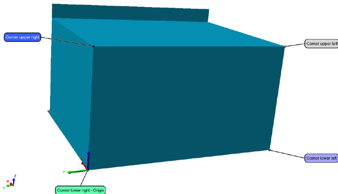
FIGURE 49 – Barrier reference system
