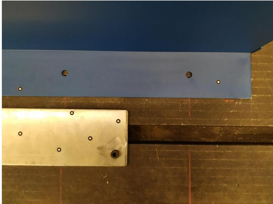
*FIGURE 84 - Holes of the barrier that does not coincide with the hole of the station in the upper part*
