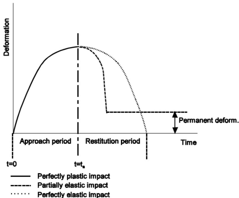
FIGURE 25 - Different behaviour of the body deformation over time
