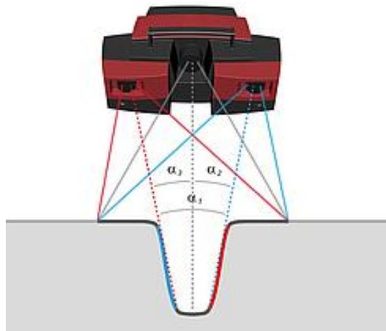
FIGURE 57 -Triple Scan technology
