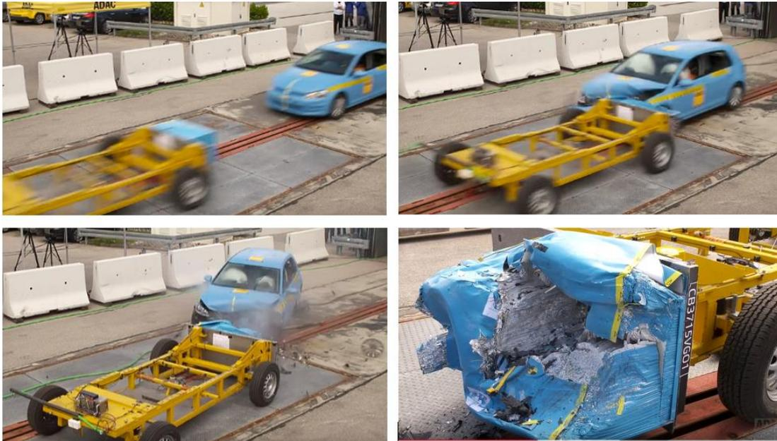
*FIGURE 40 – MPDB frontal impact test sequence*
