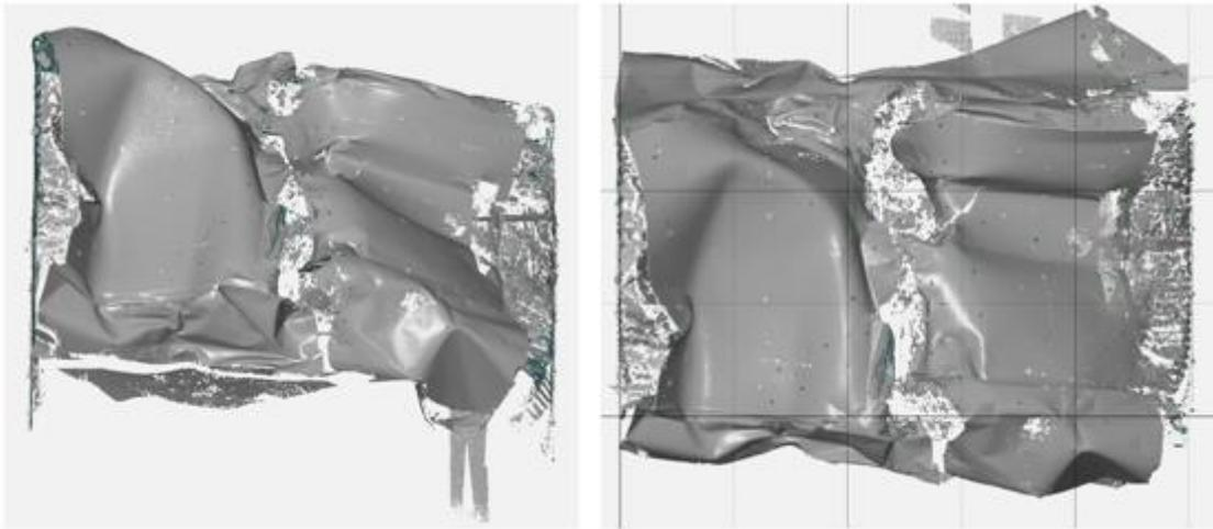
*FIGURE 62 - Barrier with broken cladding. Axonometric view on left ad frontal view on right*
