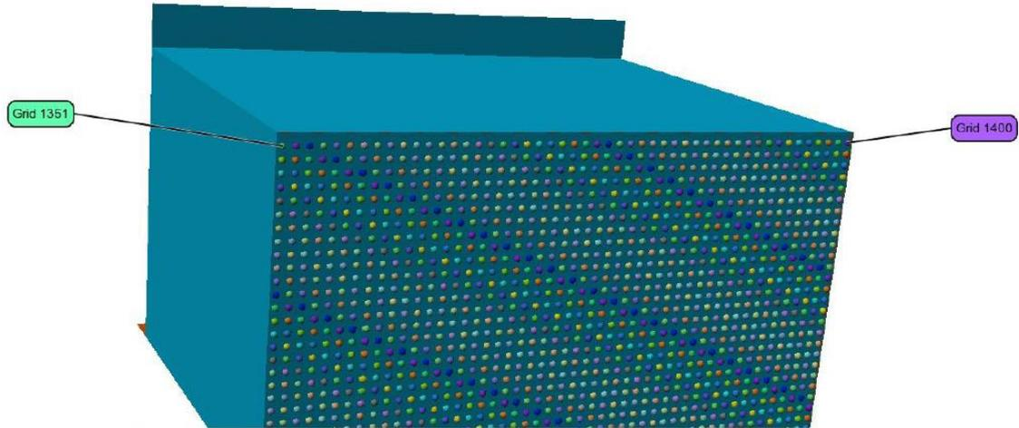
FIGURE 51 - Grid of points centred in undeformed barrier
