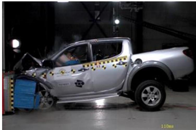
*FIGURE 5 - Frontal impact of a pick-up*
