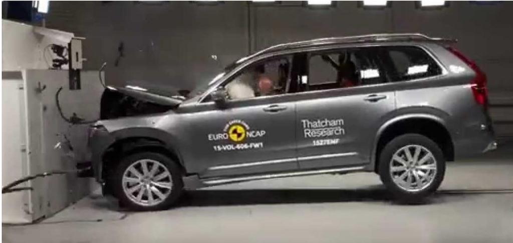
*FIGURE 10 - Full overlap test with rigid barrier*
