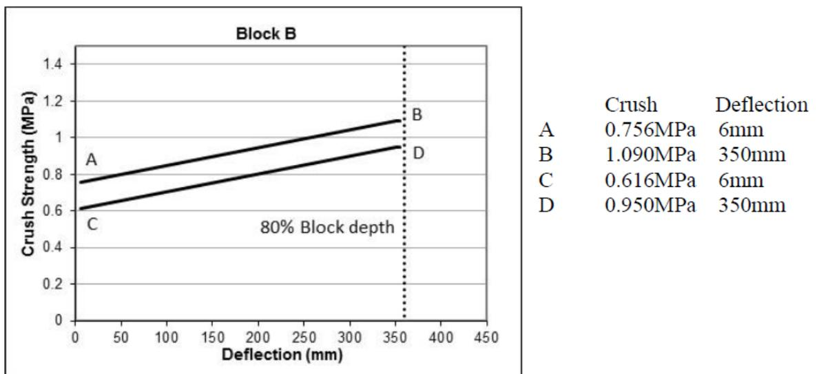
FIGURE 43 - Block B crush strength characteristic
