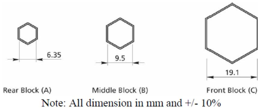
FIGURE 48 - Honeycomb cell dimensions
