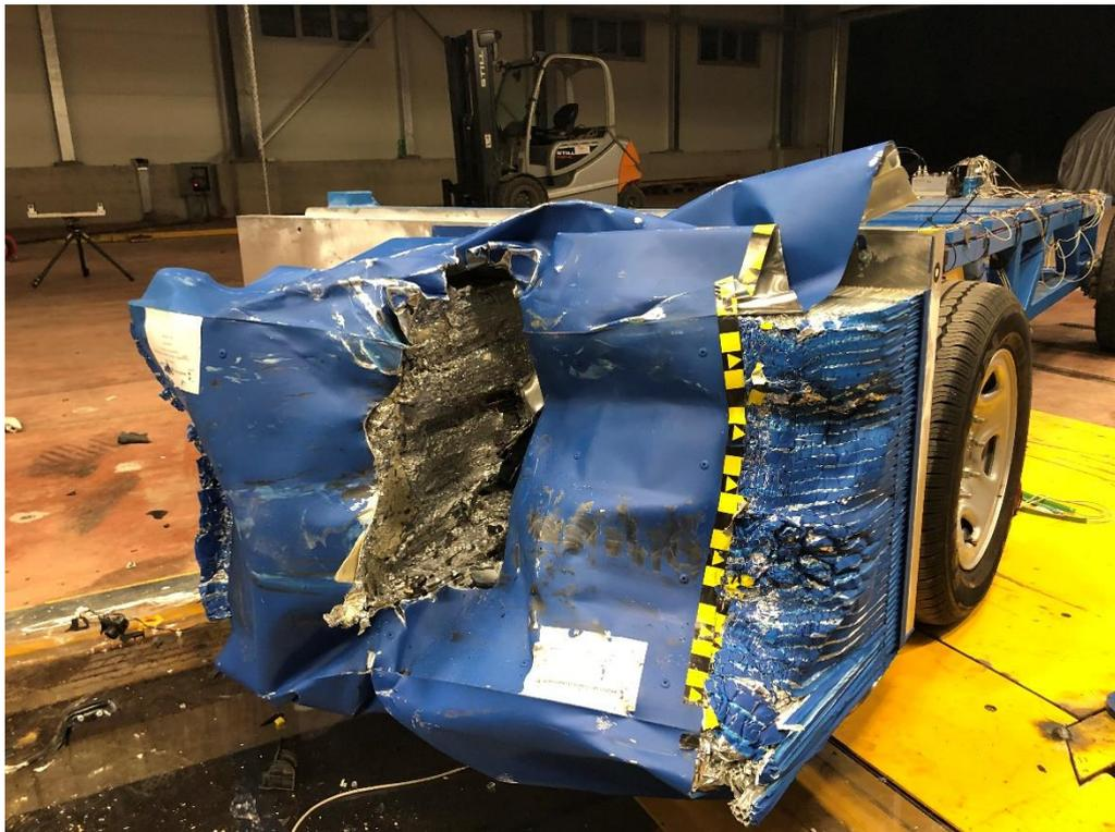
*FIGURE 93 - Crashed barrier on the trolley*
