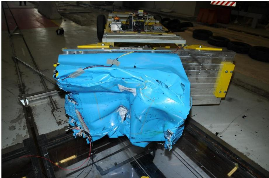
*FIGURE 107 - Crashed barrier on the trolley*
