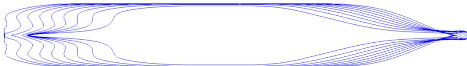
Figure 2.4: z-sections of the undeformed hull.
