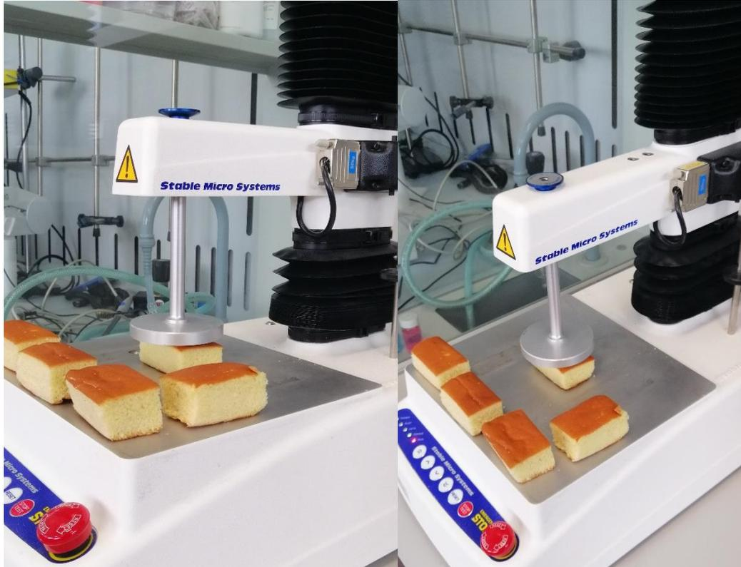
Figure 3 Instrument for TPA
