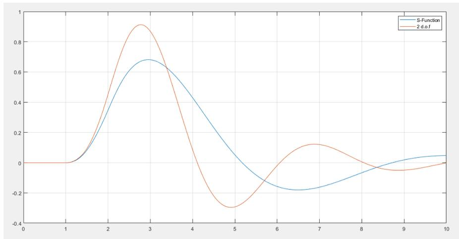
Figure 5-10 Lateral displacement of vehicle using 2 d.o.f model or CarSim S-Function
