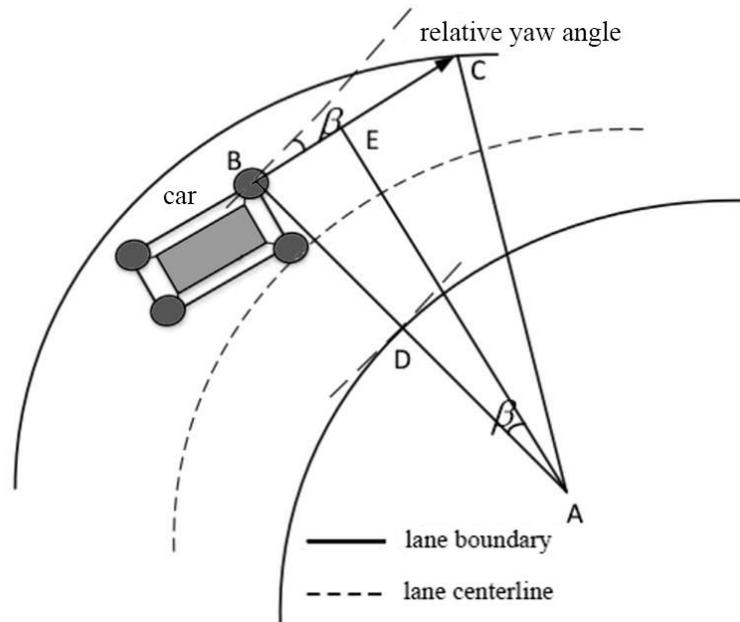
Figure 3-3 The vehicle on the curved road deviates to the left with a straight trajectory
