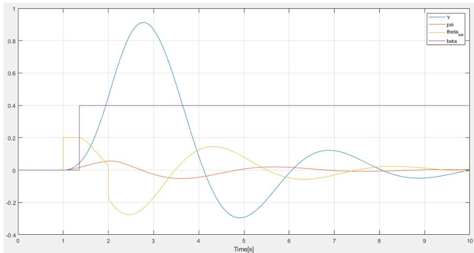
Figure 5-7 Lateral displacement, yaw angle, steering wheel angle, LKA intervention conditions variation
