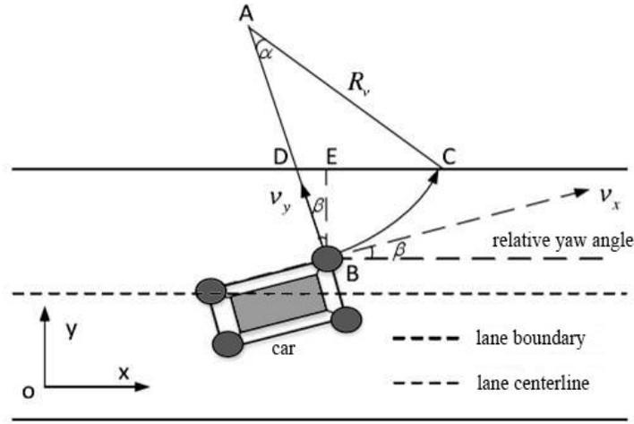
Figure 3.1 The vehicle on the straight road deviates to the left with a curved trajectory
