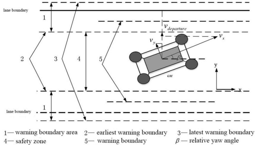
Figure 3-4 The warning boundary and its relative positional with the lane boundary.
