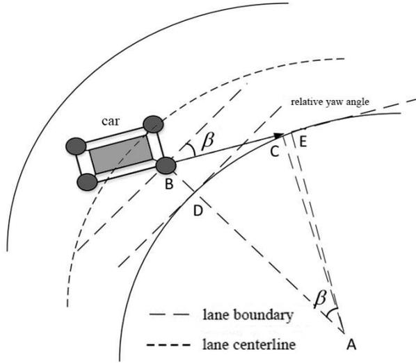
Figure 3-2 The vehicle on the curved road deviates to the right with a straight trajectory
