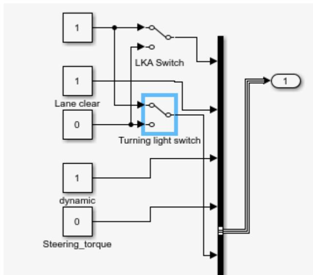
Figure 4-12 Virtual switches of turning light switch
