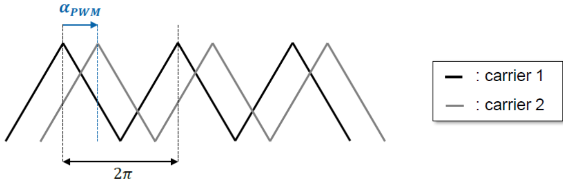
Fig. 49: Shifted carriers for 3-levels PWM control routine.
