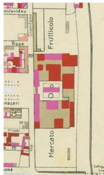
Figure 1.8 The damages caused by WWII. In dark red are shown structural collapses, while the critical damages are noted in light magenta. (Historical Archives)
