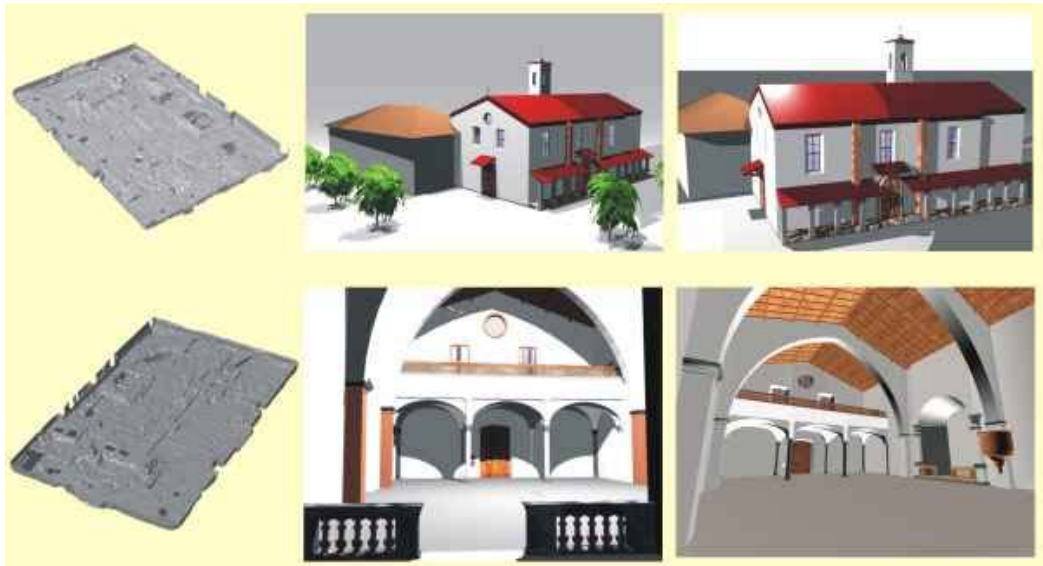
Reproduction of the excavated surface obtained through the elaboration of the laser scans; outside and inside 3D representation of the church
