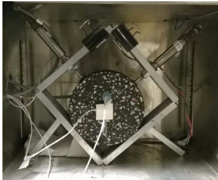
Figure 3.14: Ohio CTE device with AC sample equipped with resistance temperature
