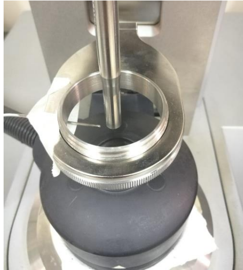
Figure 5.6: monitoring the air temperature near the measuring system with a thermocouple
