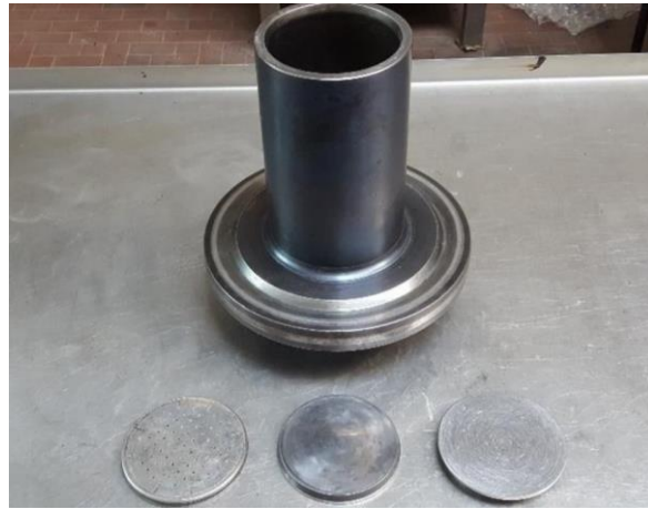
Figure 6.2: mould used for the gyratory shear compactor
