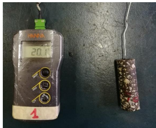
Figure 5.4: Asphalt concrete specimen equipped with type k thermocouple (right side) and datalogger (left side)
