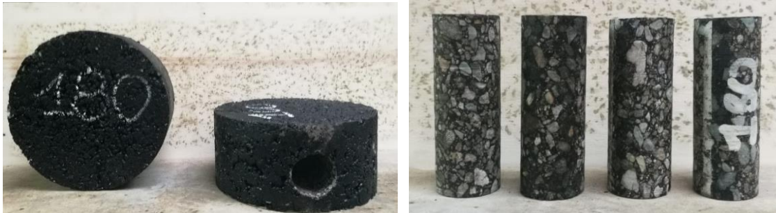
Figure 6.4: Compacted sample (left), 80 mm sample cored and sawed (right)
