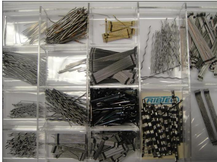
Figure 3: Different types of steel fibres [2]
