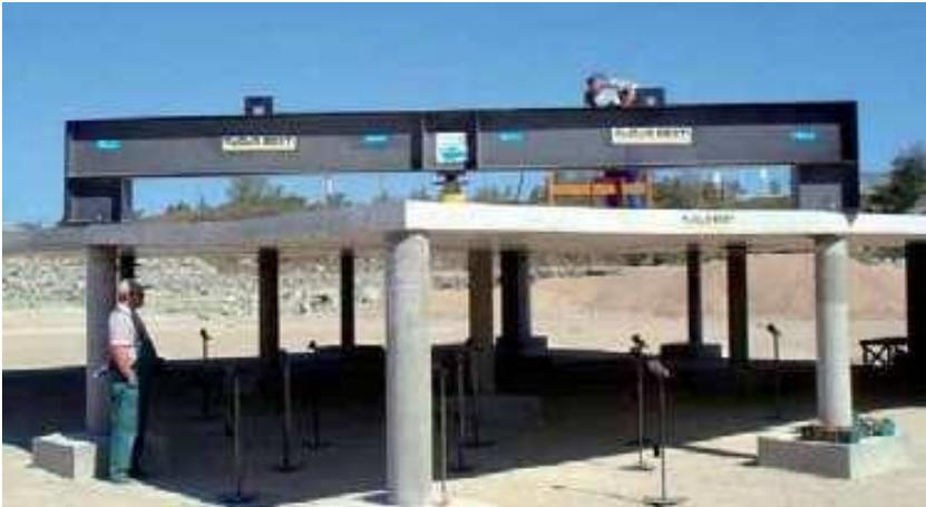
Figure 24: Full scale test in Tallinn with test rig and deflection gauges to measure the deformation of the slab under the loads in the uls. [10]
