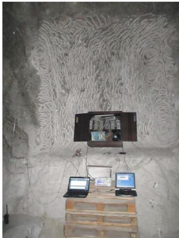
Fig. 2. 3: Experimental set-up of the monitoring station
