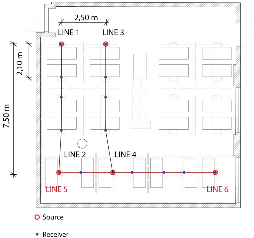
Fig.2: Plan of OP OFFICE 1, condition C0\_at (scale 1:100) with source and receiver positions.
