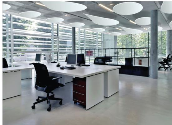
*Fig. 11: Examples of application of Cloudsorba suspended acoustic panels..*
