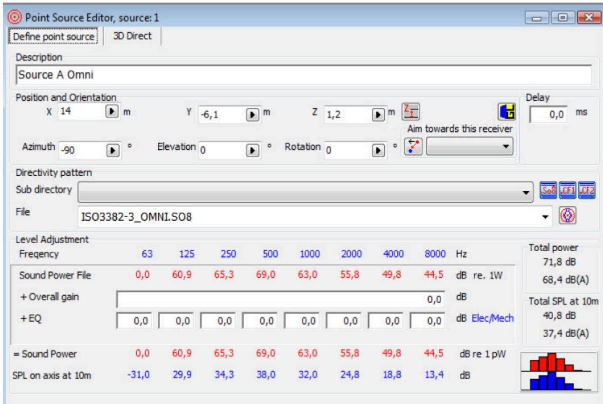
Fig. 4: The source definition menu in Odeon; the source with the name ISO 3382-3 OMNI.SO8 has the spectrum and sound power of normal speech as specified in the standard. The A-weighted sound power level is 68,4 dB(A).
