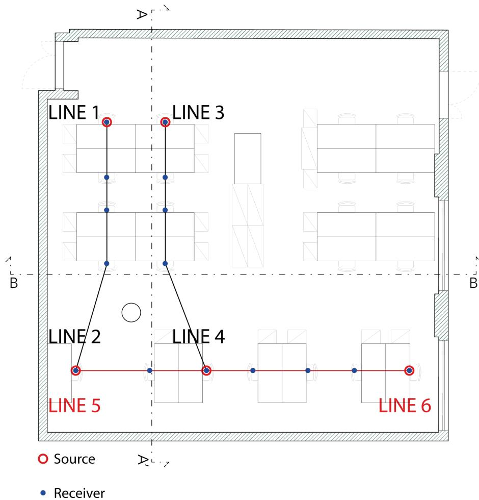
Fig. 1: Plan of OP OFFICE 1 (scale 1:100) with source and receiver positions. Four measurement lines are used, each associated with a point source.
