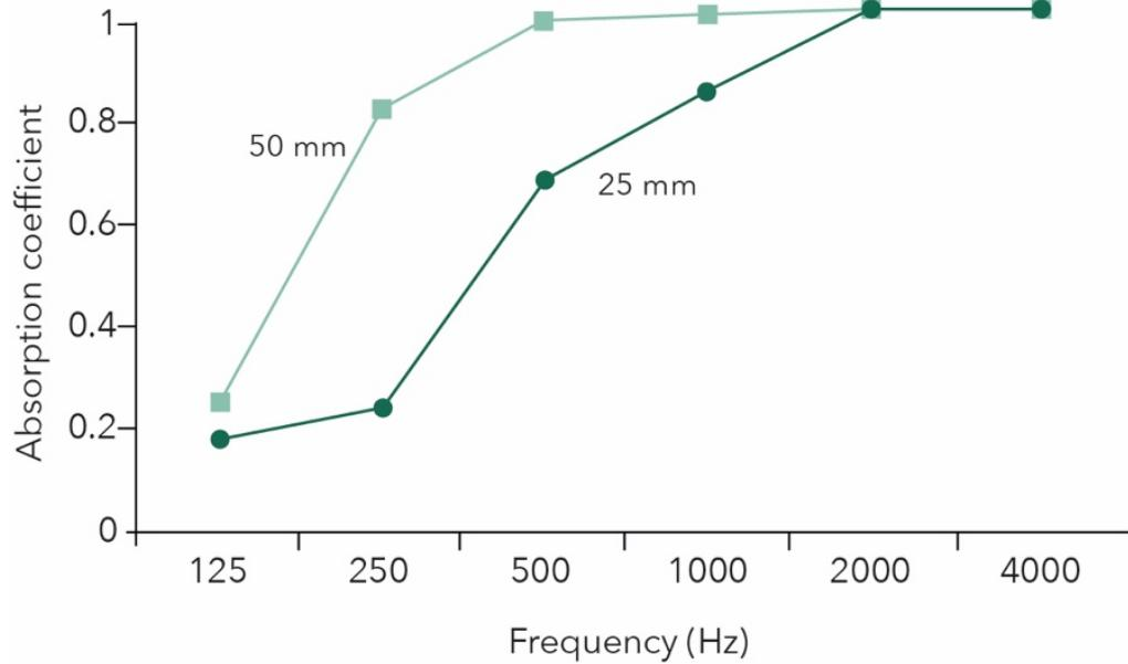
Fig. 7: Random incidence absorption coefficient for mineral wool of two different thickness on a rigid backing.[8]
