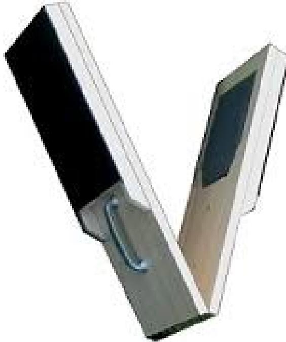
*Fig. 11: 2009 version of the clapper used in acoustic measurements.*
