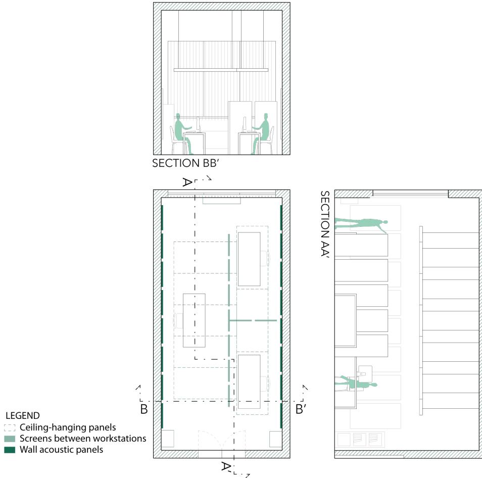
Fig. 4: Plan and sections of acoustic project of SH OFFICE 2 – scale 1:100
