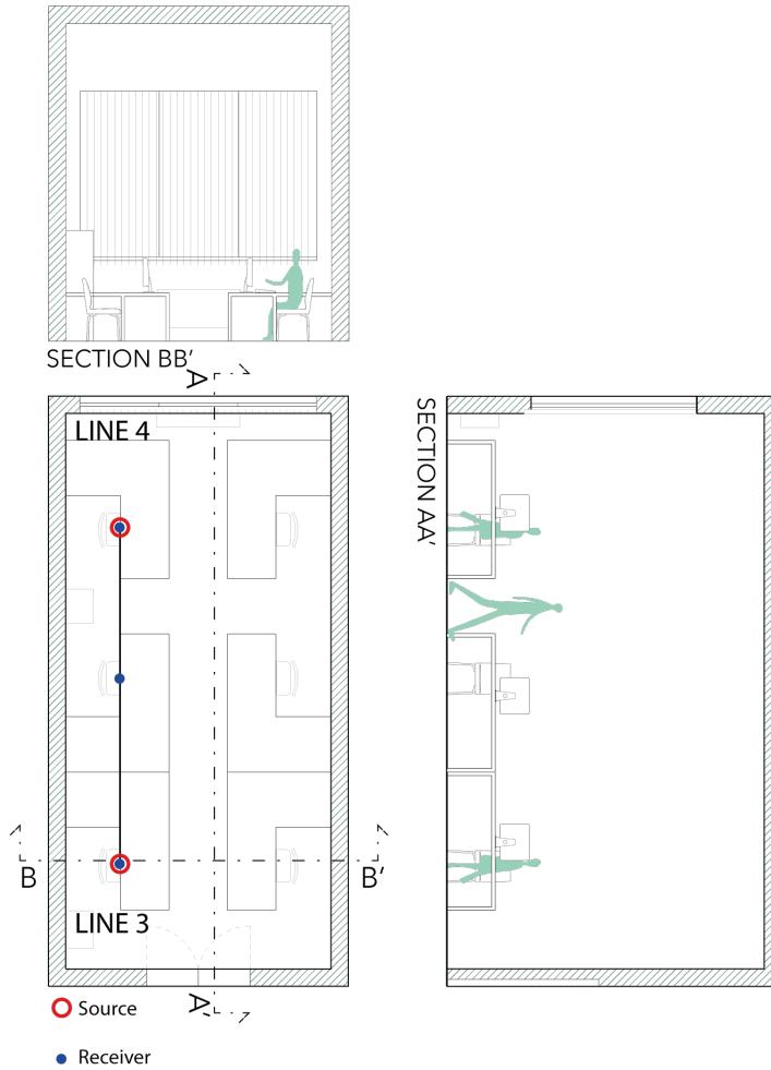
Fig.3: Plan and sections of SH OFFICE 2 (scale 1:100) with source and receiver positions. Four measurement lines are used, each associated with a point source.
