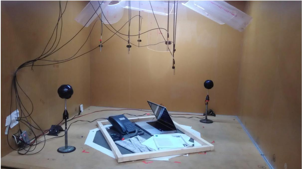
*Fig. 2: Experiment of the measurement of absorption coefficients of desks of SH OFFICE 2.*
