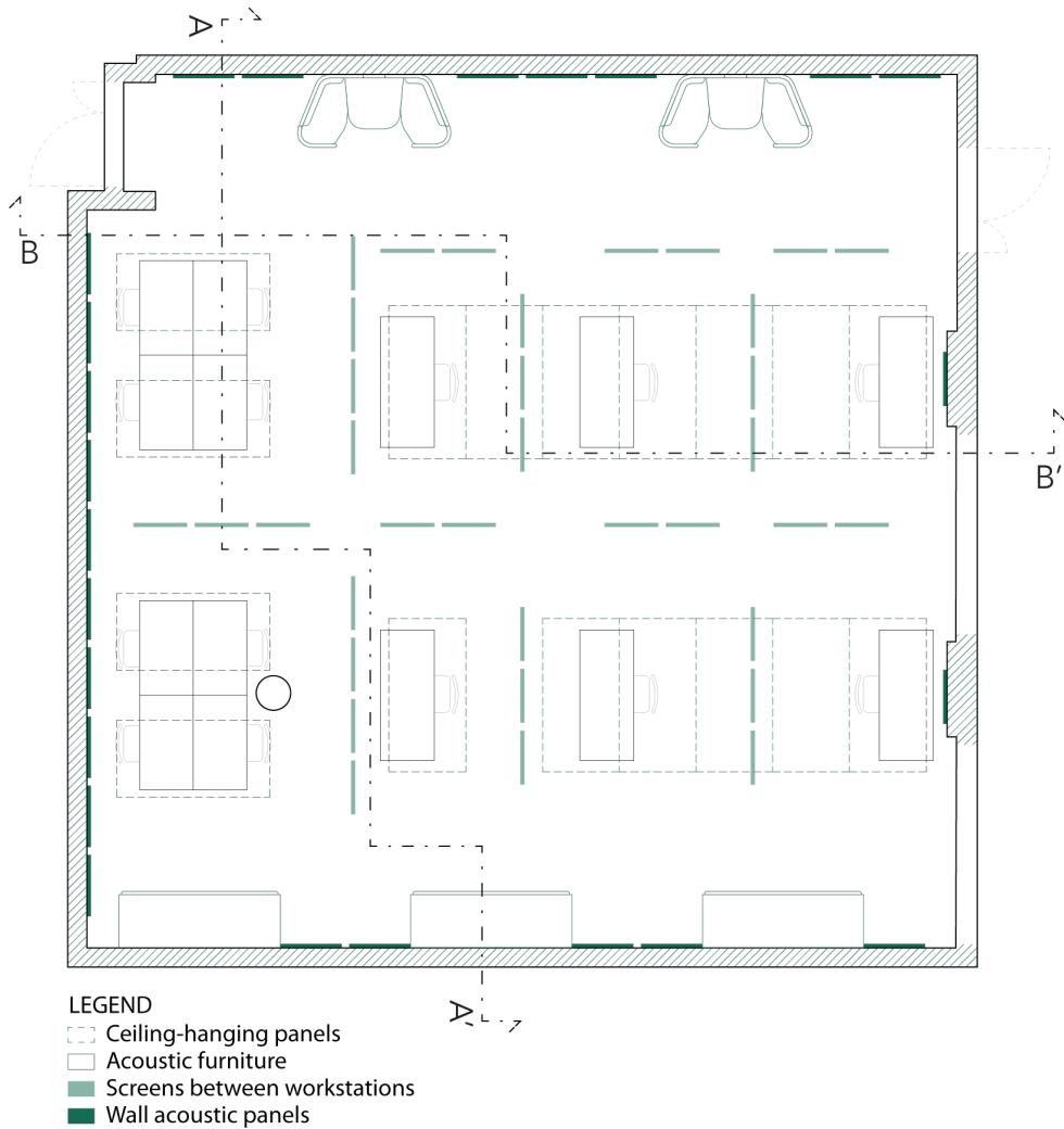
Fig. 12: Plan of acoustic project of OP OFFICE 1 - scale 1:100
