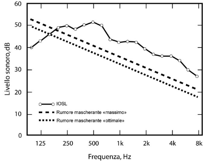
Fig. 1: curve of sound masking level.
