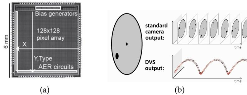
Figure 2.6: (a) 128x128 pixel array of a 4M2P DVS (b) Rotating disc stimulus output comparison between legacy vision sensors and DVS.
