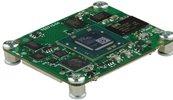
Figure 4.2. The Trenz Electronic SoC
