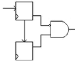
Figure 4.10. Circuit for overflow detection
