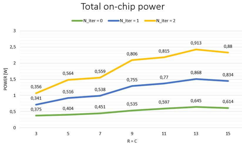
Figure 6.24. Total power consumption for different iterations
