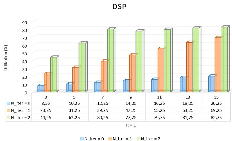
Figure 6.21. Number of used DSPs for different iterations
