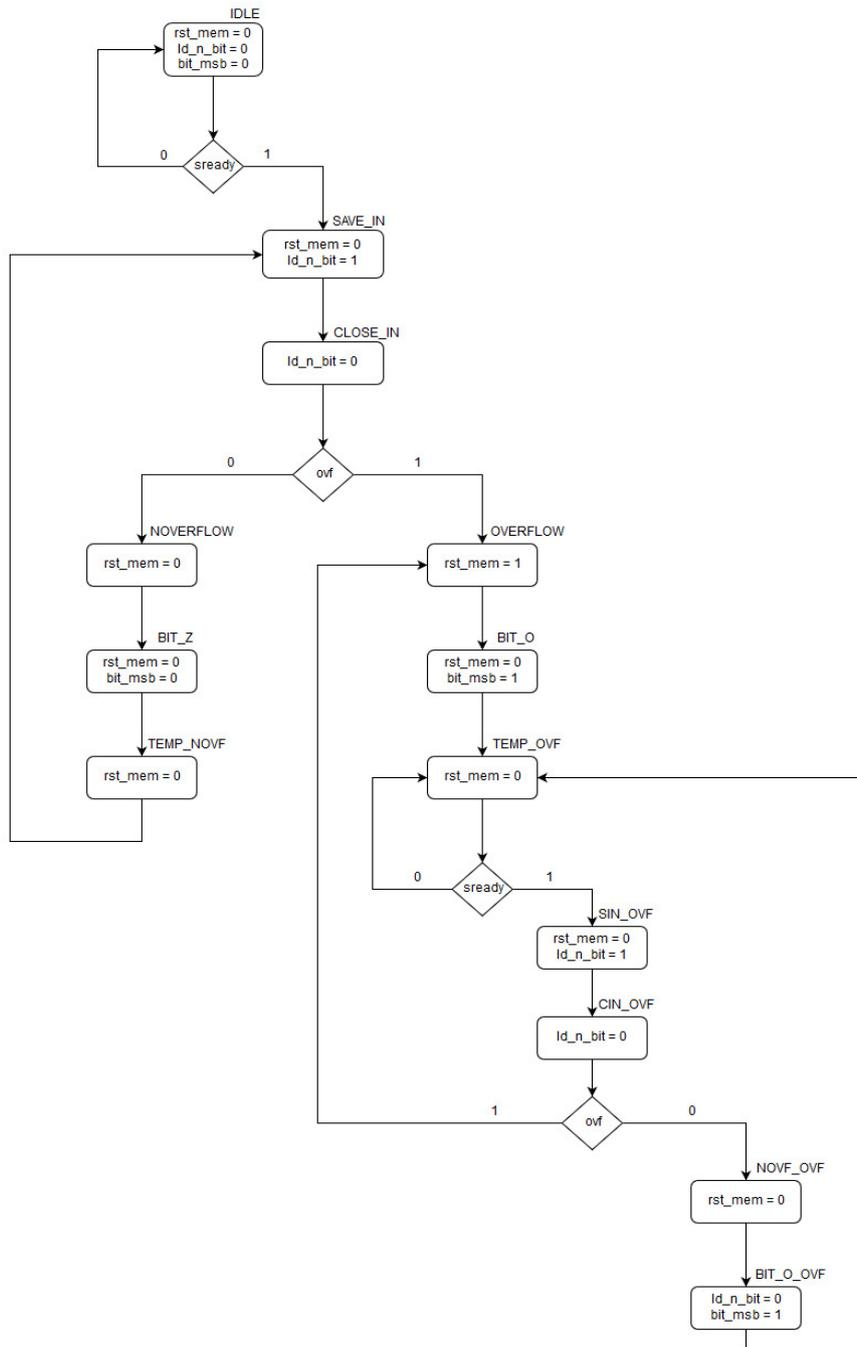
Figure 5.3. Control chart of the state machine
