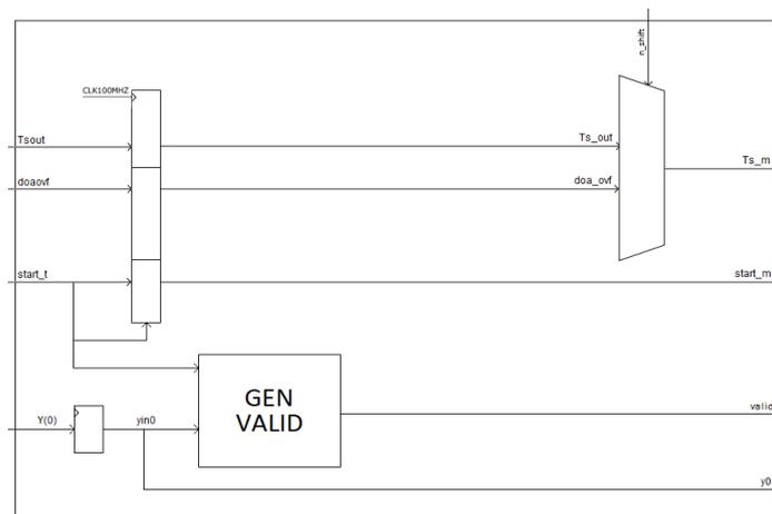
Figure 5.4. Valid generator and shifter blocks
