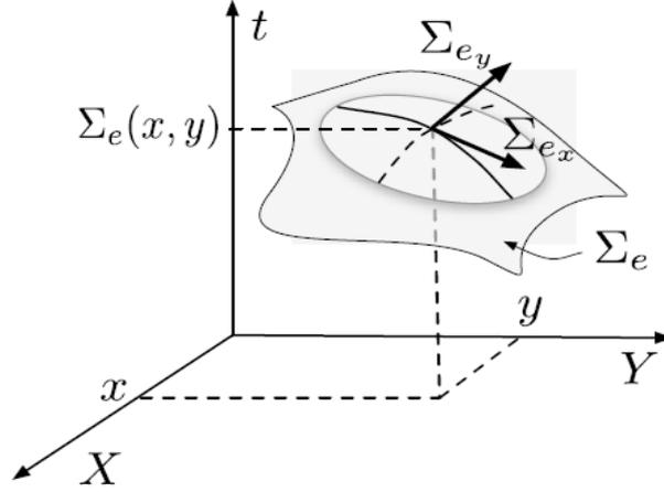
Figure 2.1. Surface of active events for optical flow computation
