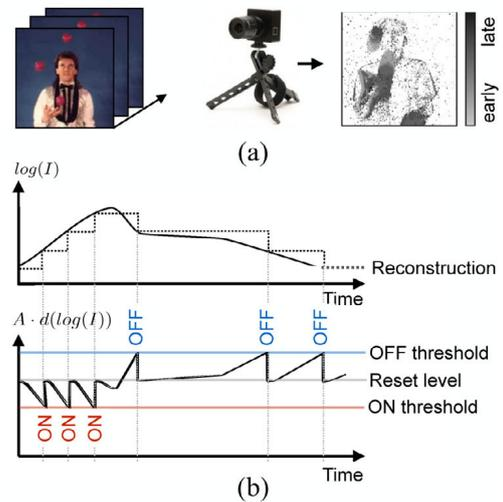
Figure 1.12. The DVS working principle
