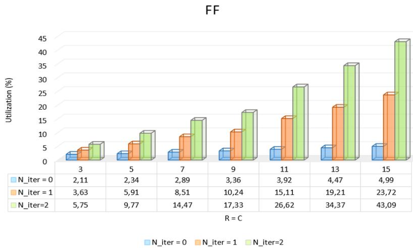
Figure 6.23. Number of used FFs for different iterations
