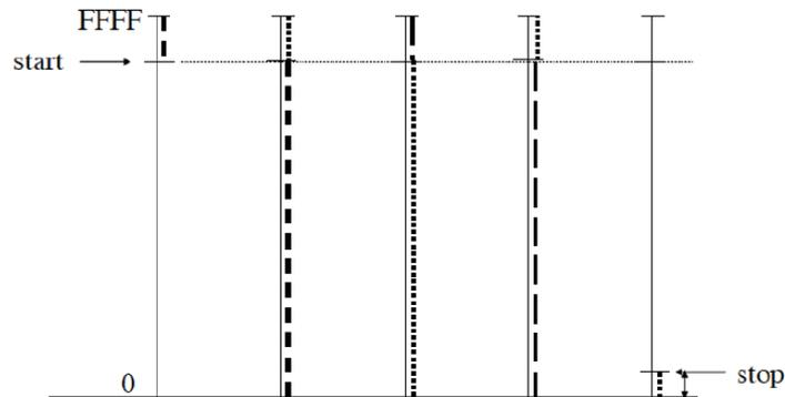
Figure 3.3. Multiple Overflows in a counter
