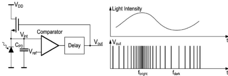
Figure 1.9. The ATIS structure and its behaviour
