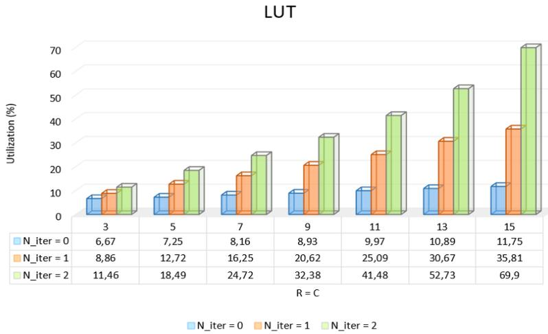
Figure 6.22. Number of used LUTs for different iterations
