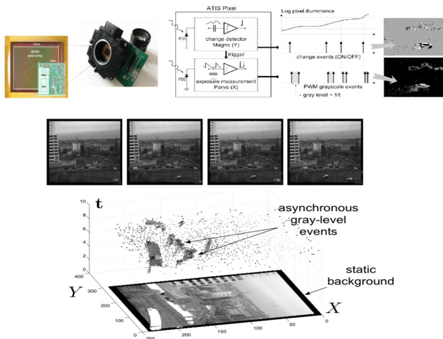
Figure 1.10. ATIS working principle
