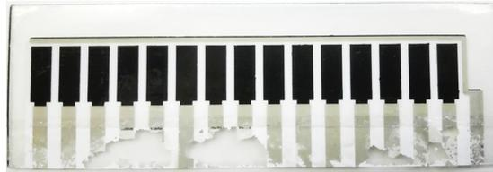
Figure 6.5: Delaminated display.
