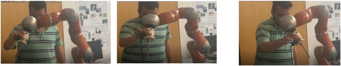
**Figure 4.1** Hands-on motion of robot for data collection of orientation angles and force sensor measurement in free motion.
