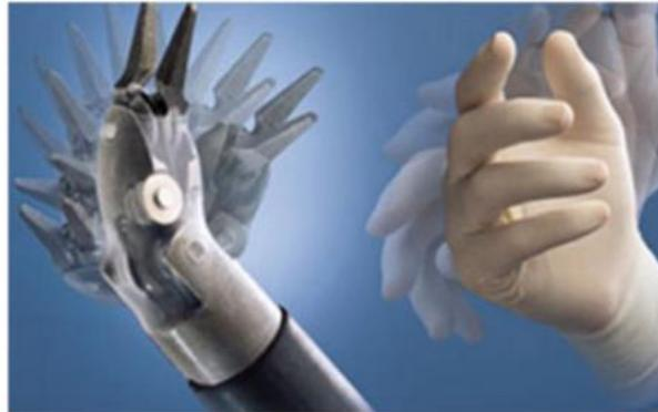
**Figure 1. 4** Comparison of the dexterity of the EndoWrist (left) with that of human hand (right). Reprinted from (Ramos, de Souza Bastos, & Kim, Obesity and diabetes: New surgical and nonsurgical approaches, 2015).
