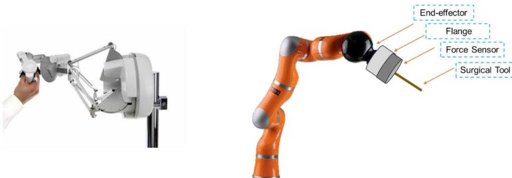
**Figure 1.5** The human operator sends commands to slave robot (right) by controlling the master device (left). Surgical Tool attached to distal part of the force sensor, placed between flange and surgical tool providing the interaction forces between surgical tool and tissue.
