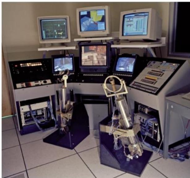
**Figure 2.3** JPL Advanced Teleoperation (ATOP) system control station. Reprinted from (Niemeyer, Preusche, & Hirzinger, 2008).
