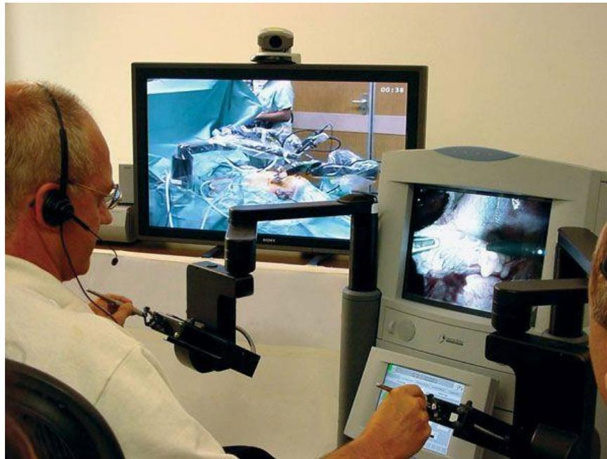
**Figure 2.7** Surgeon operating the robotic console in New York to remove the gall bladder of a patient in France. Reprinted from (Marescaux, et al., 2001).
