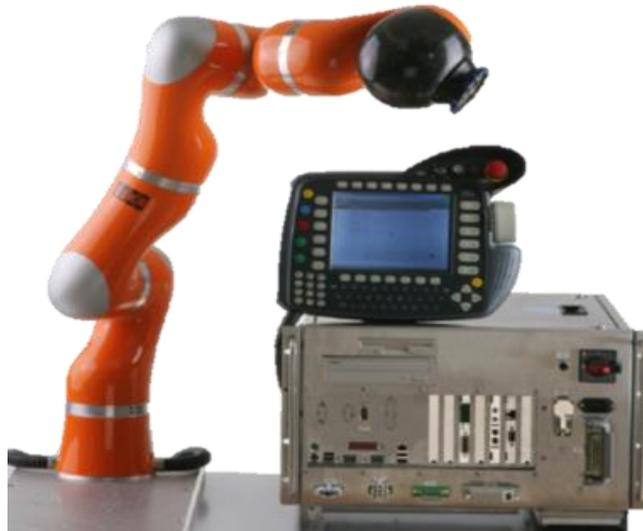
**Figure 3.3.** KUKA Lightweight Robot 4+ (LWR4+) with KUKA Robot Controller (KRC) and KUKA Teach Pendant. Adapted from (Penza, 2013).
