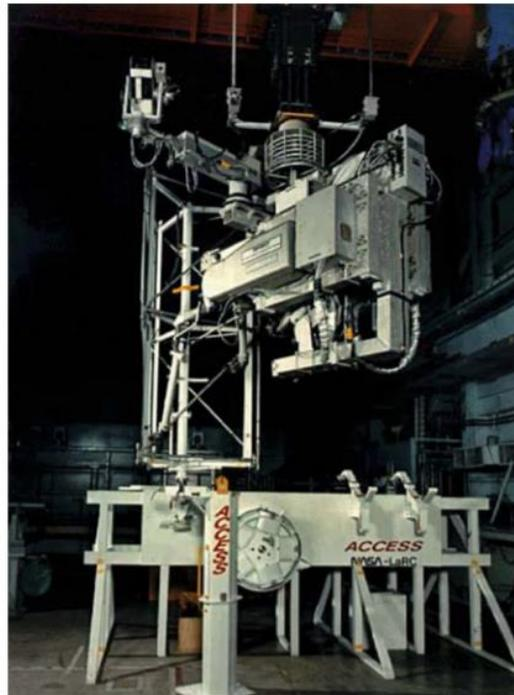
**Figure 2.2** Telerobotic system CRL Model M2 developed by Oak Ridge National Laboratory and used by NASA in deep space assembly applications. Reprinted from (Trevelyan, Kang, & Hamel, 2008).
