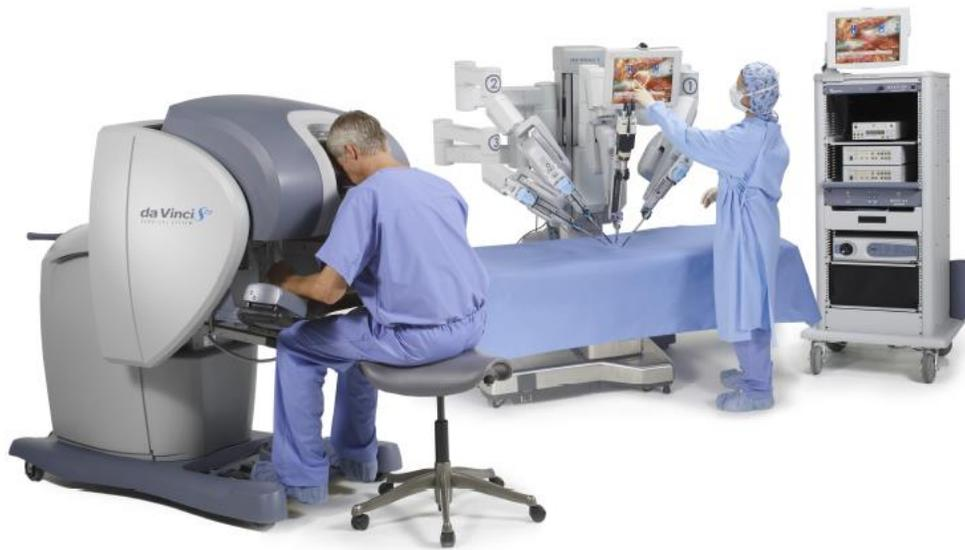
**Figure 1. 2** Da Vinci Surgical System (SI version). Reprinted from (Uzunoglu, 2012).
