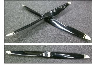
(c) Off-the-shelf rotor used for recirculation test. ©Smigła Biela
