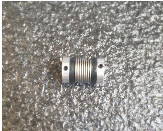
Figure 2.27: R+W MK1 miniature bellow coupling
