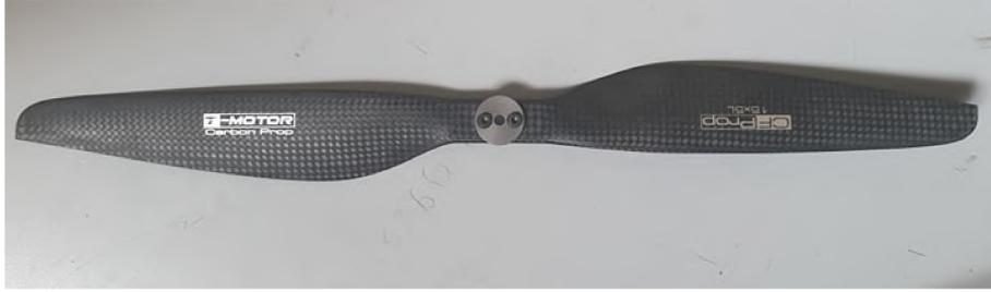
Figure 2.31: T-motor 15"x5" L propeller and fixing cover
