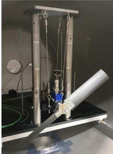
Figure 1.10: Swing test bench in TAS-I PHASE vacuum chamber
