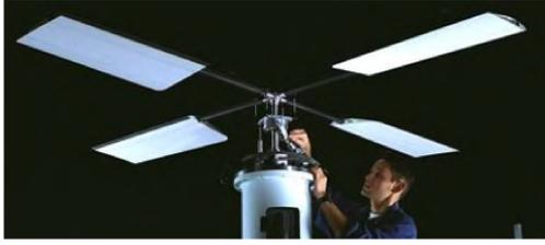
(a) Isolated rotor testing blade. [9]
