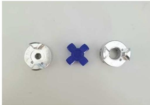
Figure 2.9: Jaw coupling elements
