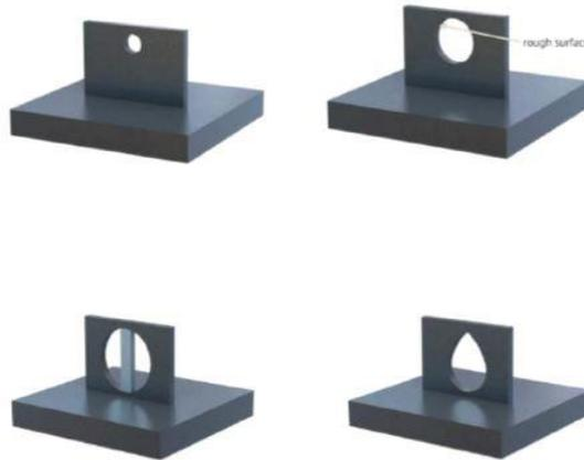
*Figura 37 - Fori in Additive Manufacturing*
