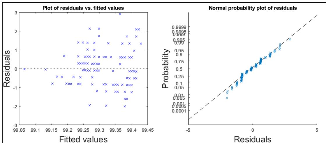
Figure B1.10: Plot of studentized residuals versus fitted values (on the left) and probability plot (on the right) derived from the simple linear regression model between train speed and mean wheel loads detected for the **right** wheel of the first axle of locomotive **917400014341** between March 18<sup>th</sup> 2018 and January 29<sup>th</sup> 2019 at **Skorped** detector station.
