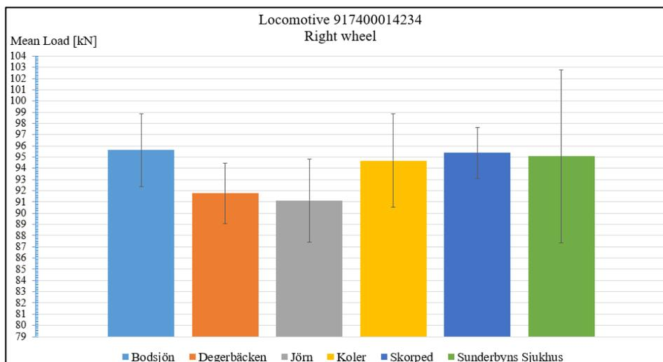
Figure 3.8: 2D-Bar plot showing the average value of mean loads registered for the **right** wheel of the first axle of locomotive **917400014234** at each detector station in the period of time **May 1<sup>st</sup> 2018 to November 1<sup>st</sup> 2019**. The vertical axis shows the average of the mean load. The thin vertical line for each bar allows to identify the upper and lower bounds for the sample data standard deviation.
