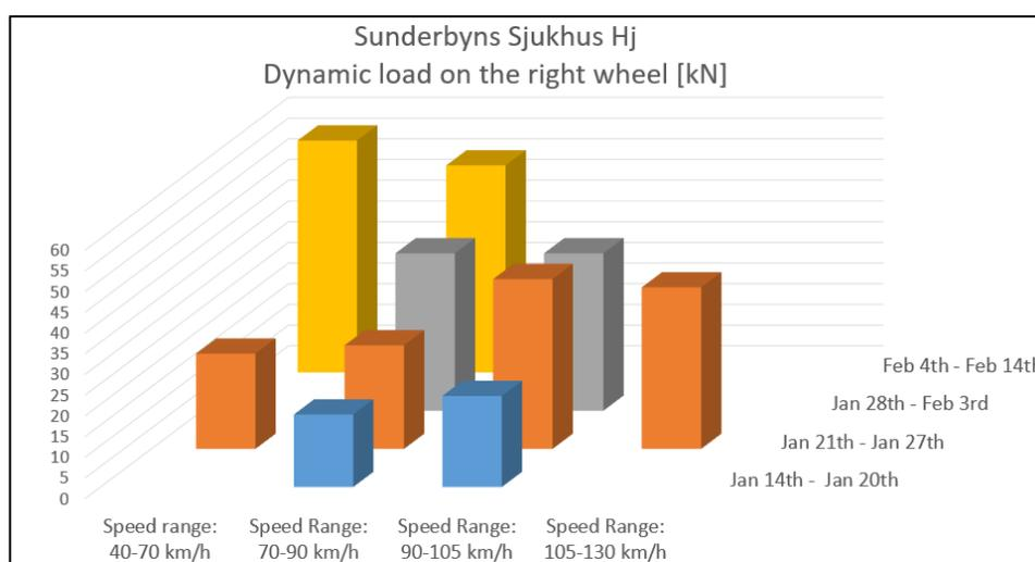
Figure 3.16: 3D-Bar plot showing the mean of dynamic loads registered for the **right** wheel of the first axle of locomotive **917400014341** at the Sunderbyns Sjukhus detector station during specific time intervals and for specific train speed ranges. The vertical axis shows the dynamic load values. The Y-axis shows the time intervals at which data have been registered, while the X-axis shows the considered speed ranges.
