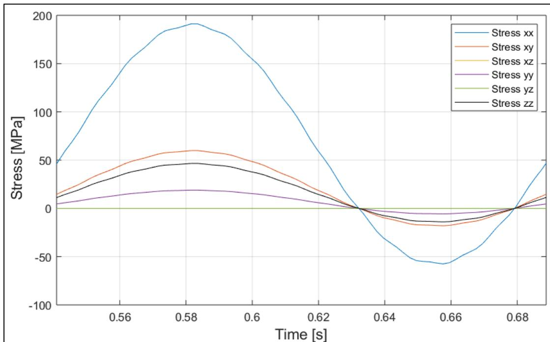
Figure 5.8: Normal and tangential stress of the point of interest in one revolution of the wheel.
