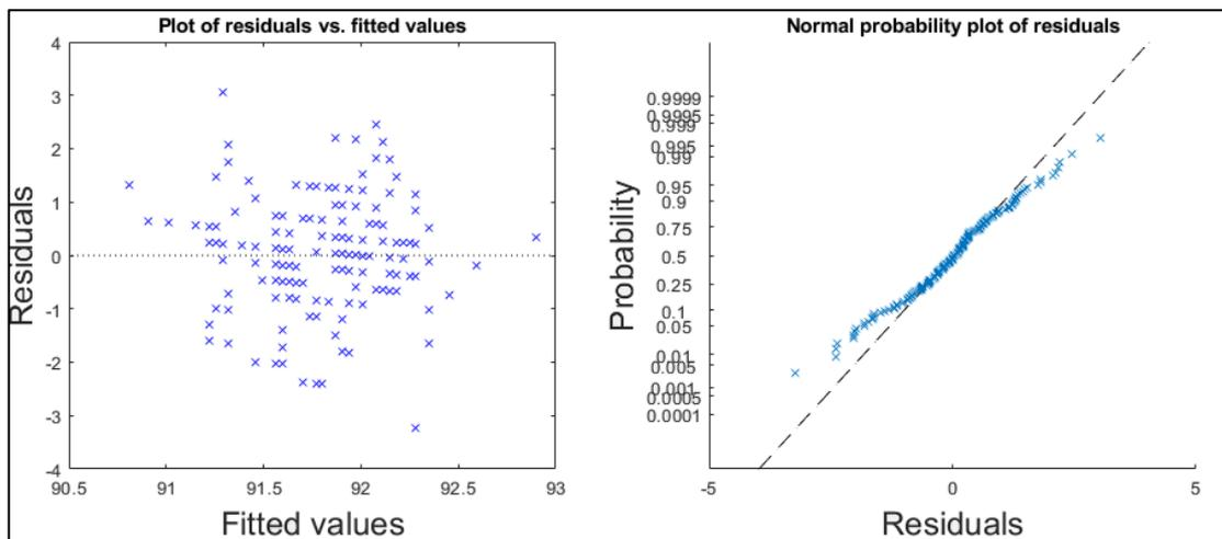
Figure B1.32: Plot of studentized residuals versus fitted values (on the left) and probability plot (on the right) derived from the simple linear regression model between train speed and mean wheel loads detected for the **left** wheel of the first axle of locomotive **917400014235** between March 18<sup>th</sup> 2018 and January 29<sup>th</sup> 2019 at **Jörn** detector station.
