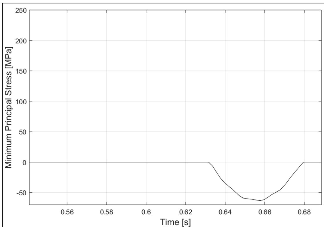
Figure 5.12: Time history of the minimum principal stress evaluated at the node of interest during one revolution of the wheels.
