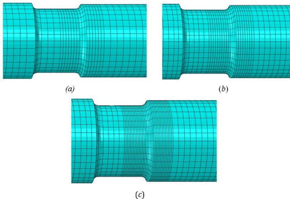
Figure 5.5: Axle mesh. (a) coarse mesh (b) medium mesh (c) fine mesh
