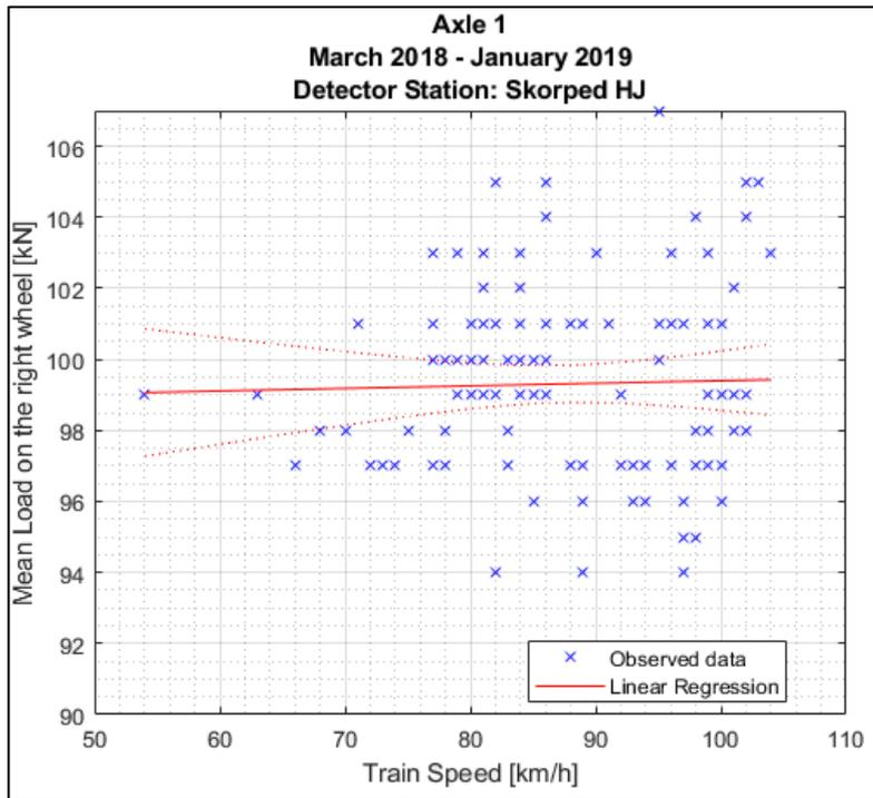
Figure B1.9: Simple linear regression model between train speed and mean wheel loads detected for the **right** wheel of the first axle of locomotive **917400014341** between March 18<sup>th</sup> 2018 and January 29<sup>th</sup> 2019 at **Skorped** detector station.
