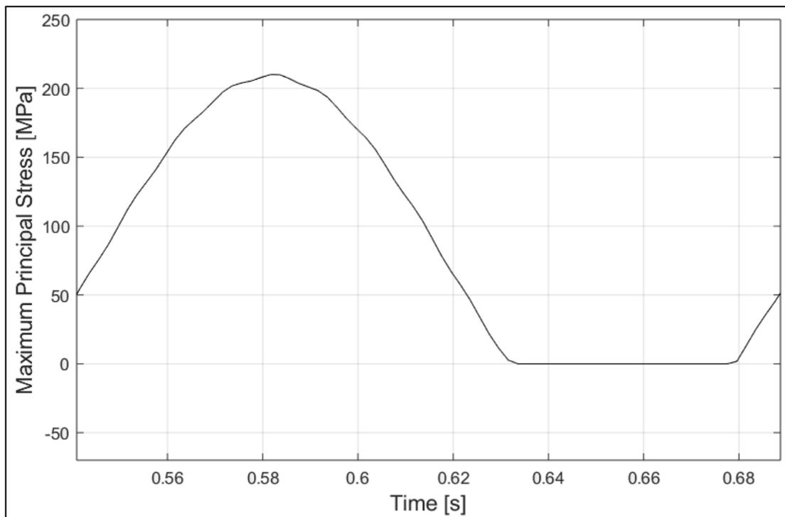
Figure 5.10: Time history of the maximum principal stress evaluated at the node of interest during one revolution of the wheels.
