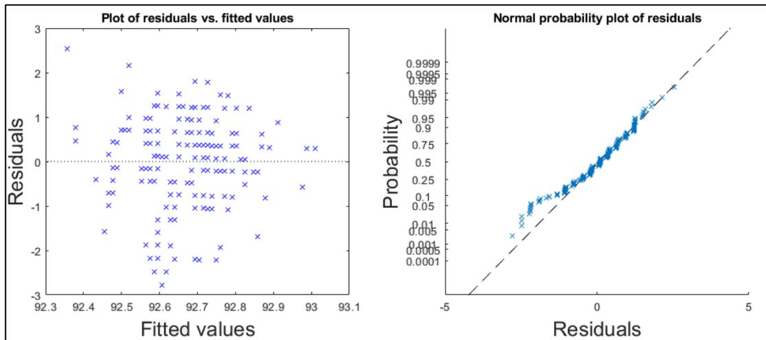
Figure B1.16: Plot of studentized residuals versus fitted values (on the left) and probability plot (on the right) derived from the simple linear regression model between train speed and mean wheel loads detected for the **left** wheel of the first axle of locomotive **917400014234** between March 18<sup>th</sup> 2018 and January 29<sup>th</sup> 2019 at **Jörn** detector station.
