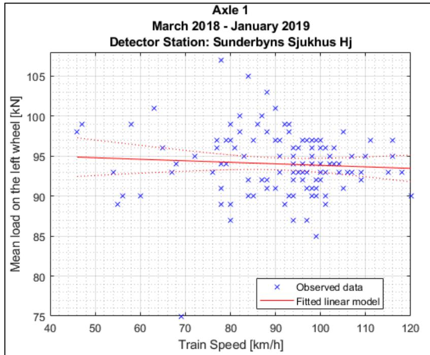
Figure B1.5: Simple linear regression model between train speed and mean wheel loads detected for the **left** wheel of the first axle of locomotive **917400014341** between March 18<sup>th</sup> 2018 and January 29<sup>th</sup> 2019 at **Sunderbyns Sjukhus** detector station.
