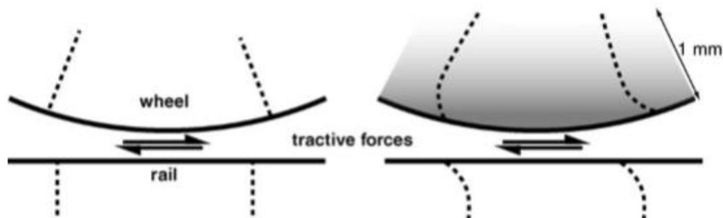
Figure 2.1: Schematic sketch regarding plastic deformation of the surface material in a railway wheel due to tangential loading. The dashed lines indicate material planes before and after deformation [6].
