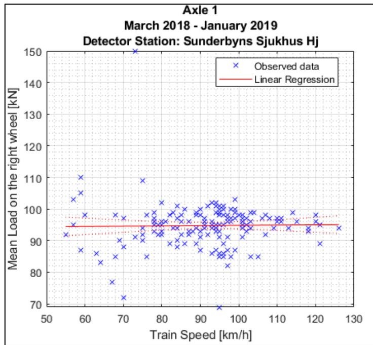
Figure B1.27: Simple linear regression model between train speed and mean wheel loads detected for the **right** wheel of the first axle of locomotive **917400014234** between March 18<sup>th</sup> 2018 and January 29<sup>th</sup> 2019 at **Sunderbyns Sjukhus** detector station.
