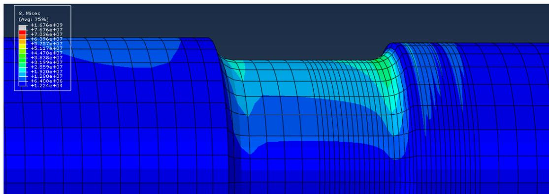
Figure 5.4: Snap shot of the numerical results in terms of Von Mises equivalent stress aimed to visualize the most critical section. The figure refers to the numerical results arisen from the adoption of the “medium” mesh.
