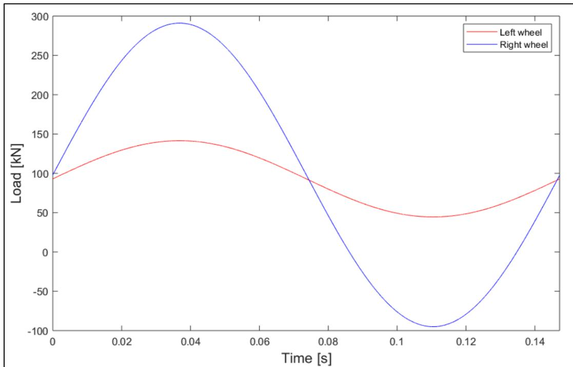
Figure 5.1: Load time history in one revolution of the wheel.
