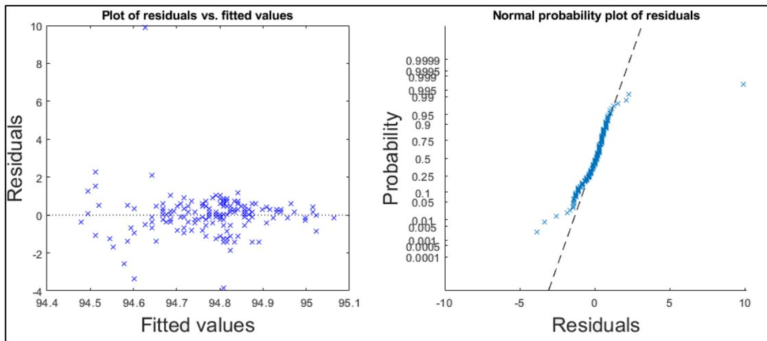
Figure B1.28: Plot of studentized residuals versus fitted values (on the left) and probability plot (on the right) derived from the simple linear regression model between train speed and mean wheel loads detected for the **right** wheel of the first axle of locomotive **917400014234** between March 18<sup>th</sup> 2018 and January 29<sup>th</sup> 2019 at **Sunderbyns Sjukhus** detector station.
