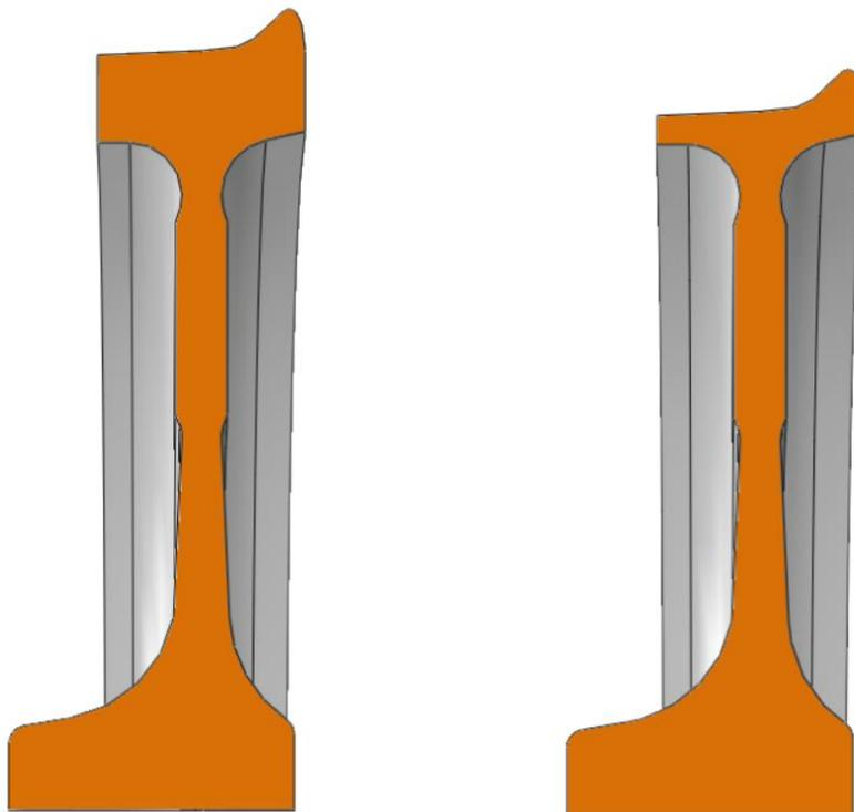
*Figure 4.5: Cross section view of the modelled railway wheel: the wheel having nominal external diameter is shown on the left , whereas critical prescribed external diameter thereof is shown on the right.*
