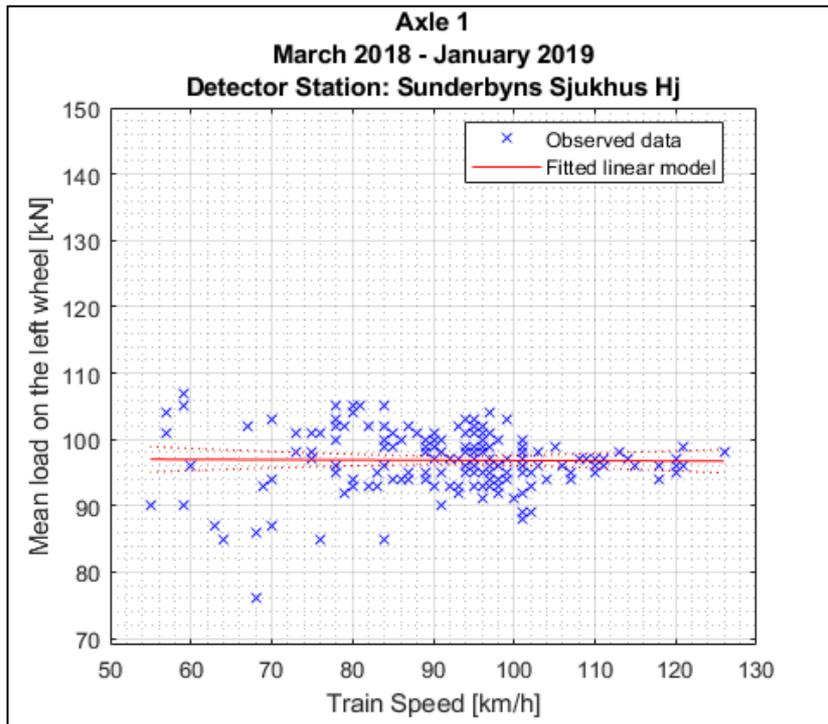
Figure B1.19: Simple linear regression model between train speed and mean wheel loads detected for the **left** wheel of the first axle of locomotive **917400014234** between March 18<sup>th</sup> 2018 and January 29<sup>th</sup> 2019 at **Sunderbyns Sjukhus** detector station.
