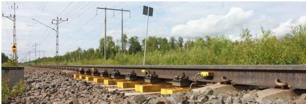
Figure 3.1: Wheel impact load detector (WILD) installed in track [13].
