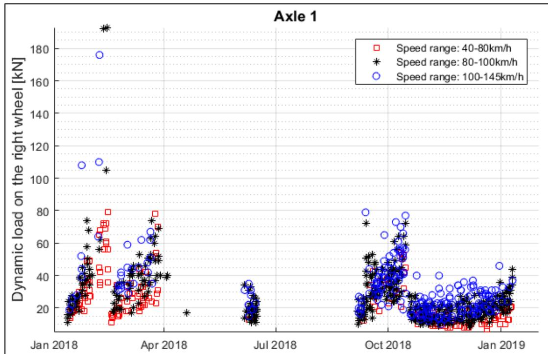
Figure 3.9: Scattered data of dynamic impact loads generated by the **right** wheel of the first axle of locomotive 917400014341 and registered by all WILDs over one year period. The data have been plotted for three different train speed ranges.
