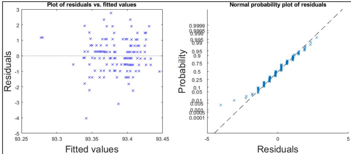
Figure B1.18: Plot of studentized residuals versus fitted values (on the left) and probability plot (on the right) derived from the simple linear regression model between train speed and mean wheel loads detected for the **left** wheel of the first axle of locomotive **917400014234** between March 18<sup>th</sup> 2018 and January 29<sup>th</sup> 2019 at **Koler** detector station.
