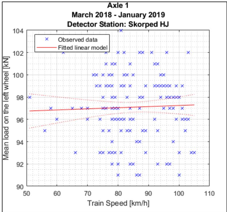
Figure B1.33: Simple linear regression model between train speed and mean wheel loads detected for the **left** wheel of the first axle of locomotive **917400014235** between March 18<sup>th</sup> 2018 and January 29<sup>th</sup> 2019 at **Skorped** detector station.
