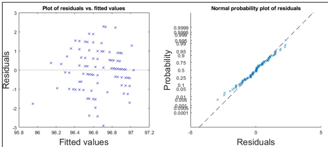
Figure B1.4: Plot of studentized residuals versus fitted values (on the left) and probability plot (on the right) derived from the simple linear regression model between train speed and mean wheel loads detected for the **left** wheel of the first axle of locomotive **917400014341** between March 18<sup>th</sup> 2018 and January 29<sup>th</sup> 2019 at **Skorped** detector station.
