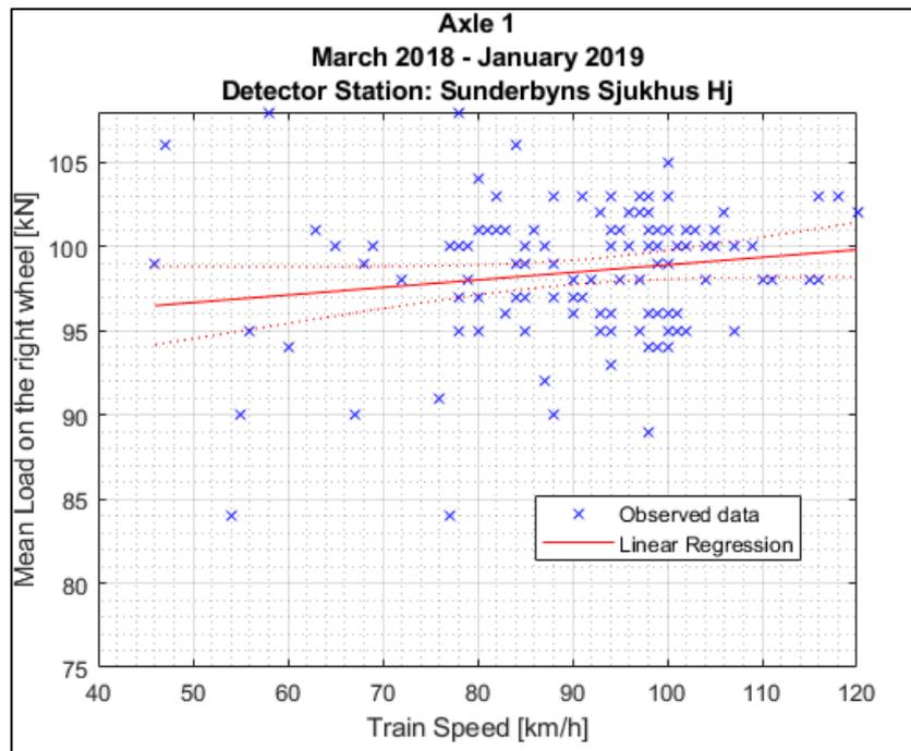
Figure B1.11: Simple linear regression model between train speed and mean wheel loads detected for the **right** wheel of the first axle of locomotive **917400014341** between March 18<sup>th</sup> 2018 and January 29<sup>th</sup> 2019 at **Sunderbyns Sjukhus** detector station.
