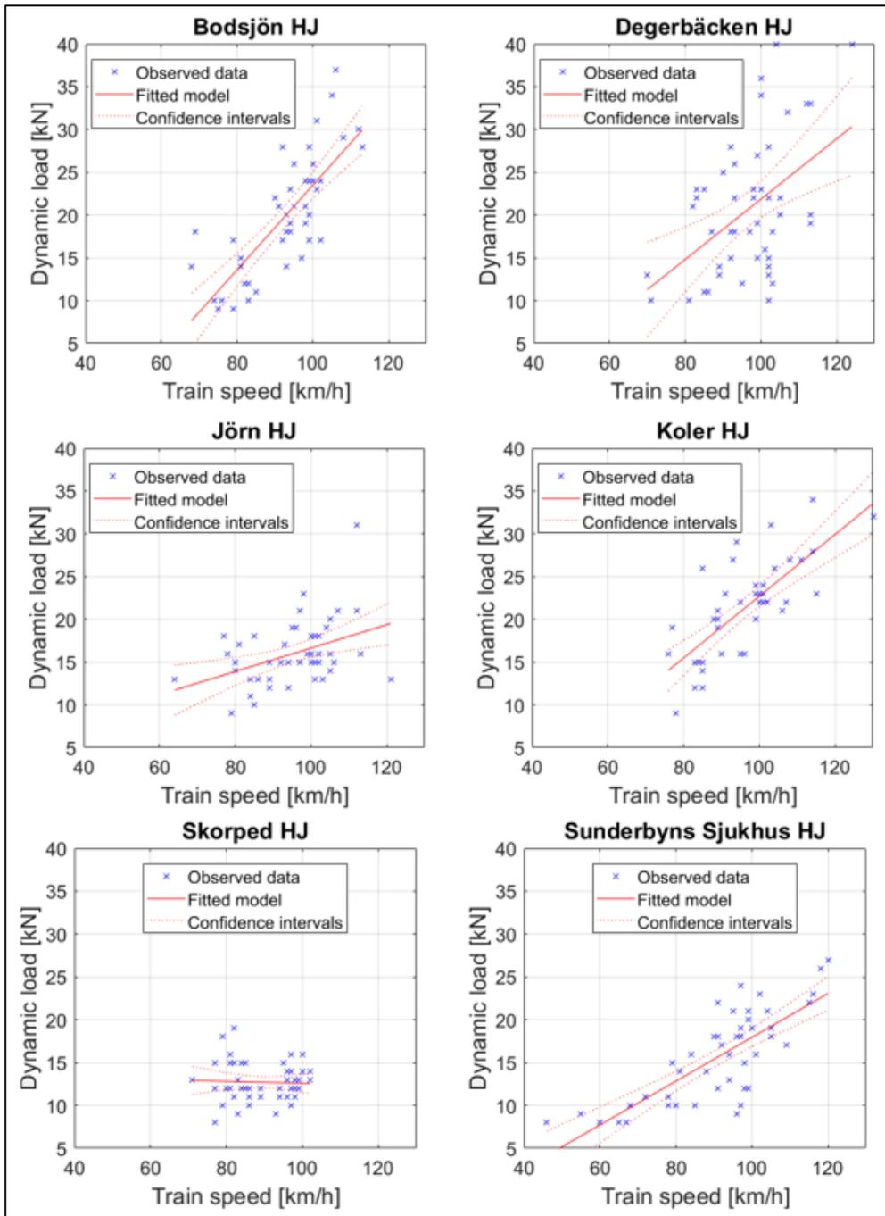
Figure 3.13: Simple linear regression models between train speed and dynamic loads detected for the **right** wheel of the first axle of locomotive 917400014341 between October 18<sup>th</sup> 2018 and December 18<sup>th</sup> for each detector station.
