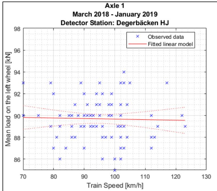
Figure B1.13: Simple linear regression model between train speed and mean wheel loads detected for the **left** wheel of the first axle of locomotive **917400014234** between March 18<sup>th</sup> 2018 and January 29<sup>th</sup> 2019 at **Degerbäcken** detector station.
