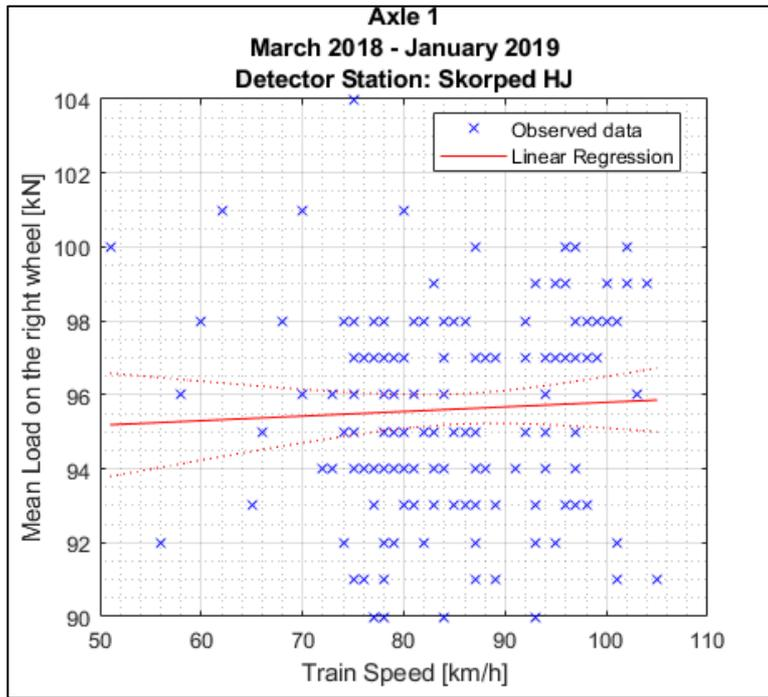
Figure B1.41: Simple linear regression model between train speed and mean wheel loads detected for the **right** wheel of the first axle of locomotive **917400014235** between March 18<sup>th</sup> 2018 and January 29<sup>th</sup> 2019 at **Skorped** detector station.
