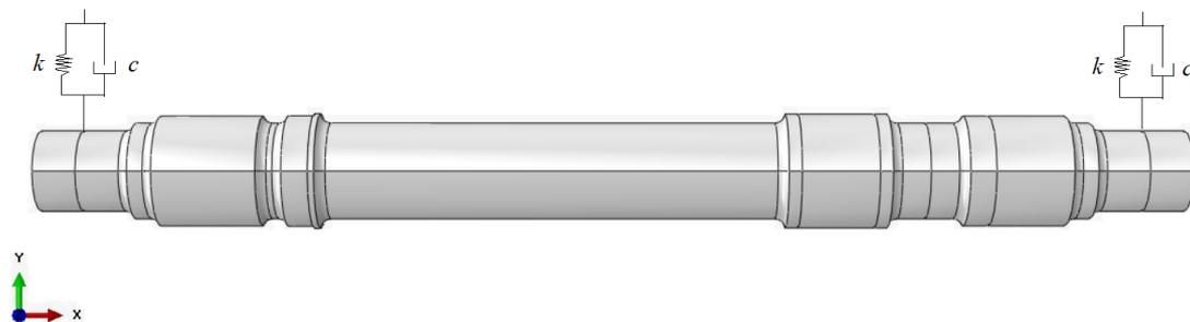
Figure 5.2: Schematic showing the location and the modelling of the primary suspension system.
