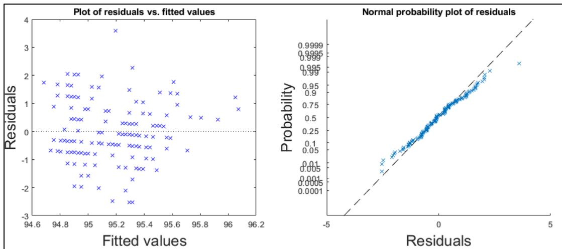
Figure B1.26: Plot of studentized residuals versus fitted values (on the left) and probability plot (on the right) derived from the simple linear regression model between train speed and mean wheel loads detected for the **right** wheel of the first axle of locomotive **917400014234** between March 18<sup>th</sup> 2018 and January 29<sup>th</sup> 2019 at **Skorpéd** detector station.
