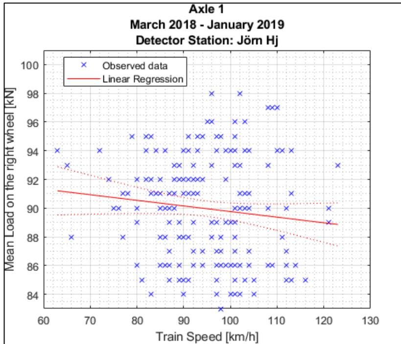
Figure B1.23: Simple linear regression model between train speed and mean wheel loads detected for the **right** wheel of the first axle of locomotive **917400014234** between March 18<sup>th</sup> 2018 and January 29<sup>th</sup> 2019 at **Jörn** detector station.
