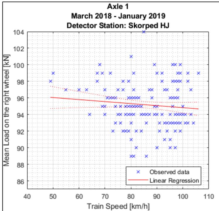
Figure B1.25: Simple linear regression model between train speed and mean wheel loads detected for the **right** wheel of the first axle of locomotive **917400014234** between March 18<sup>th</sup> 2018 and January 29<sup>th</sup> 2019 at **Skorpéd** detector station.
