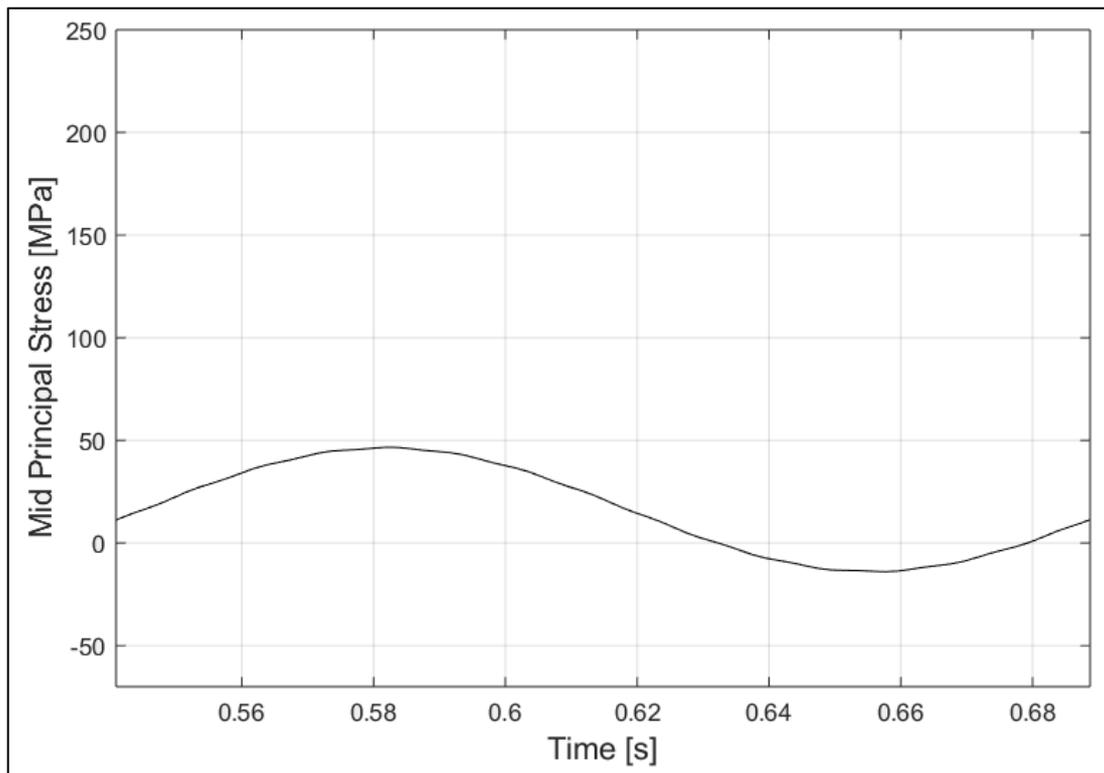
Figure 5.11: Time history of the mid principal stress evaluated at the node of interest during one revolution of the wheels.
