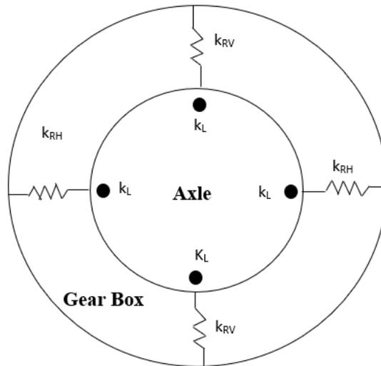
Figure 4.3: Schematic illustrating the modelled interaction between axle and gear box.
