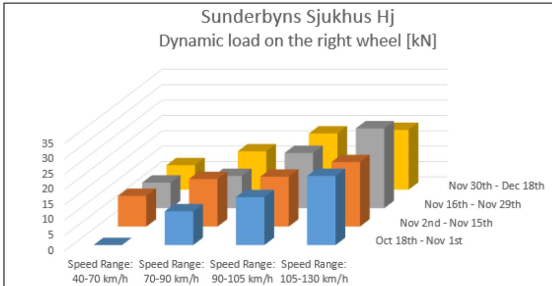
Figure 3.10: 3D-Bar plot showing the mean of dynamic loads registered for the **right** wheel of the first axle of locomotive **917400014341** at the Sunderbyns Sjukhus detector station during specific time intervals and for specific train speed ranges. The vertical axis shows the dynamic load values. The Y-axis shows the time intervals at which data have been registered, while the X-axis shows the considered speed ranges.
