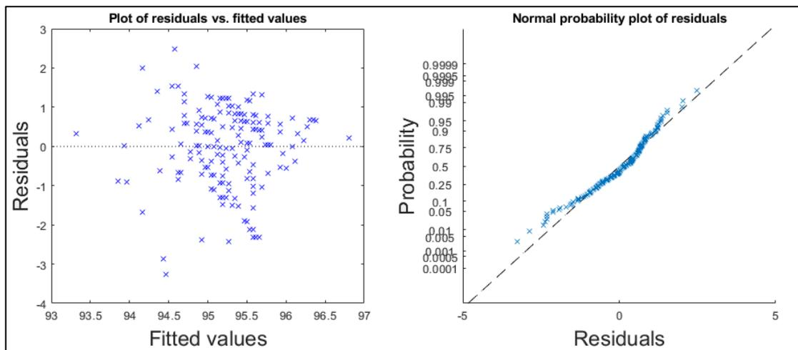
Figure B1.44: Plot of studentized residuals versus fitted values (on the left) and probability plot (on the right) derived from the simple linear regression model between train speed and mean wheel loads detected for the **left** wheel of the first axle of locomotive **917400014235** between March 18<sup>th</sup> 2018 and January 29<sup>th</sup> 2019 at **Sunderbyns Sjukhus** detector station.
