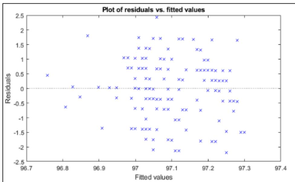
Figure 3.6: Plot of studentized residuals versus fitted values derived from the simple linear regression model between train speed and mean wheel loads detected for the **left** wheel of the first axle of locomotive 917400014325 between March 18<sup>th</sup> 2018 and January 29<sup>th</sup> 2019 at **Skorped** detector station.
