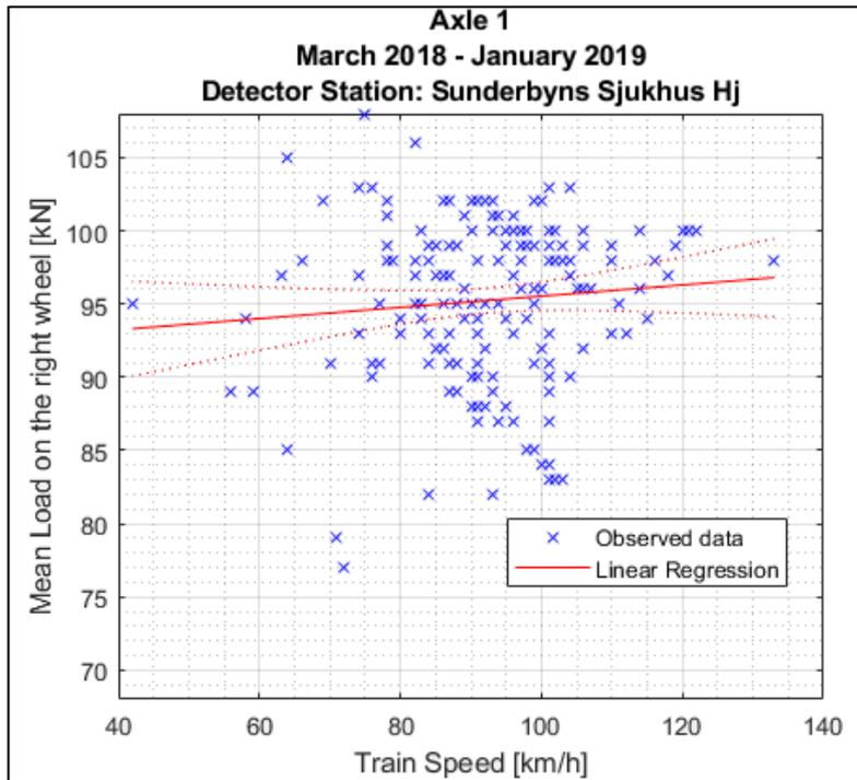
Figure B1.43: Simple linear regression model between train speed and mean wheel loads detected for the **right** wheel of the first axle of locomotive **917400014235** between March 18<sup>th</sup> 2018 and January 29<sup>th</sup> 2019 at **Sunderbyns Sjukhus** detector station.
