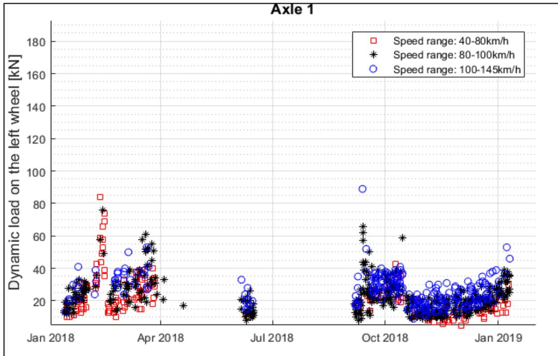
Figure B1.45: Scattered data of dynamic impact loads acting for the **left** wheel of the first axle of locomotive **917400014341** registered by WILDs over one year period. The data have been plotted for three different train speed ranges.
