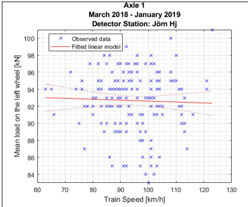
Figure B1.15: Simple linear regression model between train speed and mean wheel loads detected for the **left** wheel of the first axle of locomotive **917400014234** between March 18<sup>th</sup> 2018 and January 29<sup>th</sup> 2019 at **Jörn** detector station.
