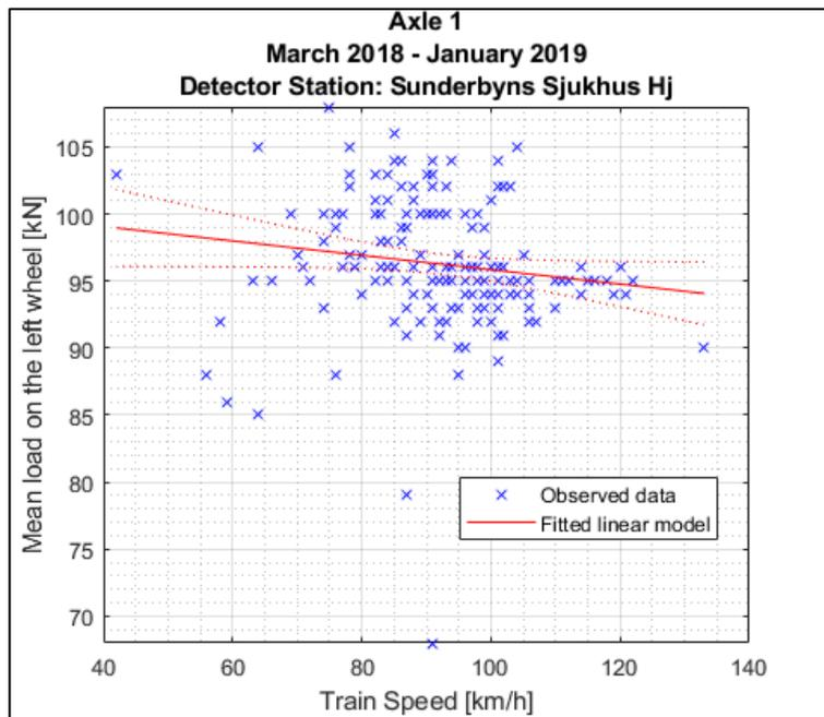
Figure B1.35: Simple linear regression model between train speed and mean wheel loads detected for the **left** wheel of the first axle of locomotive **917400014235** between March 18<sup>th</sup> 2018 and January 29<sup>th</sup> 2019 at **Sunderbyns Sjukhus** detector station.
