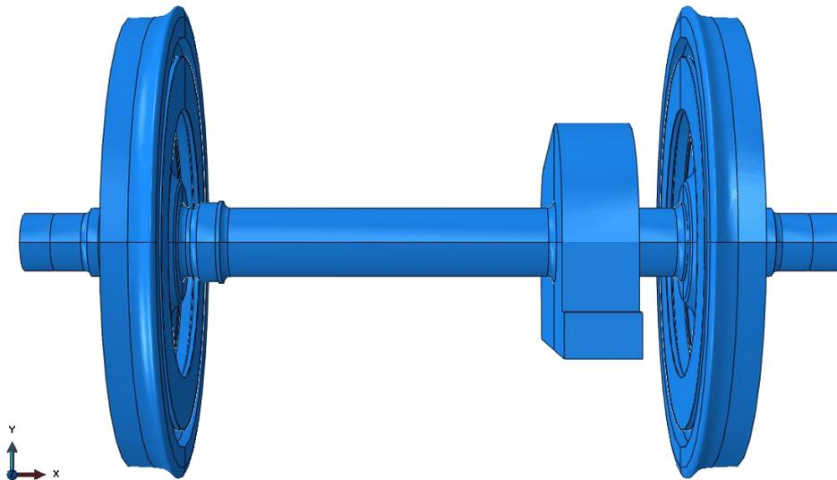
Figure 4.4: Frontal view of the wheelset model in Abaqus CAD interface.
