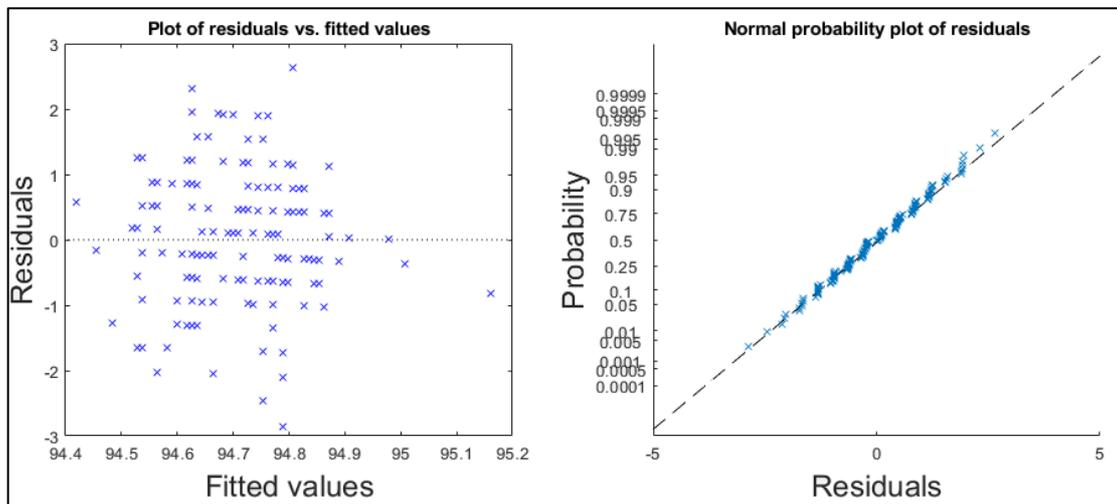
Figure B1.40: Plot of studentized residuals versus fitted values (on the left) and probability plot (on the right) derived from the simple linear regression model between train speed and mean wheel loads detected for the **left** wheel of the first axle of locomotive **917400014235** between March 18<sup>th</sup> 2018 and January 29<sup>th</sup> 2019 at **Koler** detector station.
