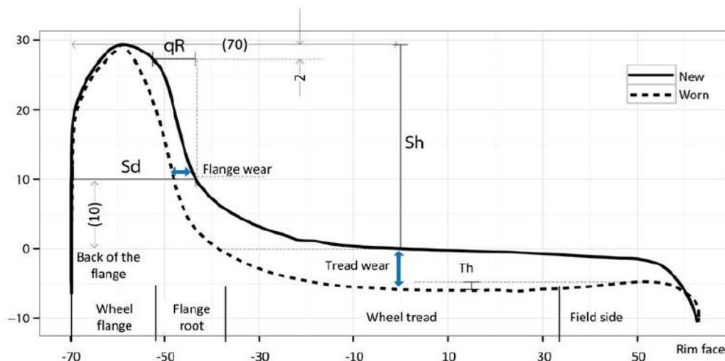
Figure 2.4: Typical railway wheel profile. The picture shows also flange and tread wear phenomena [11].
