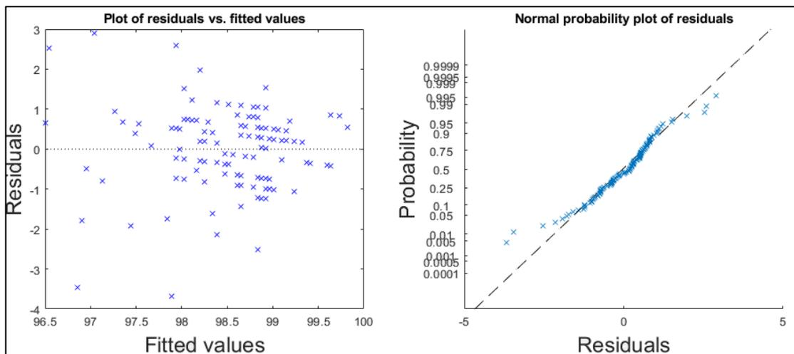
Figure B1.12: Plot of studentized residuals versus fitted values (on the left) and probability plot (on the right) derived from the simple linear regression model between train speed and mean wheel loads detected for the **right** wheel of the first axle of locomotive **917400014341** between March 18<sup>th</sup> 2018 and January 29<sup>th</sup> 2019 at **Sunderbyns Sjukhus** detector station.
