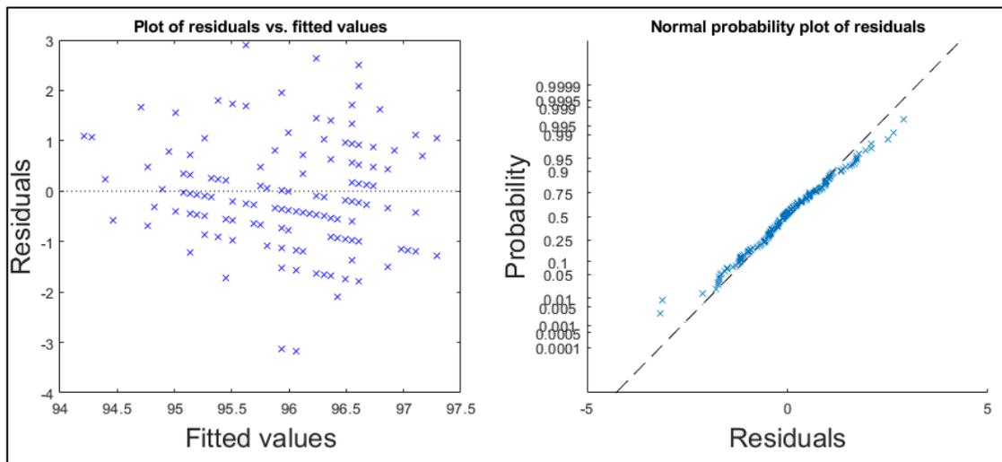
Figure B1.30: Plot of studentized residuals versus fitted values (on the left) and probability plot (on the right) derived from the simple linear regression model between train speed and mean wheel loads detected for the **left** wheel of the first axle of locomotive **917400014235** between March 18<sup>th</sup> 2018 and January 29<sup>th</sup> 2019 at **Degerbücken** detector station.
