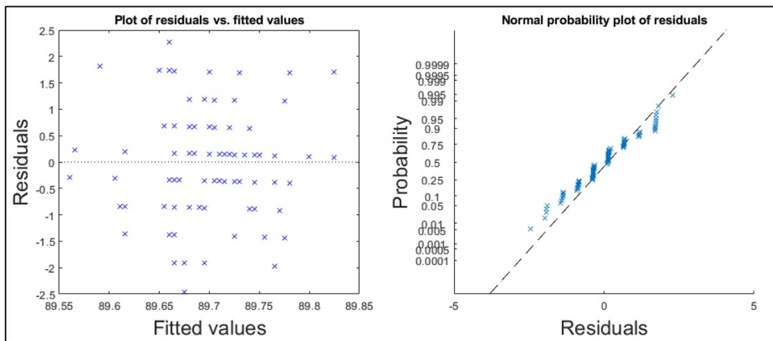
Figure B1.14: Plot of studentized residuals versus fitted values (on the left) and probability plot (on the right) derived from the simple linear regression model between train speed and mean wheel loads detected for the **left** wheel of the first axle of locomotive **917400014234** between March 18<sup>th</sup> 2018 and January 29<sup>th</sup> 2019 at **Degerbäcken** detector station.
