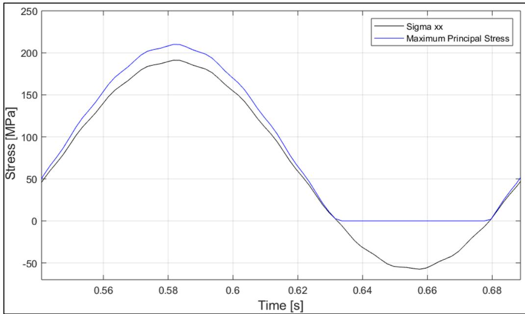
Figure 5.9: Time history in one revolution of the wheels of the maximum principal stress and normal stress due to the bending.
