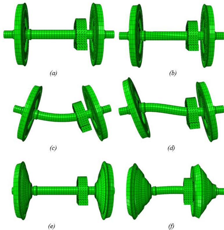
Figure 4.6: Elastic modes of the wheelset: (a) Undeformed wheelset. (b) Mode 3. (c) Mode 4. (d) Mode 7. (e) Mode 11. (f) Mode 17.
