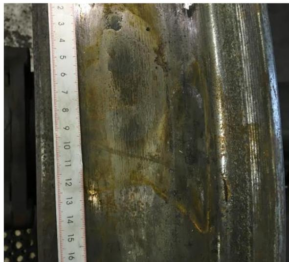
Figure 2.3: Wheel flat on the tread surface. [Picture courtesy Michele Maria Maglio].
