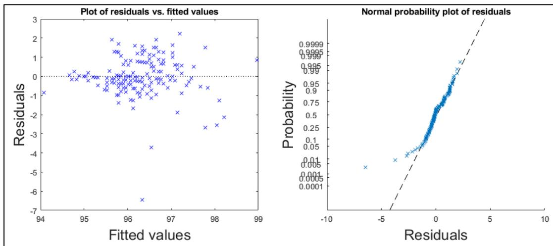
Figure B1.36: Plot of studentized residuals versus fitted values (on the left) and probability plot (on the right) derived from the simple linear regression model between train speed and mean wheel loads detected for the **left** wheel of the first axle of locomotive **917400014235** between March 18<sup>th</sup> 2018 and January 29<sup>th</sup> 2019 at **Sunderbyns Sjukhus** detector station.
