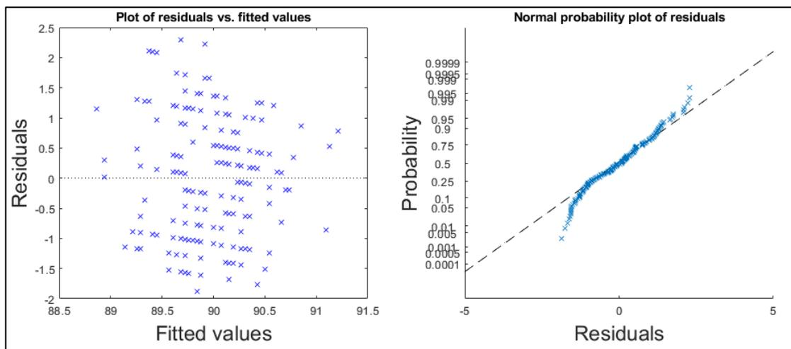
Figure B1.24: Plot of studentized residuals versus fitted values (on the left) and probability plot (on the right) derived from the simple linear regression model between train speed and mean wheel loads detected for the **right** wheel of the first axle of locomotive **917400014234** between March 18<sup>th</sup> 2018 and January 29<sup>th</sup> 2019 at **Jörn** detector station.
