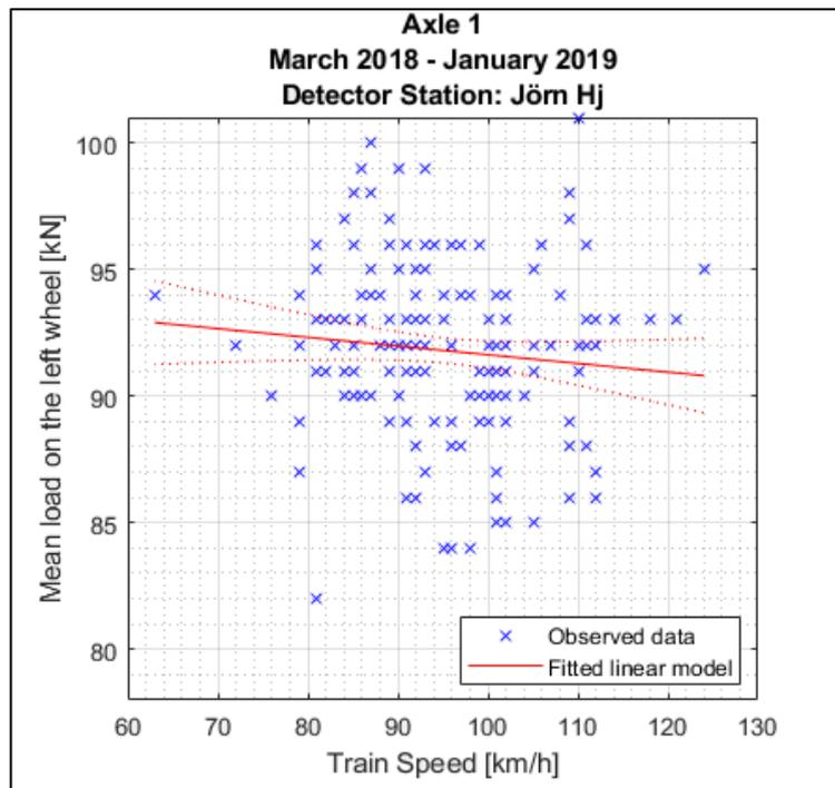
Figure B1.31: Simple linear regression model between train speed and mean wheel loads detected for the **left** wheel of the first axle of locomotive **917400014235** between March 18<sup>th</sup> 2018 and January 29<sup>th</sup> 2019 at **Jörn** detector station.
