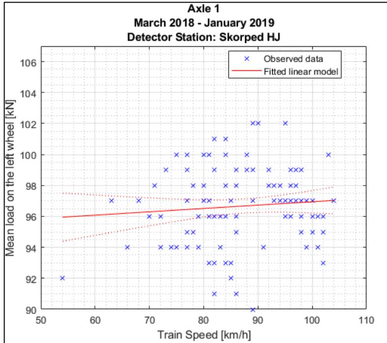
Figure B1.3: Simple linear regression model between train speed and mean wheel loads detected for the **left** wheel of the first axle of locomotive **917400014341** between March 18<sup>th</sup> 2018 and January 29<sup>th</sup> 2019 at **Skorped** detector station.
