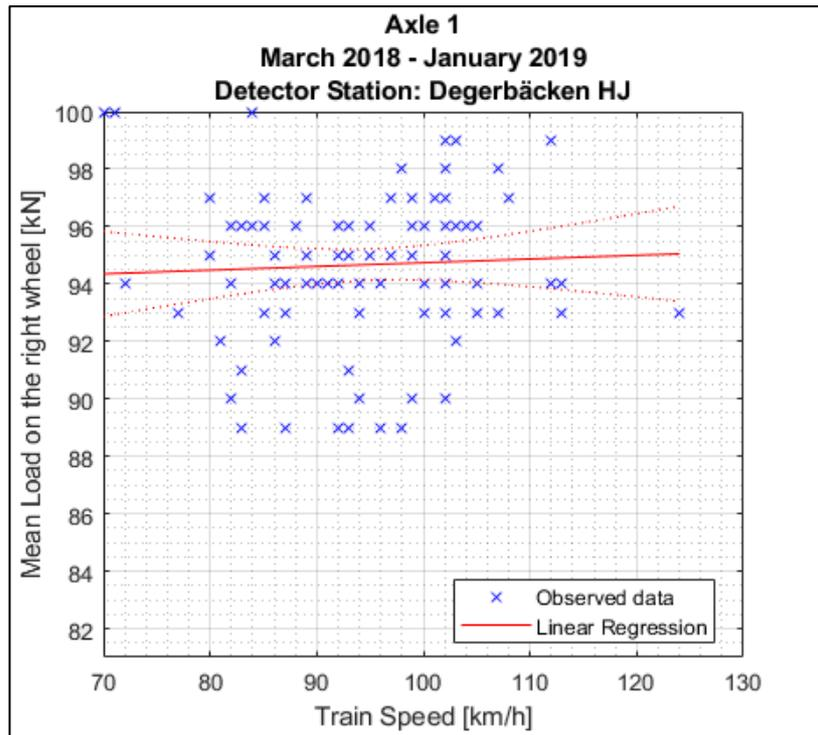
Figure B1.7: Simple linear regression model between train speed and mean wheel loads detected for the **right** wheel of the first axle of locomotive **917400014341** between March 18<sup>th</sup> 2018 and January 29<sup>th</sup> 2019 at **Degerbäcken** detector station.
