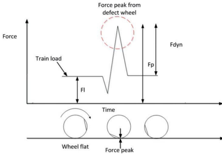
Figure 1.1: Theoretical description of an impact force acting on the wheel of a railway vehicle [4].
