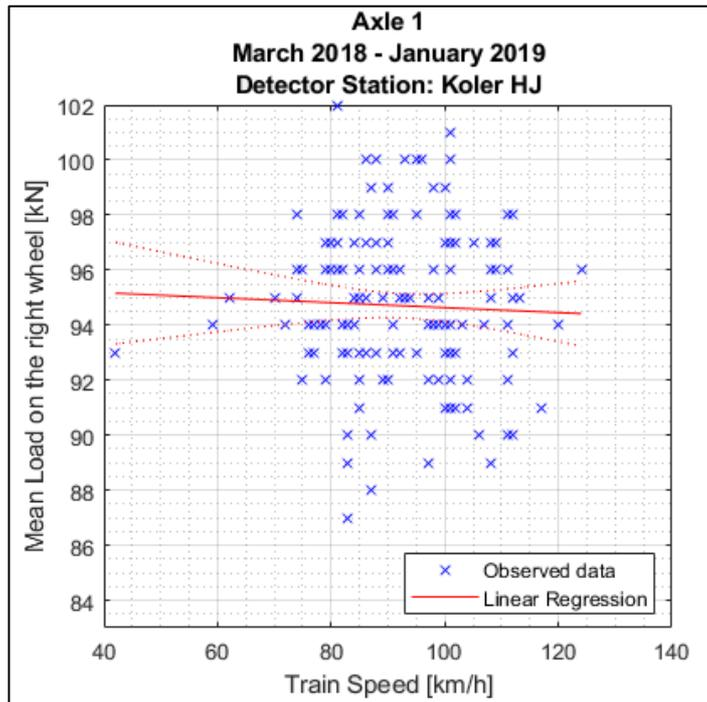
Figure B1.39: Simple linear regression model between train speed and mean wheel loads detected for the **right** wheel of the first axle of locomotive **917400014235** between March 18<sup>th</sup> 2018 and January 29<sup>th</sup> 2019 at **Koler** detector station.
