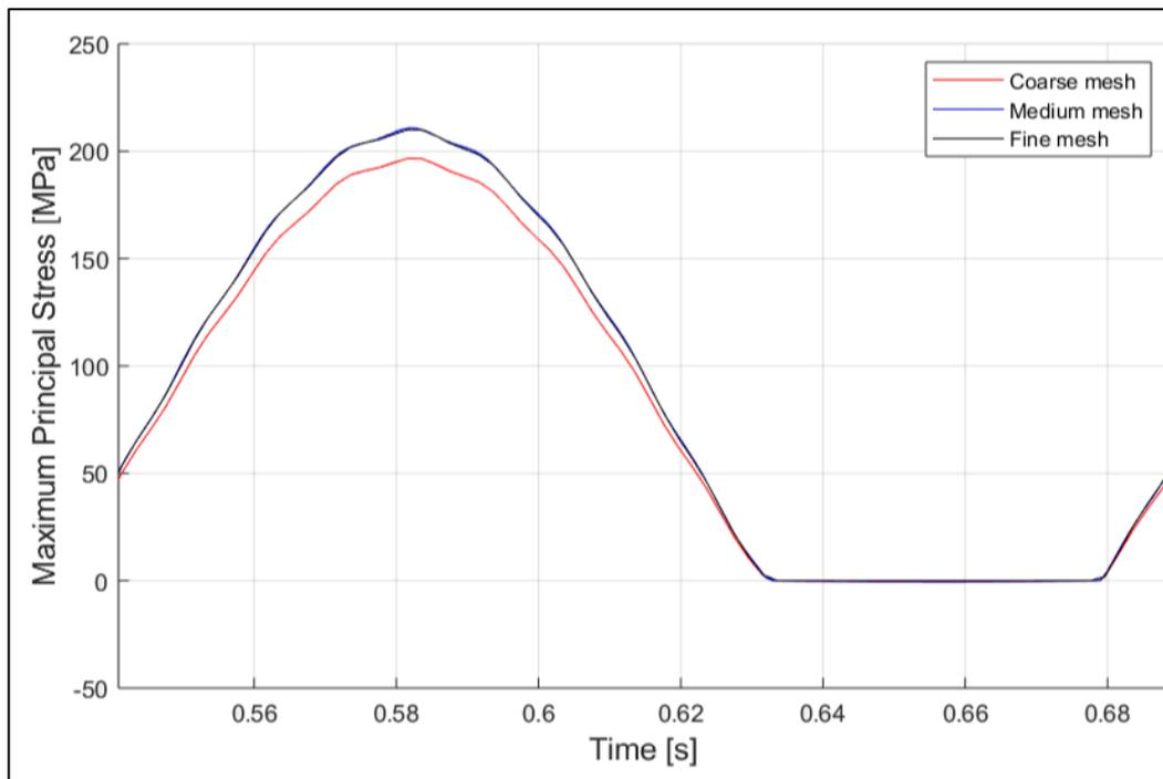
Figure 5.6: Comparison of the maximum principal stress time histories in one revolution of the wheel using the three different meshes.
