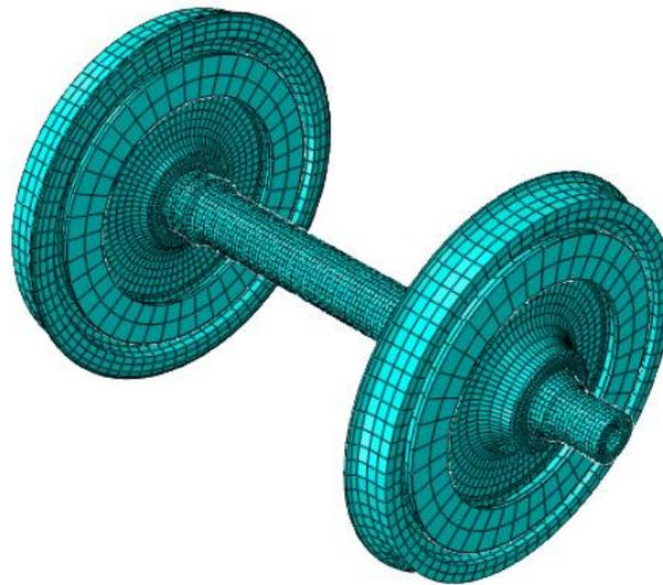
Figure 5.3: Mesh of the wheelset model. The figure refers to the final mesh adopted for extracting the numerical results.
