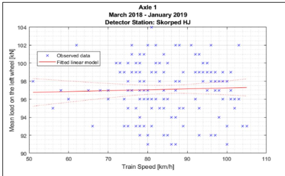
Figure 3.5: Simple linear regression model between train speed and mean wheel loads detected for the **left** wheel of the first axle of locomotive 917400014325 between March 18<sup>th</sup> 2018 and January 29<sup>th</sup> 2019 at **Skorped** detector station. Red dashed lines account for the confidence bounds.
