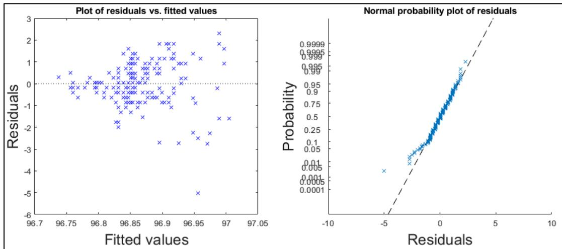
Figure B1.20: Plot of studentized residuals versus fitted values (on the left) and probability plot (on the right) derived from the simple linear regression model between train speed and mean wheel loads detected for the **left** wheel of the first axle of locomotive **917400014234** between March 18<sup>th</sup> 2018 and January 29<sup>th</sup> 2019 at **Koler** detector station.
