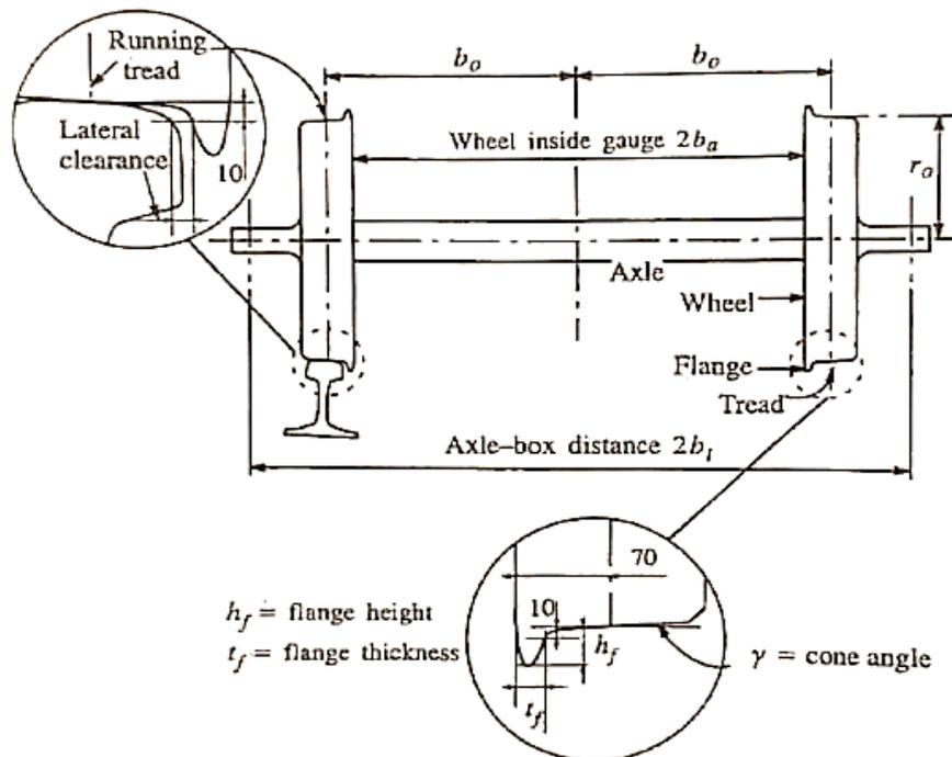
Figure 4.2: Schematic of a conventional wheelset. Measures in mm. [22]
