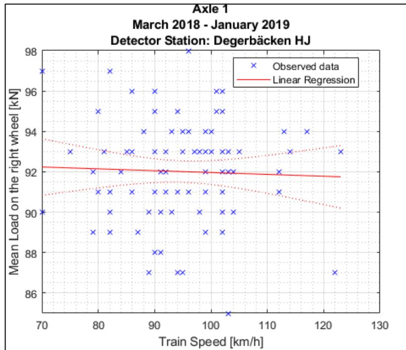
Figure B1.21: Simple linear regression model between train speed and mean wheel loads detected for the **right** wheel of the first axle of locomotive **917400014234** between March 18<sup>th</sup> 2018 and January 29<sup>th</sup> 2019 at **Degerbäcken** detector station.
