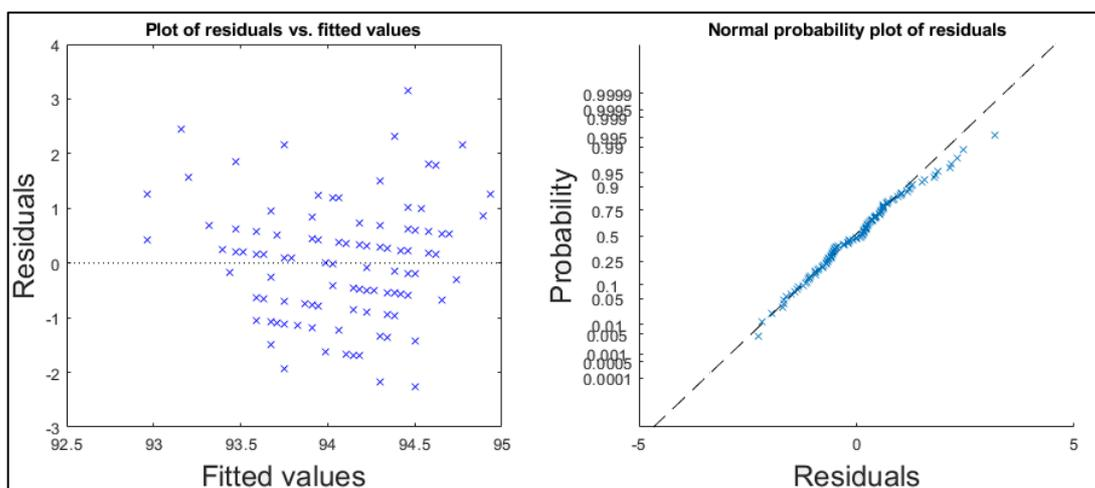
Figure B1.2: Plot of studentized residuals versus fitted values (on the left) and probability plot (on the right) derived from the simple linear regression model between train speed and mean wheel loads
