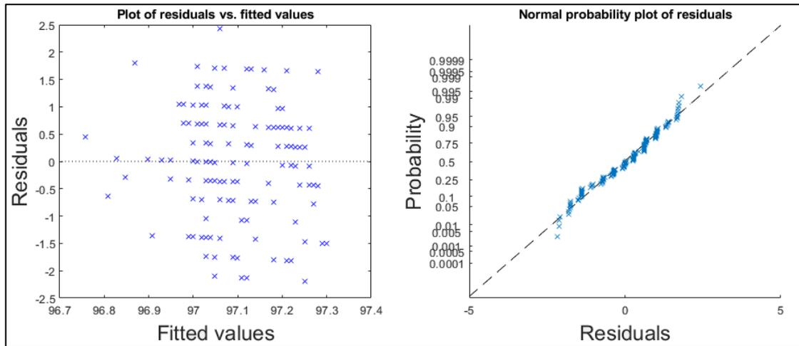
Figure B1.34: Plot of studentized residuals versus fitted values (on the left) and probability plot (on the right) derived from the simple linear regression model between train speed and mean wheel loads detected for the **left** wheel of the first axle of locomotive **917400014235** between March 18<sup>th</sup> 2018 and January 29<sup>th</sup> 2019 at **Skorped** detector station.
