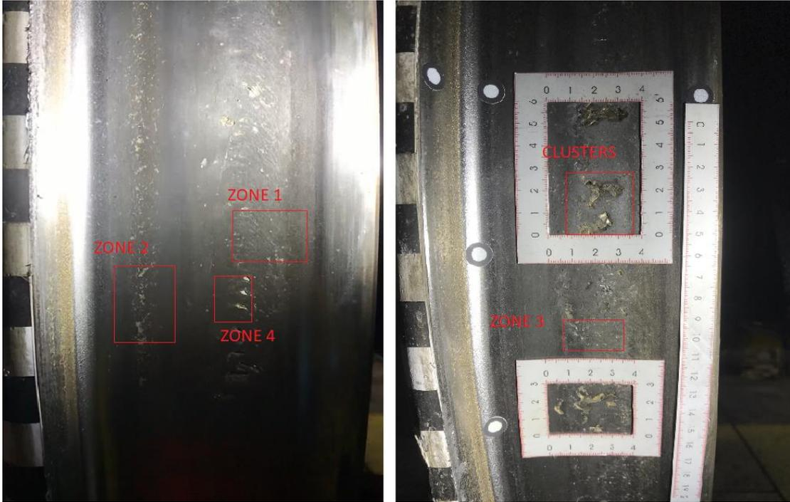
Figure 2.2: RCF damage on a locomotive wheel. [Picture courtesy Michele Maria Maglio].
