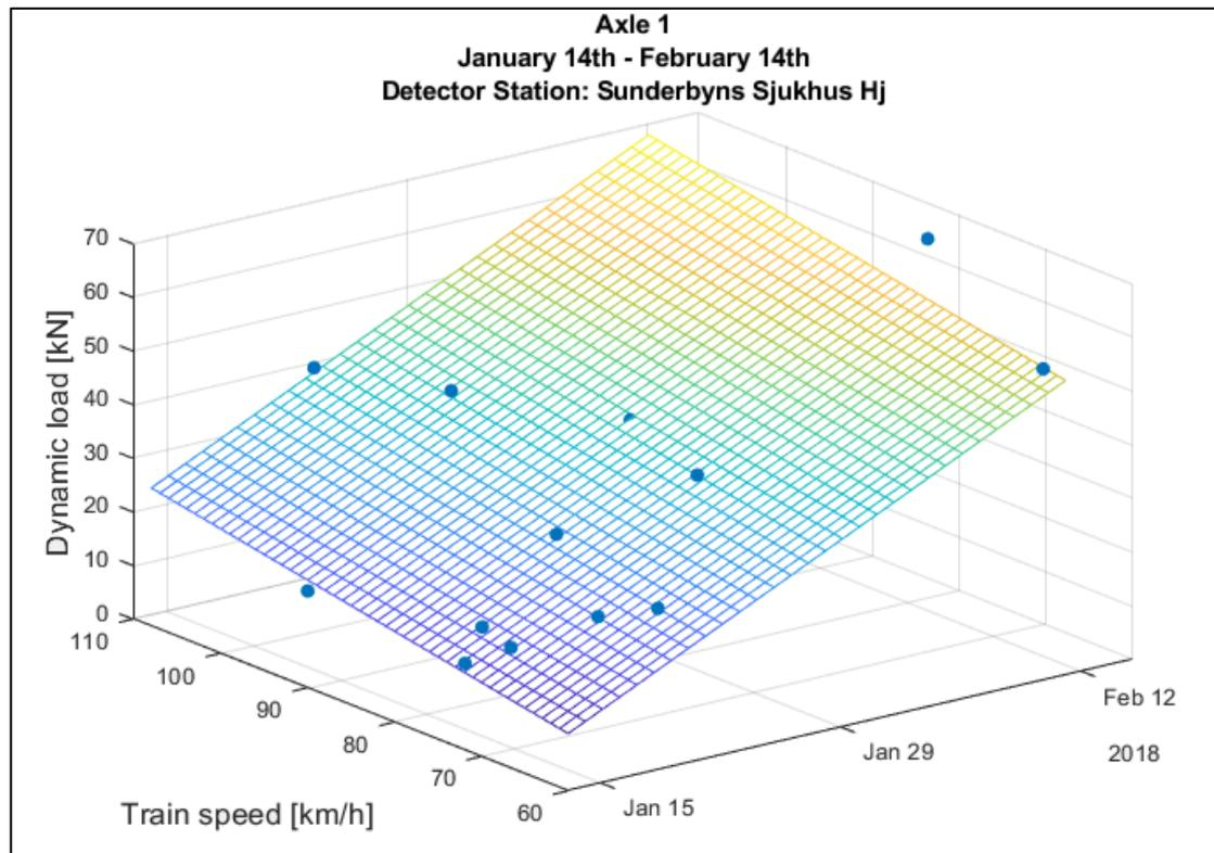
Figure 3.17: Surface fitting of dynamic impact loads expressed as a linear function of time and train speed. Data have been registered at the Sunderbyns Sjukhus detector station and referring to dynamic impact loads detected for the **right** wheel of the first axle of locomotive **917400014341** between January 14<sup>th</sup> and February 14<sup>th</sup> 2018.
