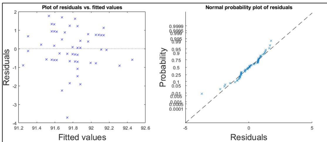
Figure B1.38: Plot of studentized residuals versus fitted values (on the left) and probability plot (on the right) derived from the simple linear regression model between train speed and mean wheel loads detected for the **left** wheel of the first axle of locomotive **917400014235** between March 18<sup>th</sup> 2018 and January 29<sup>th</sup> 2019 at **Degerbäcken** detector station.
