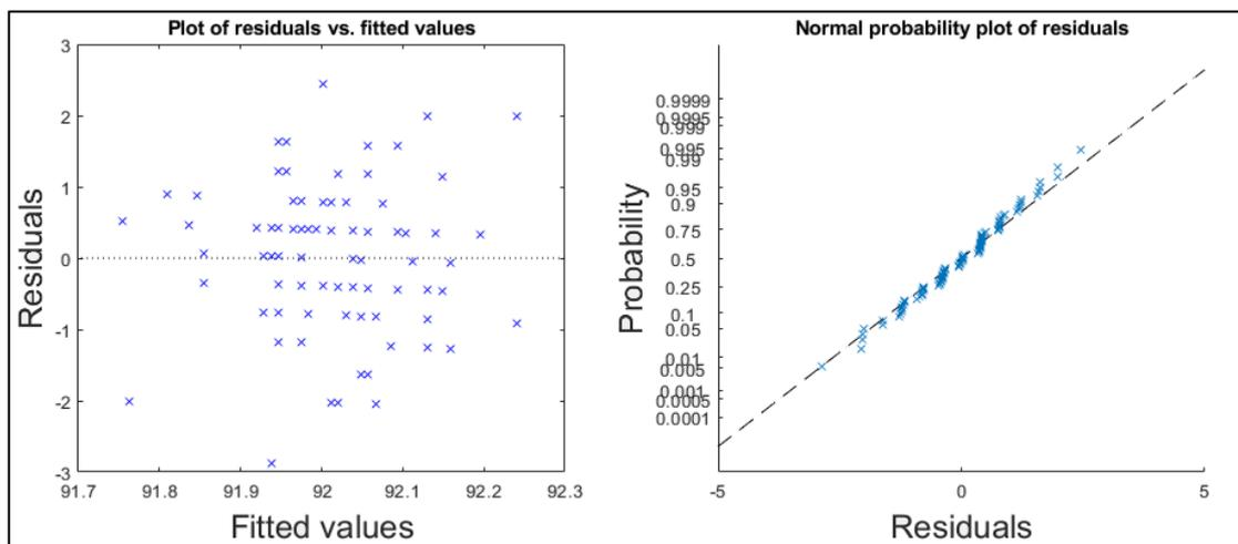
Figure B1.22: Plot of studentized residuals versus fitted values (on the left) and probability plot (on the right) derived from the simple linear regression model between train speed and mean wheel loads detected for the **right** wheel of the first axle of locomotive **917400014234** between March 18<sup>th</sup> 2018 and January 29<sup>th</sup> 2019 at **Degerbäcken** detector station.
