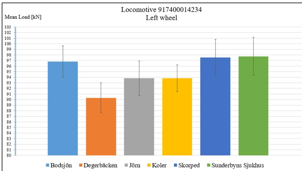
Figure 3.7: 2D-Bar plot showing the average value of mean loads registered for the **left** wheel of the first axle of locomotive **917400014234** at each detector station in the period of time **May 1<sup>st</sup> 2018 to November 1<sup>st</sup> 2019**. The vertical axis shows the average of the mean load. The thin vertical line for each bar allows to identify the upper and lower bounds for the sample data standard deviation.
