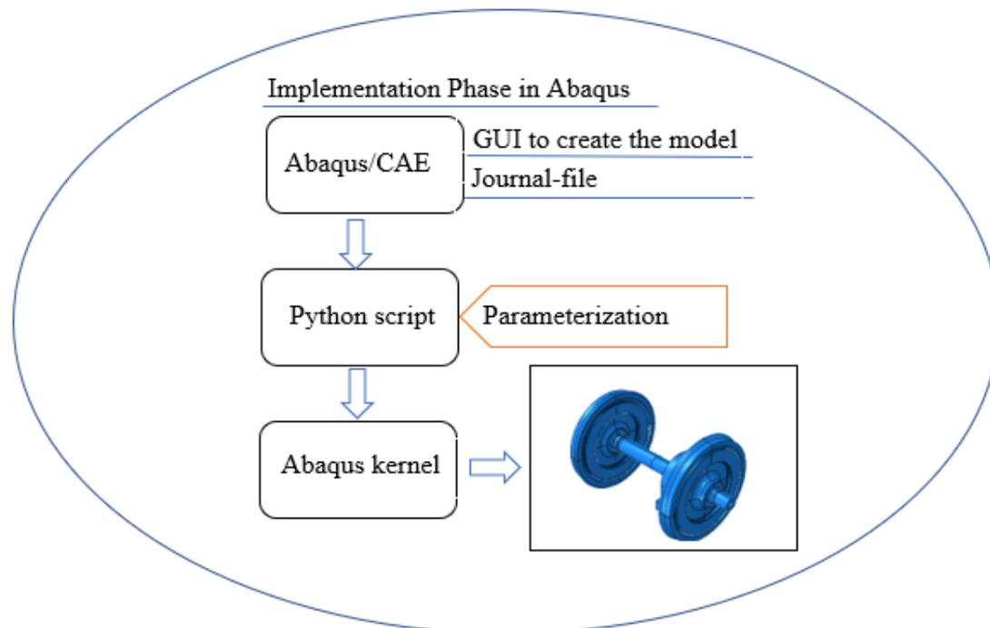
Figure 4.1: Block diagram summarizing the implementation procedure in Abaqus.
