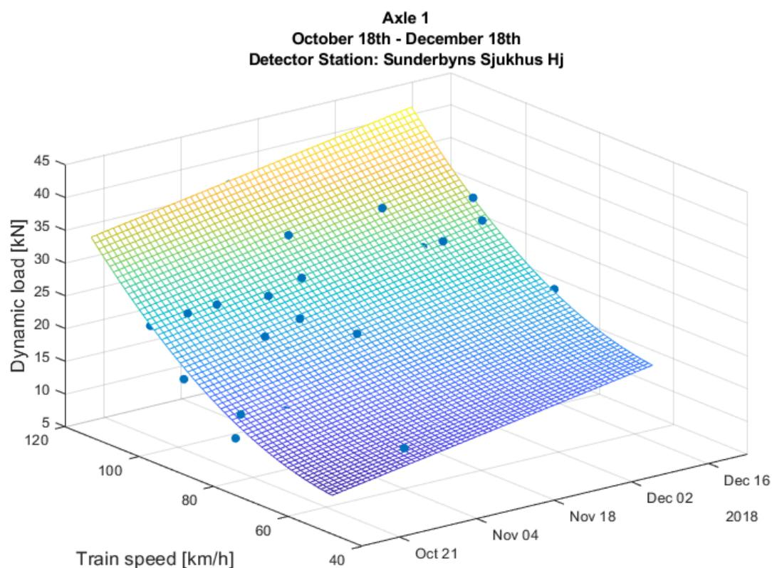
Figure 3.11: Surface fitting of dynamic impact loads expressed as a linear function of time and including both linear and quadratic terms of the train speed. Data have been registered by the **Sunderbyns Sjukhus** detector station and referring to dynamic impact loads measured for the **right** wheel of the first axle of locomotive **917400014341** between October 18<sup>th</sup> and December 18<sup>th</sup> 2018.
