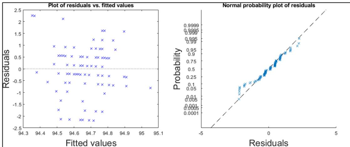
Figure B1.8: Plot of studentized residuals versus fitted values (on the left) and probability plot (on the right) derived from the simple linear regression model between train speed and mean wheel loads detected for the **right** wheel of the first axle of locomotive **917400014341** between March 18<sup>th</sup> 2018 and January 29<sup>th</sup> 2019 at **Degerbäcken** detector station.
