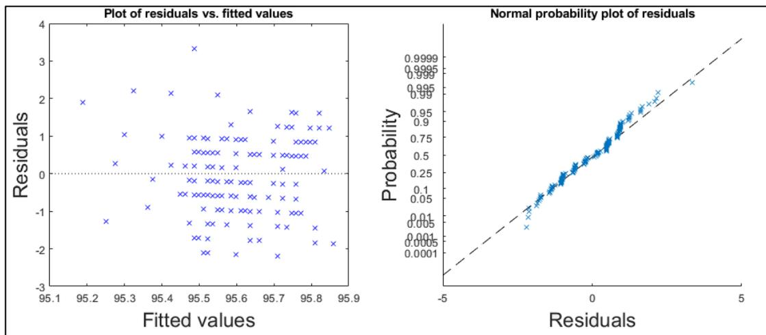
Figure B1.42: Plot of studentized residuals versus fitted values (on the left) and probability plot (on the right) derived from the simple linear regression model between train speed and mean wheel loads detected for the **left** wheel of the first axle of locomotive **917400014235** between March 18<sup>th</sup> 2018 and January 29<sup>th</sup> 2019 at **Skorped** detector station.
