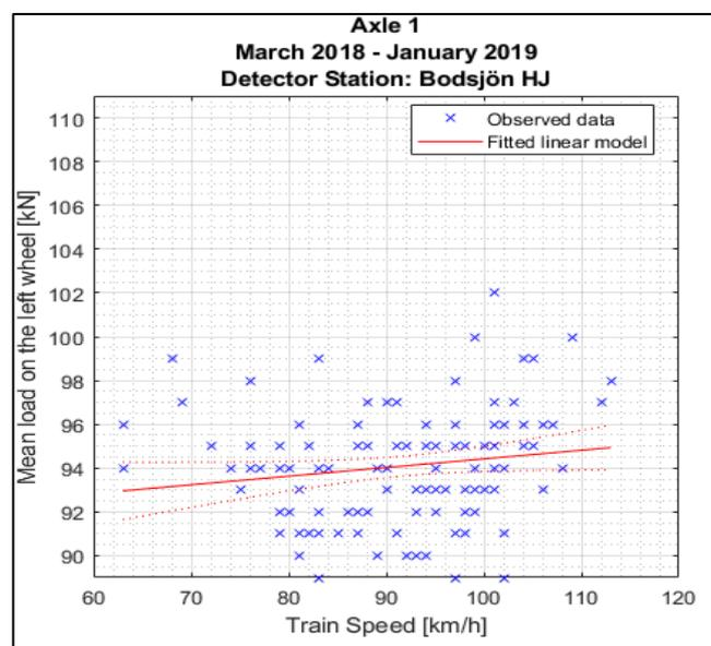
Figure B1.1: Simple linear regression model between train speed and mean wheel loads detected for the left wheel of the first axle of locomotive 917400014341 between March 18<sup>th</sup> 2018 and January 29<sup>th</sup> 2019 at Bodsjön detector station.
