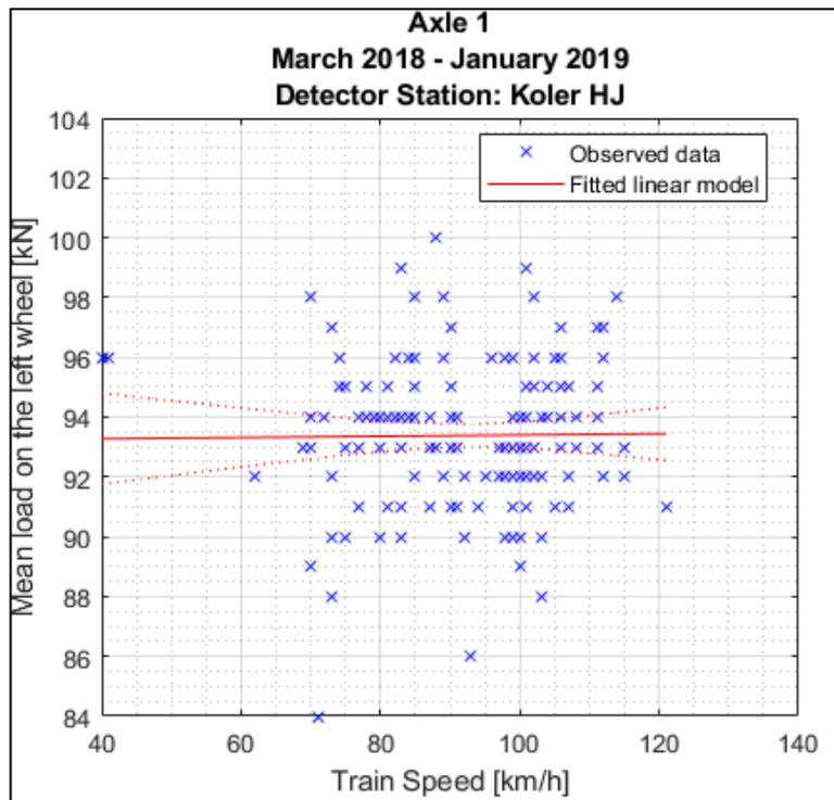
Figure B1.17: Simple linear regression model between train speed and mean wheel loads detected for the **left** wheel of the first axle of locomotive **917400014234** between March 18<sup>th</sup> 2018 and January 29<sup>th</sup> 2019 at **Koler** detector station.
