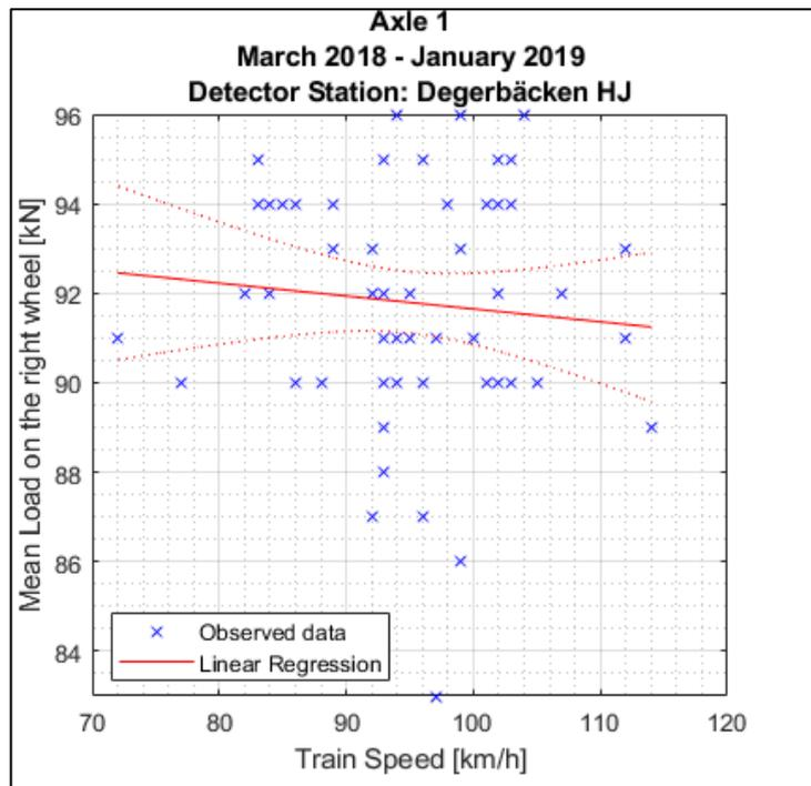
Figure B1.37: Simple linear regression model between train speed and mean wheel loads detected for the **right** wheel of the first axle of locomotive **917400014235** between March 18<sup>th</sup> 2018 and January 29<sup>th</sup> 2019 at **Degerbäcken** detector station.
